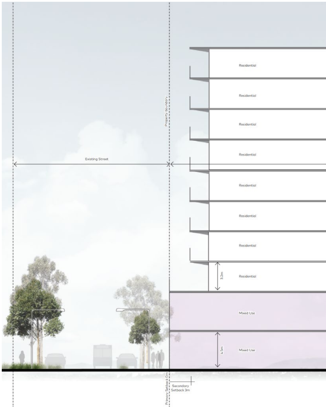
Figure 16: Example section for a mixed-use building
