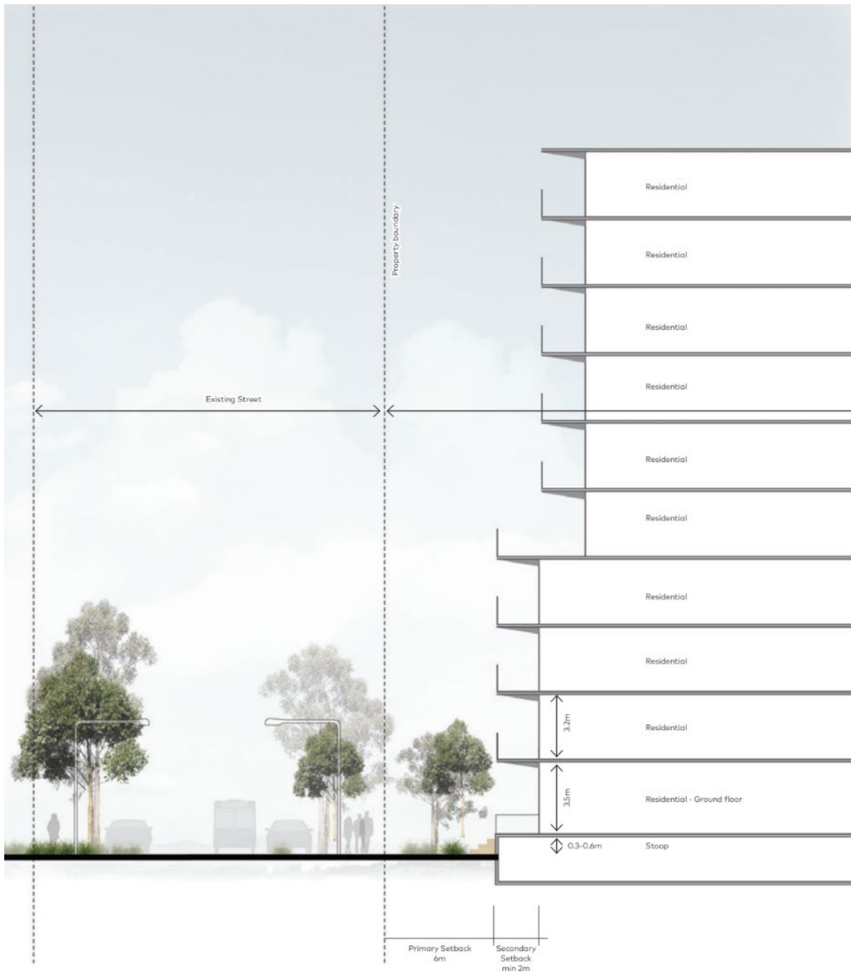
Figure 17: Example section for a high-density residential building
