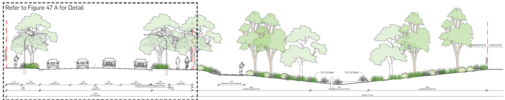
Figure 47 Typical Street Section - Riparian Collector Street
