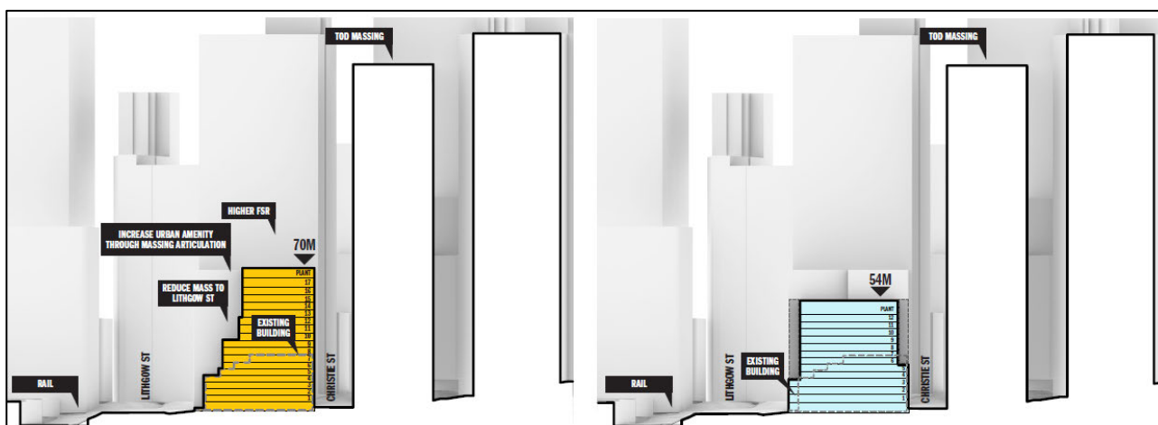
Figure 3 – Comparative Section Analysis – East-West: alternate building envelope (yellow) vs TOD changes (blue) Source: Hassell
