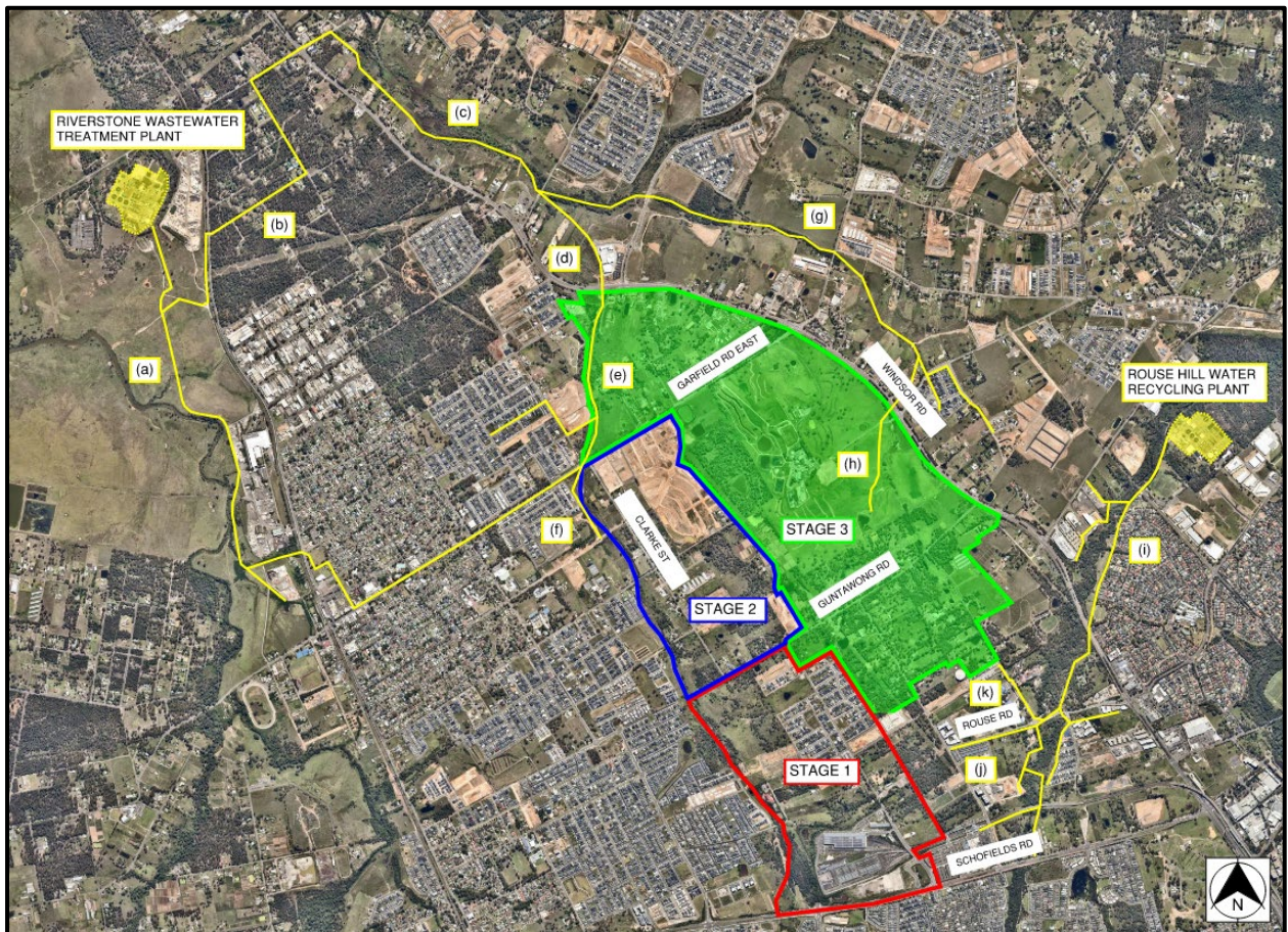
Figure 4 – Existing Wastewater Infrastructure
