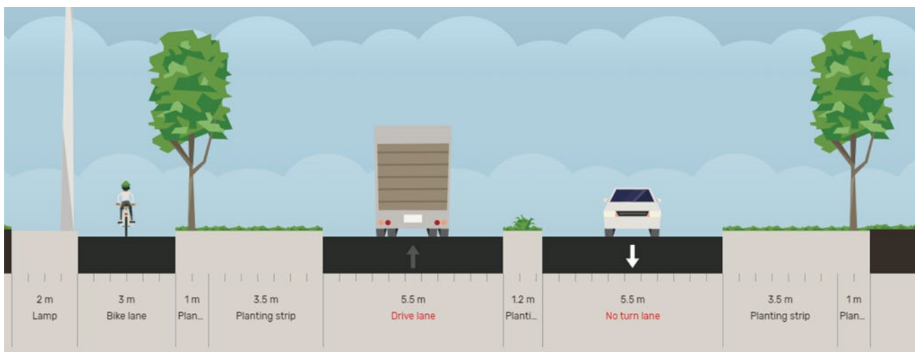
Figure 6.10 Southern Connector Road indicative cross-section
