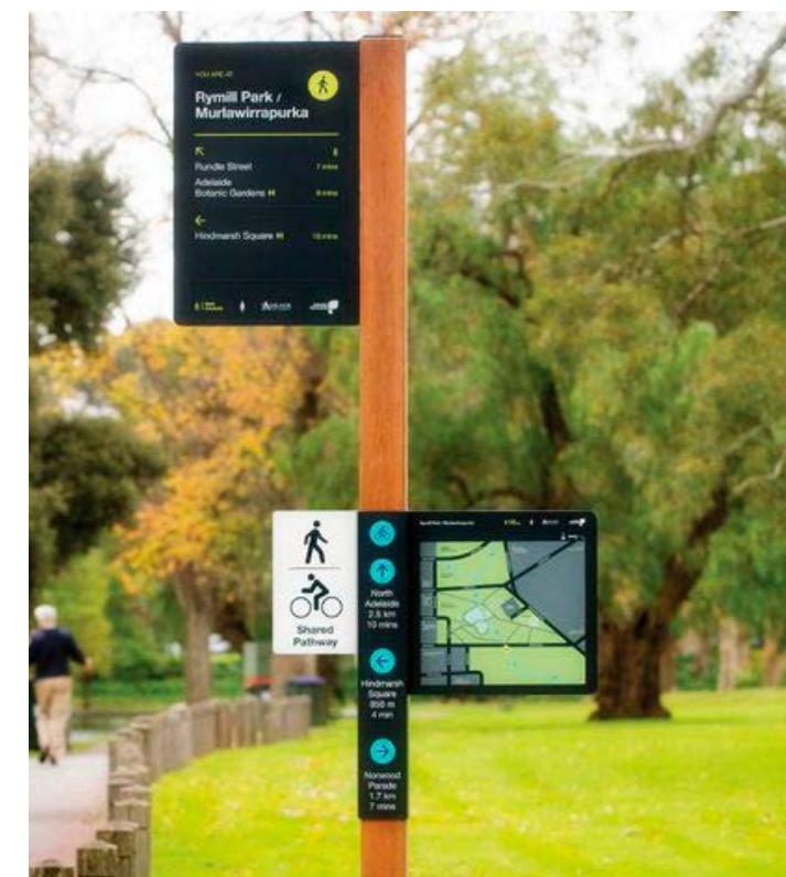
Extensive directional signage, timber and mild steel with printed graphics.
