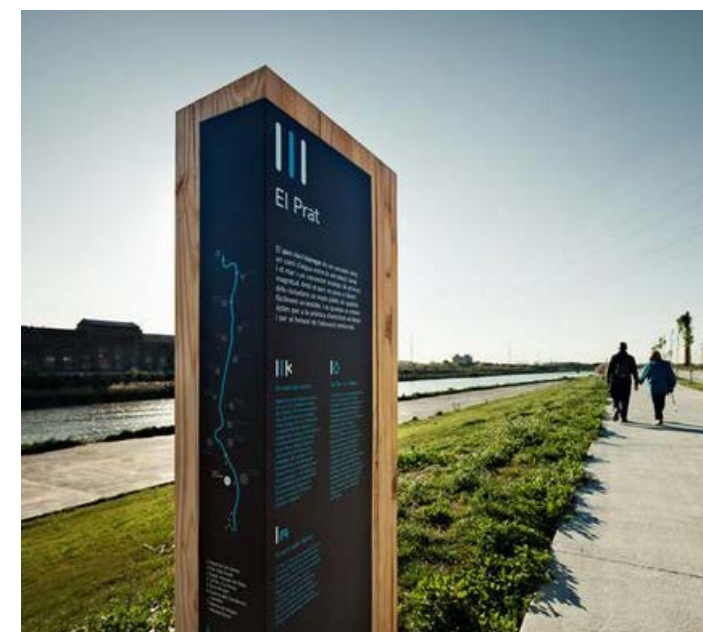
Pedestrian level informative signage, timber block and mild steel with printed graphics.
