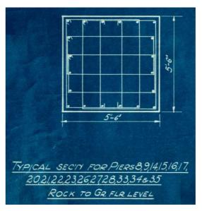
Figure 4 Original Structural drawing for Pier under a Typical column, founded down to rock.
