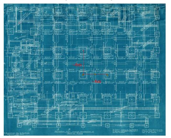
Figure 3 Ground Floor Column Layout Plan
