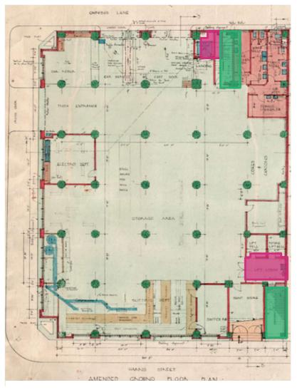
Figure 5 Original Ground Floor plan showing location of lift wells (pink) and stair cores (green).
