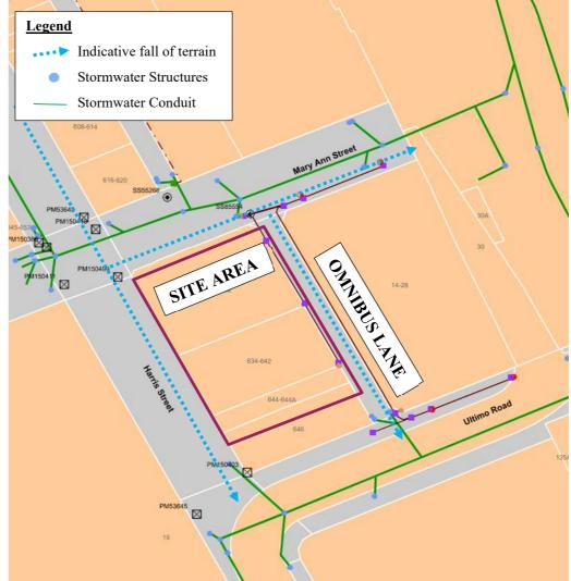
Figure 9 City of Sydney DBYD Plans (Please note: the brown lines, purple squares and pink circles represent electrical underground conduits, electrical pits and smart poles which are not relevant to this flooding assessment)
