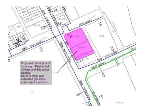
The current site is connected to 75NY medium pressure gas main 210kPa. Review of the capacity against future demand will be required to inform any system upgrades. Based on our initial review the existing gas meter would need to be upgraded to cater for the future loads. Application to Jemena would need to be lodged to verify the future demand during design stage.
