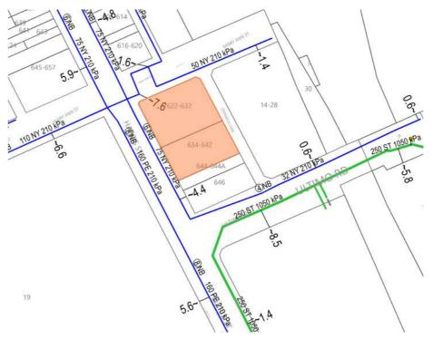
The existing gas meter is located on level 1 Harris Street, next to main Switch room. The current site is connected to 75NY medium pressure gas main 210kPa. Review of the capacity against future demand will require the gas meter upgrade and relocation to meet new building layout. The existing gas meter would need to be upgraded to cater for the future loads.
