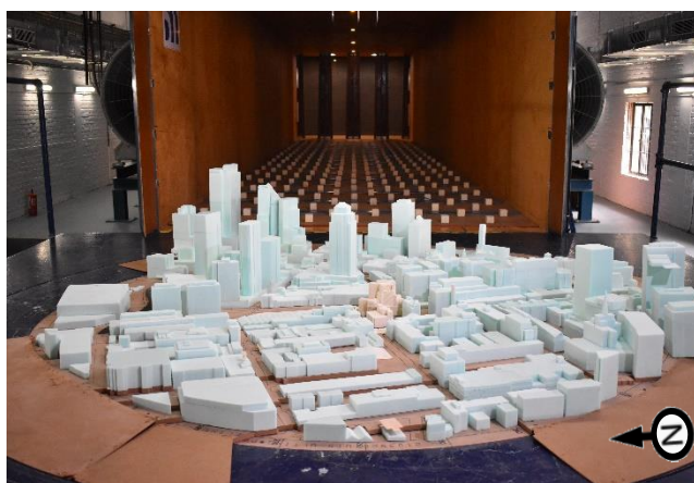
Image 2A: Wind Tunnel Study Model – Existing Configuration
