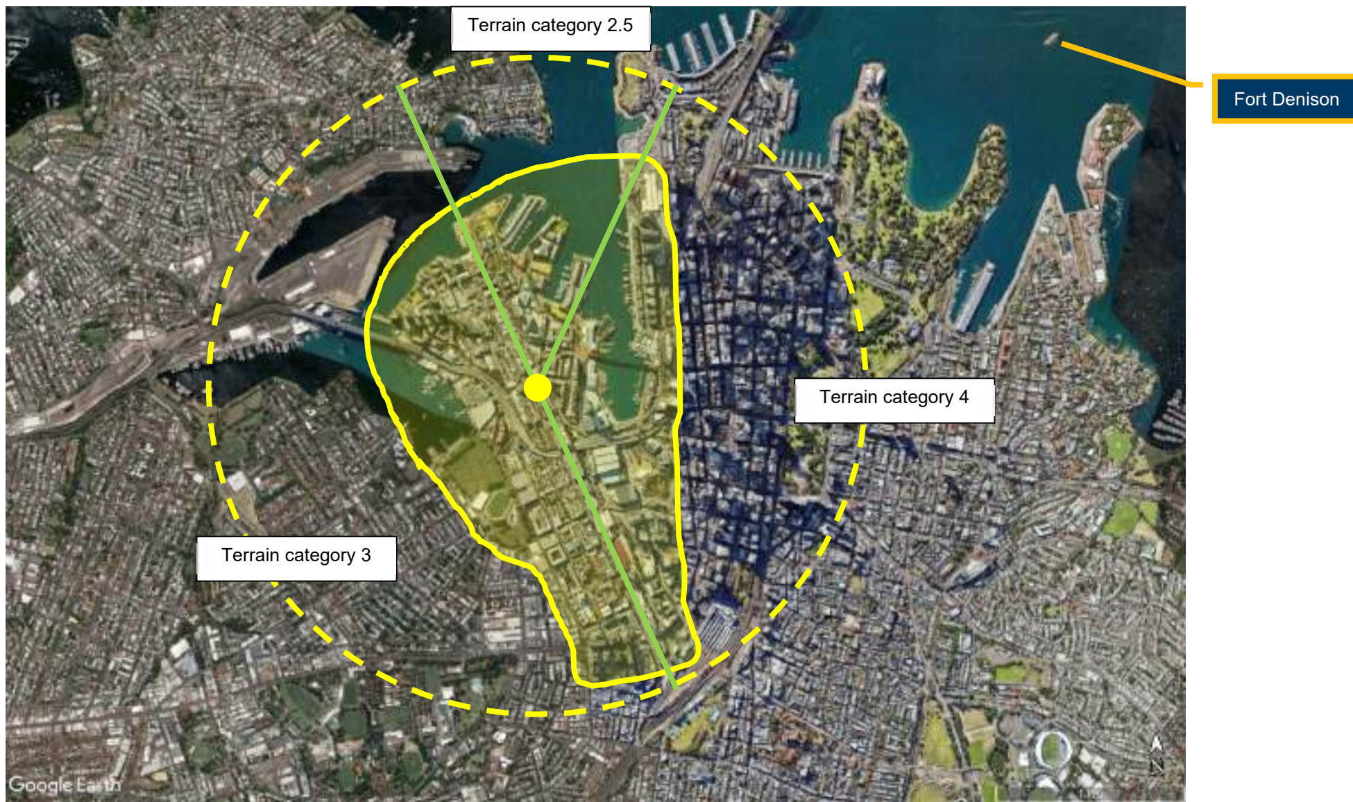
Figure 2 Aerial image of Pyrmont-Ultimo Development Region and Sydney CBD. Buildings modelled in highlighted region. Applied terrain categorisation as per AS1170.2
