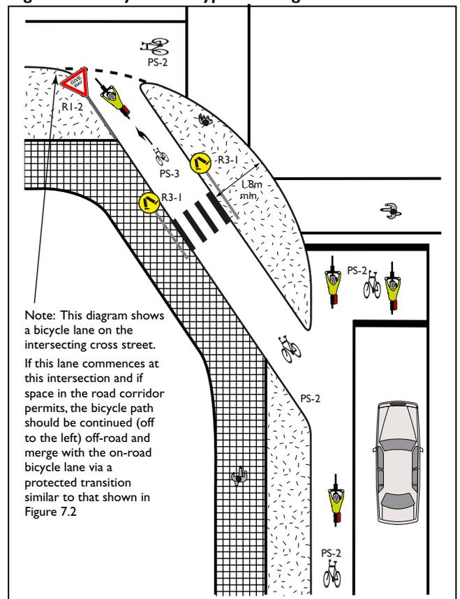
7.20 shows a left-turn bypass for riders at a signalised intersection. The concept behind this treatment is similar to Figure 5-21 in *Austrroads – Part 14*.
