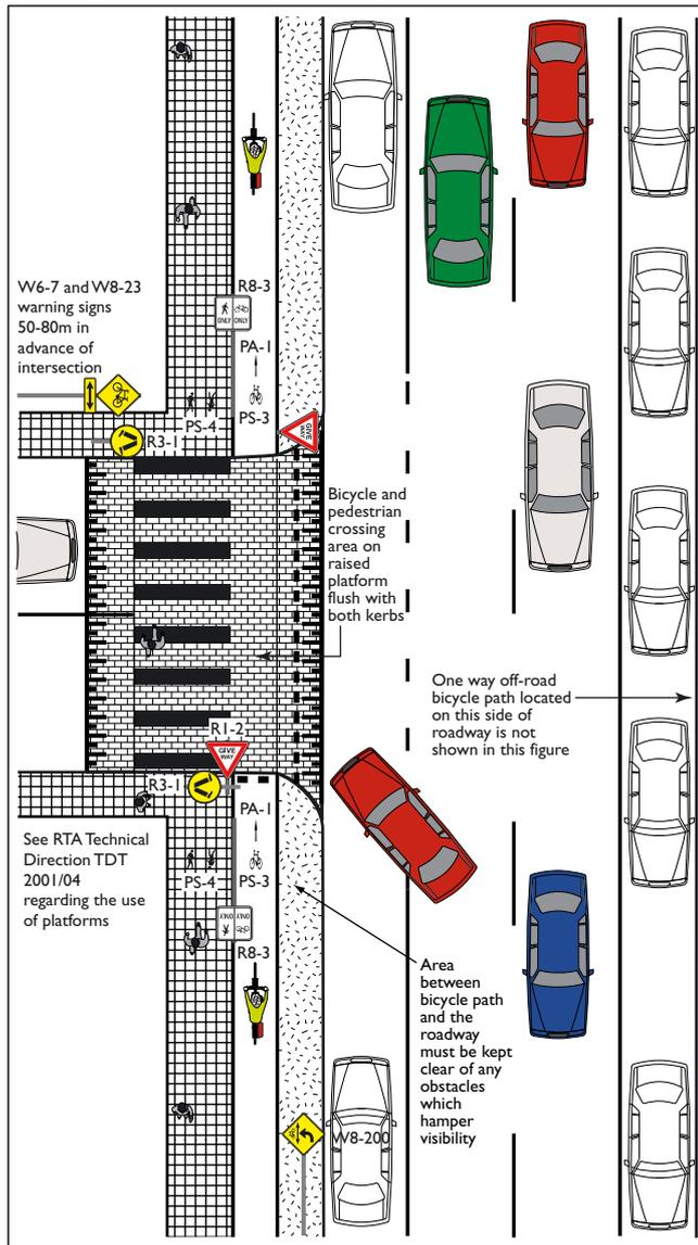
**Figure 7.5: Two-way off-road bicycle path intersection crossing on platform (not bent).**
