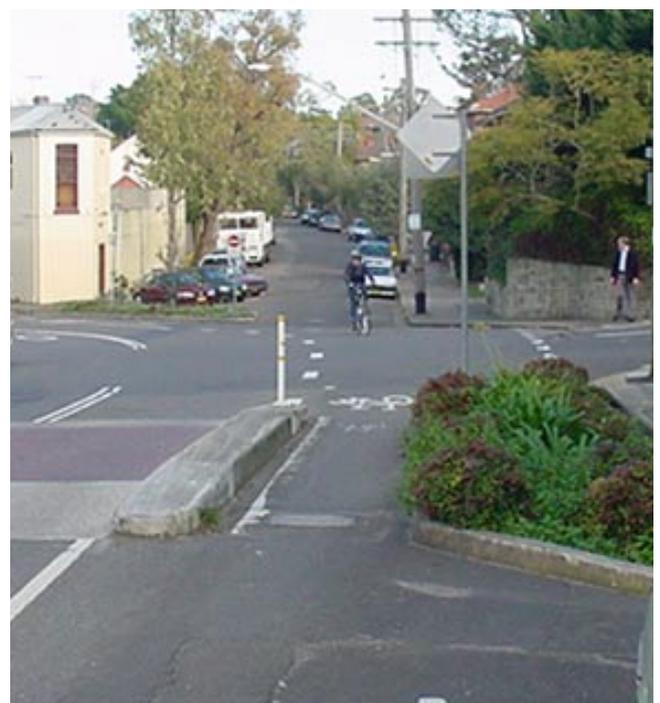
**Figure 5.14: Off-road two-way bicycle path to on-road bicycle lanes transition (with central refuge).**
