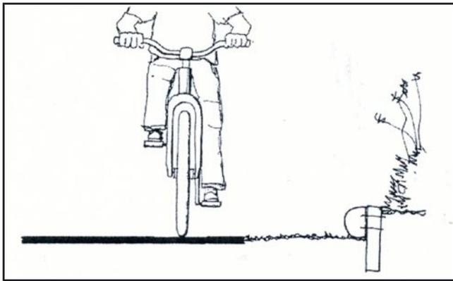
**Figure 8.5:** Clearances should be maintained on path edges to provide a safe and level run-off area.
