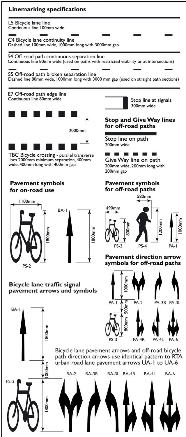
linemarking for dual-direction off-road paths is a dashed S5 centre line on straight sections becoming a S4 solid line on curves, steep gradients or where visibility is restricted.
