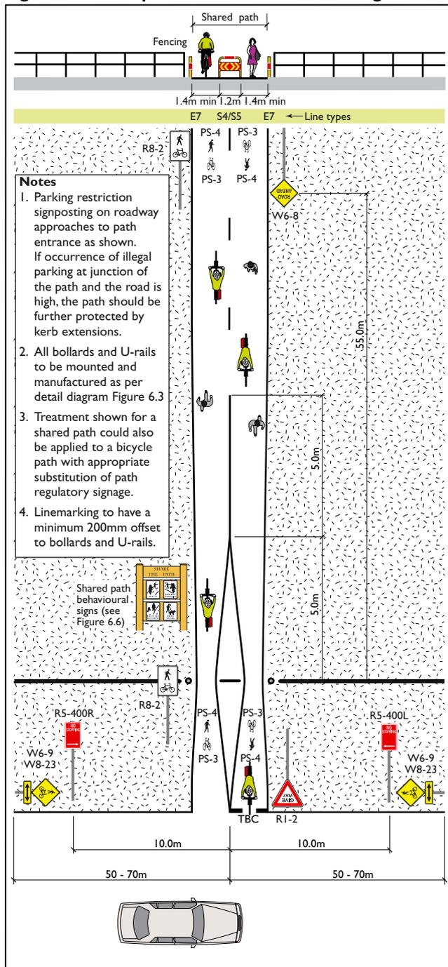
**Figure 6.5: Narrow path terminal treatment using bollards.**
