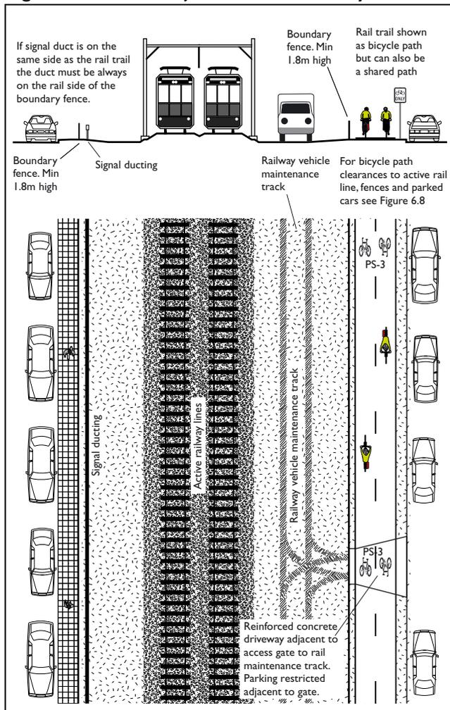
**Figure 6.8: Minimum clearance dimensions for rail trails.**
