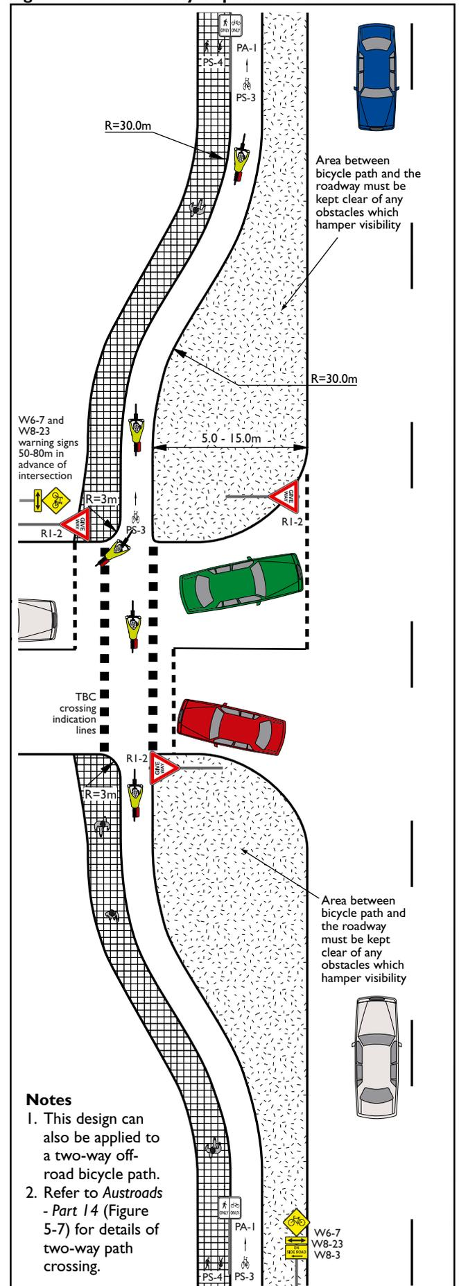
**Figure 7.4: One-way off-road bicycle path intersection crossing on platform (not bent).**
