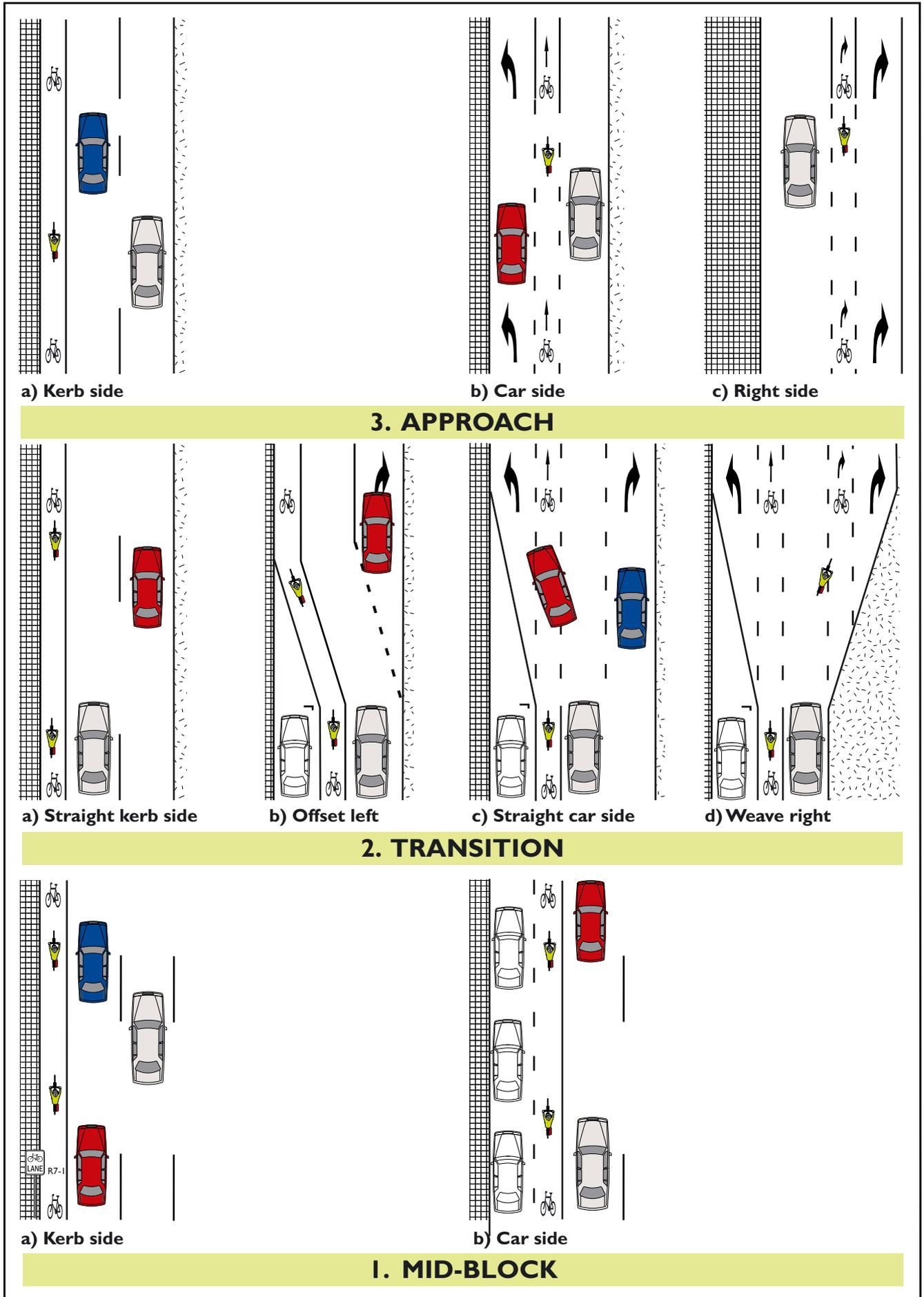
Figure 7.15b: Design options for signalised intersections.
