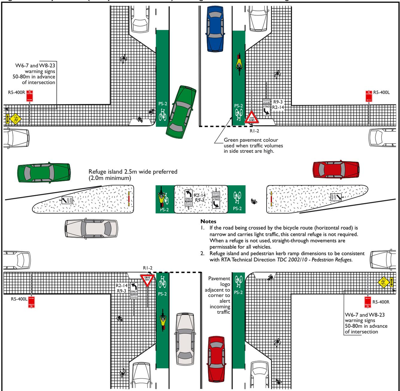
**Photo 7.2: Example of through lanes linking bicycle shoulder lanes at an unsignalled intersection on a rural type road with a left-turn lane. Blacktown Rd, Richmond.**
