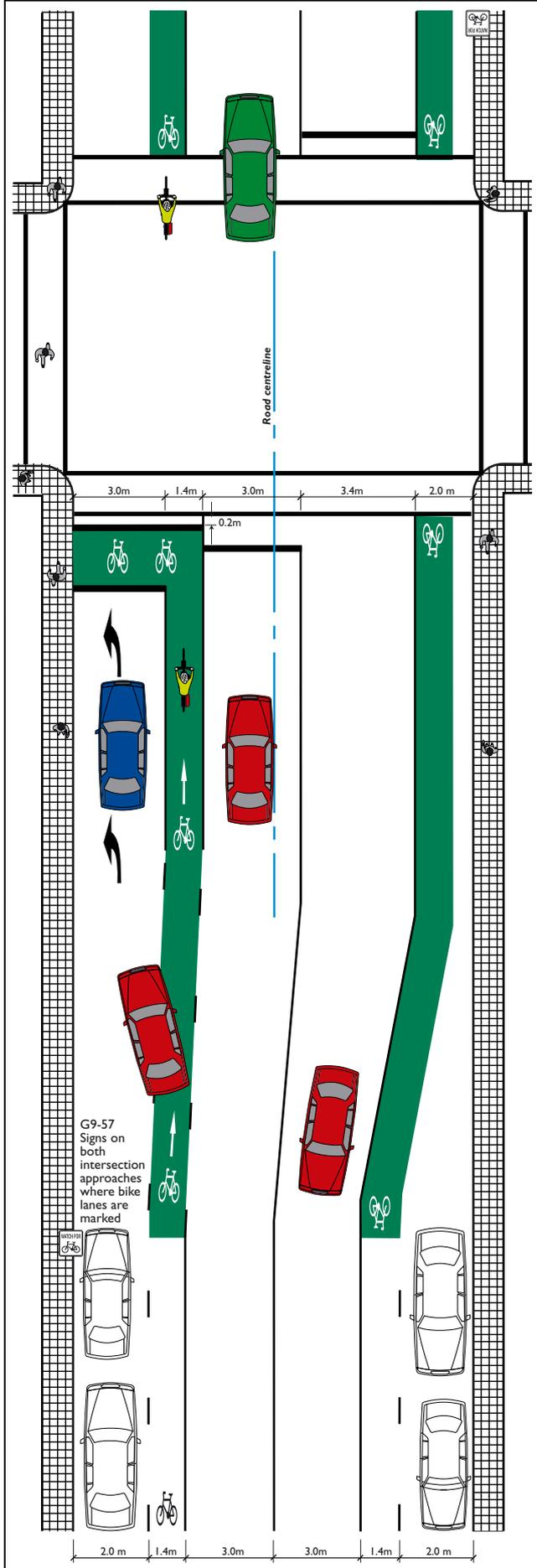
**Figure 7.17: Bicycle shoulder lanes through a signalised intersection located kerbside on approach and departure.**
