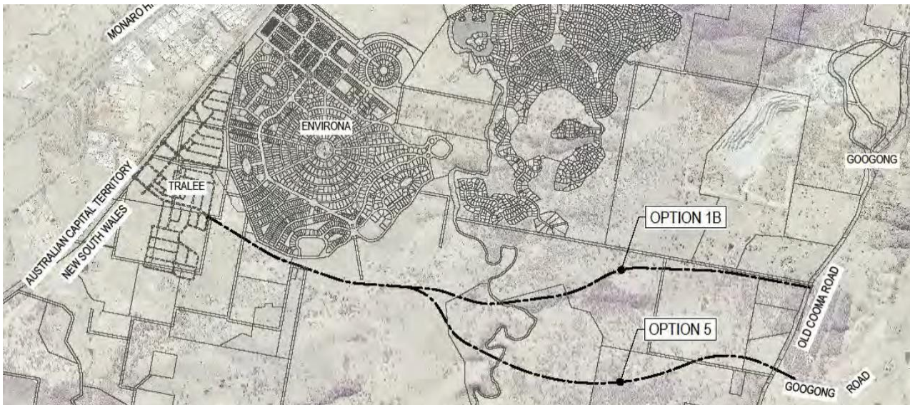
Figure 5–7 | Dunns Creek Road alignment options (QPRC, 2015)
