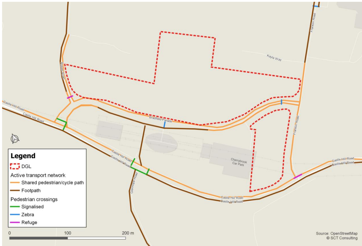
Figure 3–6 Existing footpath and pedestrian crossing facilities in proximity of the site
