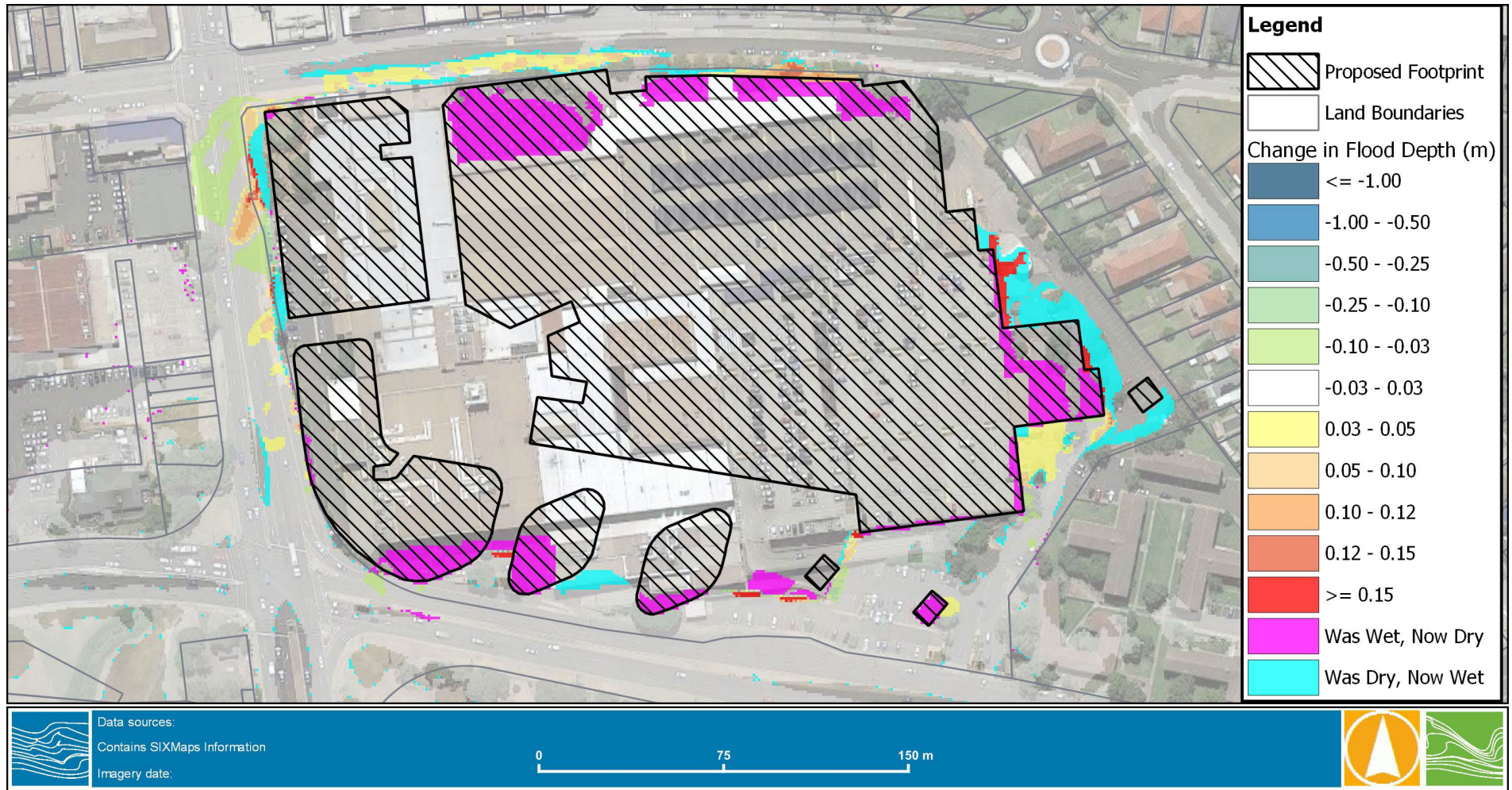
Figure 16: Afflux in 1% AEP overland flood based on the reference design (Water Technology, 2023)
