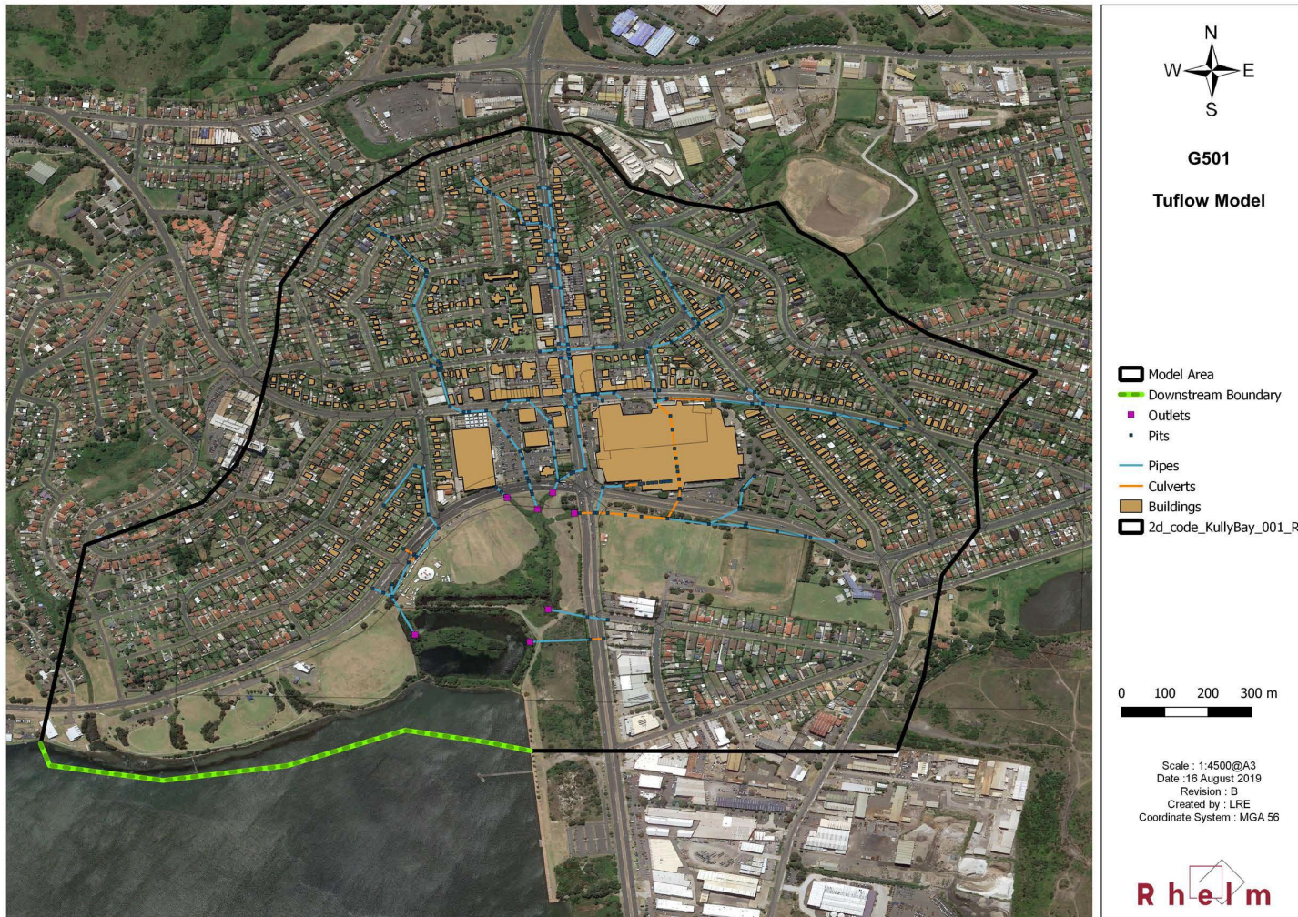
Figure 22: Drainage network incorporated into TUFLOW model for the Kelly Bay overland Flow Study (Rhelm, 2019)
