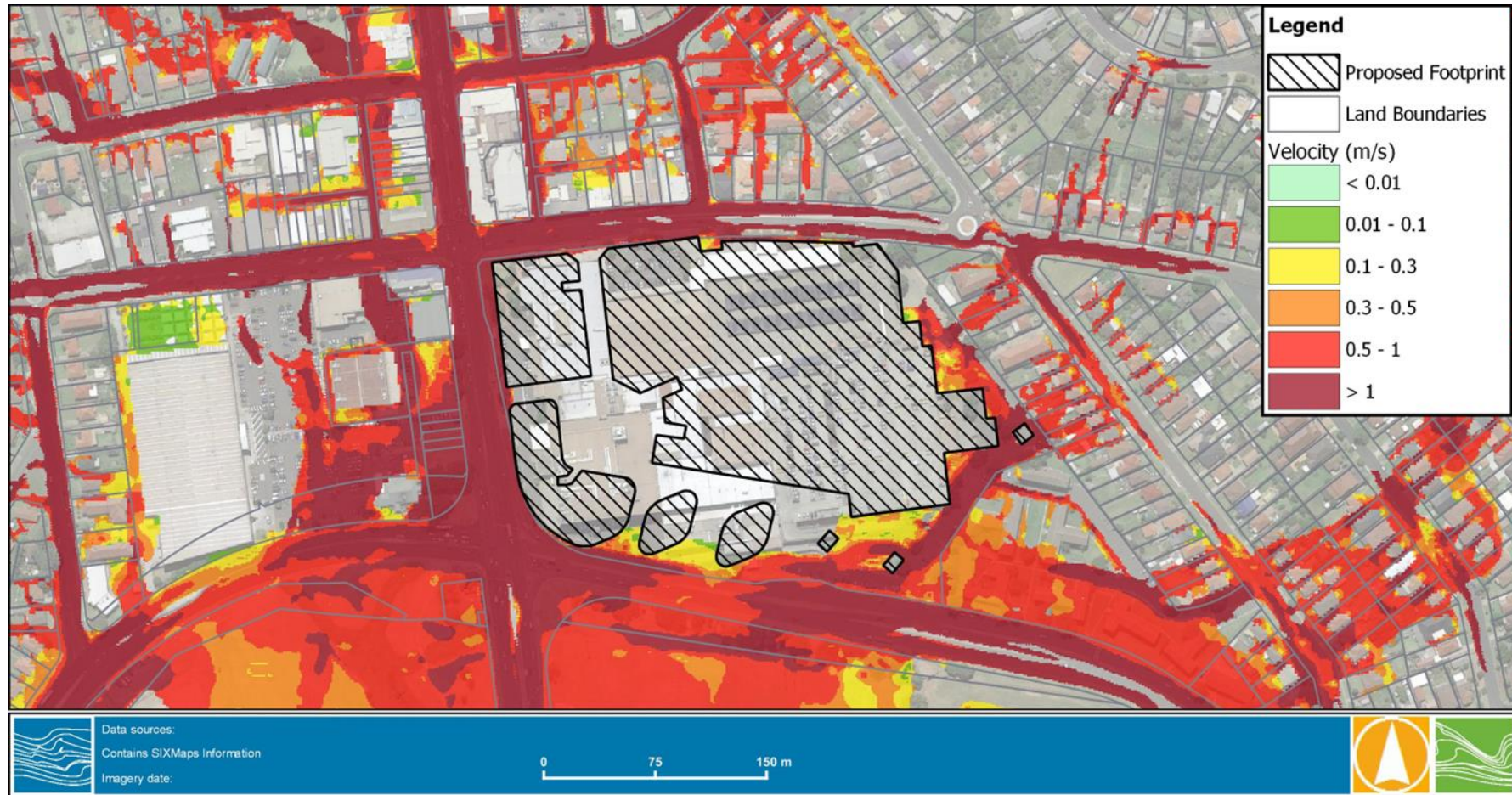
FIGURE 3-11 PMF PEAK VELOCITY - REFERENCE DESIGN
