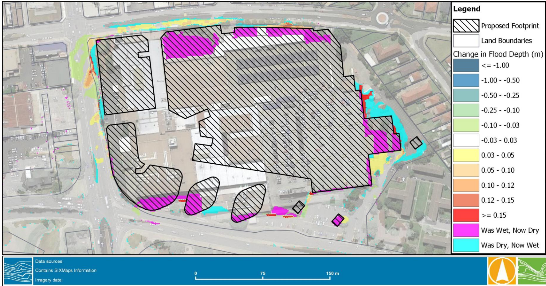
FIGURE 3-8 1% AEP FLOOD DEPTH DIFFERENCE REFERENCE DESIGN VS EXISTING (SITE SPECIFIC)
