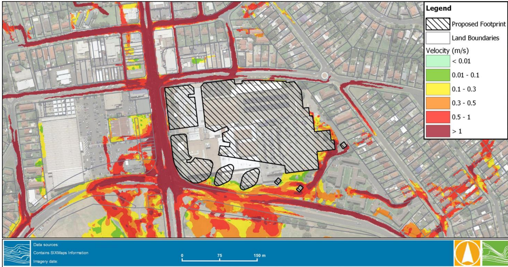
FIGURE 3-6 1% AEP PEAK VELOCITY - REFERENCE DESIGN
