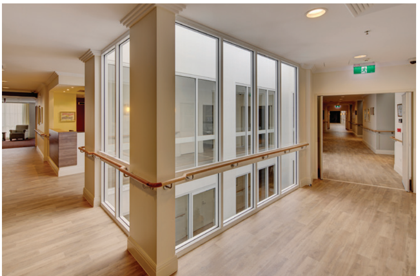
Fig 1.4.A Lightwells bring daylight and variance in light quality through the day into deep parts of the building
