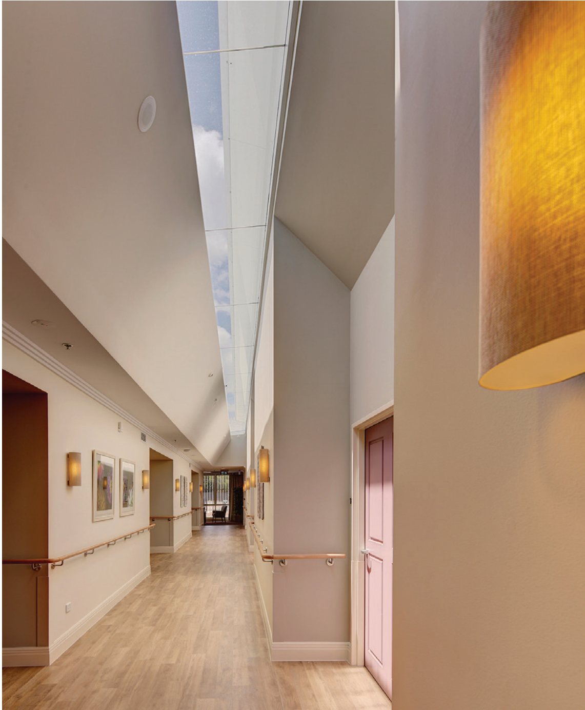
Fig 4.4.A Residential care facility with skylit corridor to vary quality of light inside, provide glimpses of the sky and maximise access to daylight
