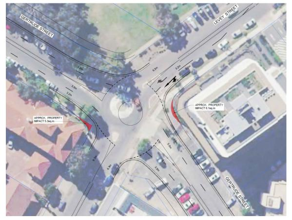
Figure 43 Roundabout intersection layout – Gertrude Street / Levey Street
