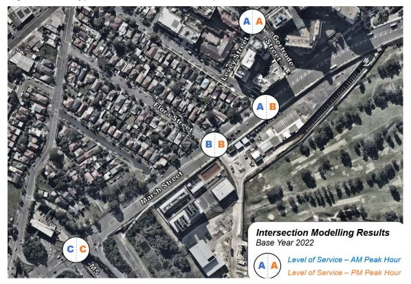
Figure 14 Existing intersection level of service
