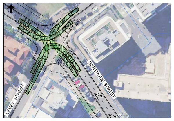
Figure 21 Intersection design – Gertrude Street / Levey Street Source: Arup
