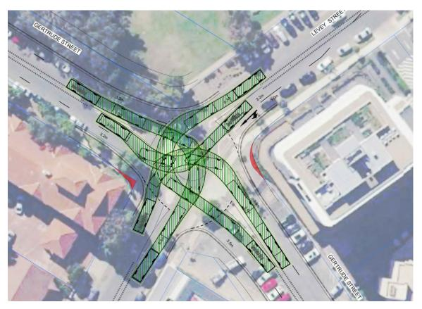
Figure 44 Vehicle swept paths – Gertrude Street / Levey Street (roundabout control)
