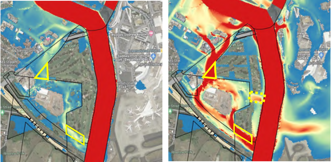
Figure 12: Option 2 case flood intensities (VxD) for 1% AEP flood (left) and PMF (right)
