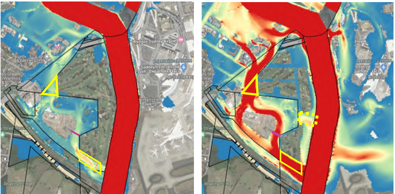
Figure 16: Option 4 case flood intensities (VxD) for 1% AEP flood (left) and PMF (right)
