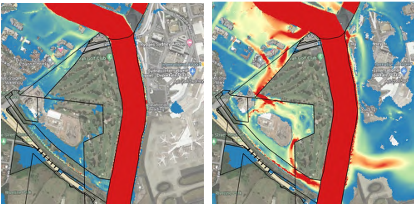
Figure 10: Option 1 case flood intensities (VxD) for 1% AEP flood (left) and PMF (right)
