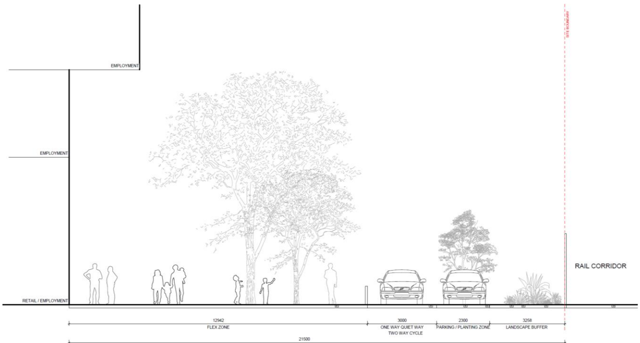
Figure 23: Section K – Pedestrian thoroughfare along rail interface
