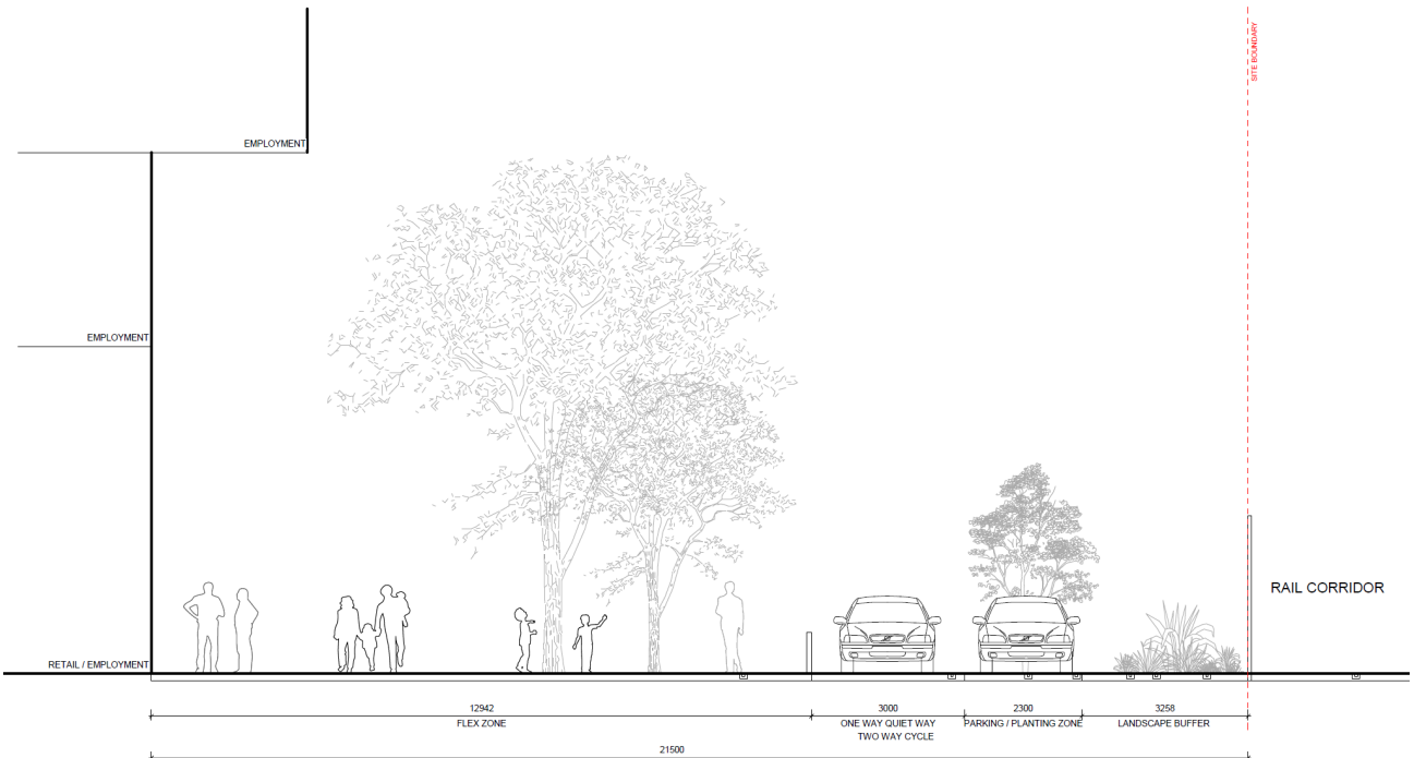
Figure 23: Section K – Pedestrian thoroughfare along rail interface
