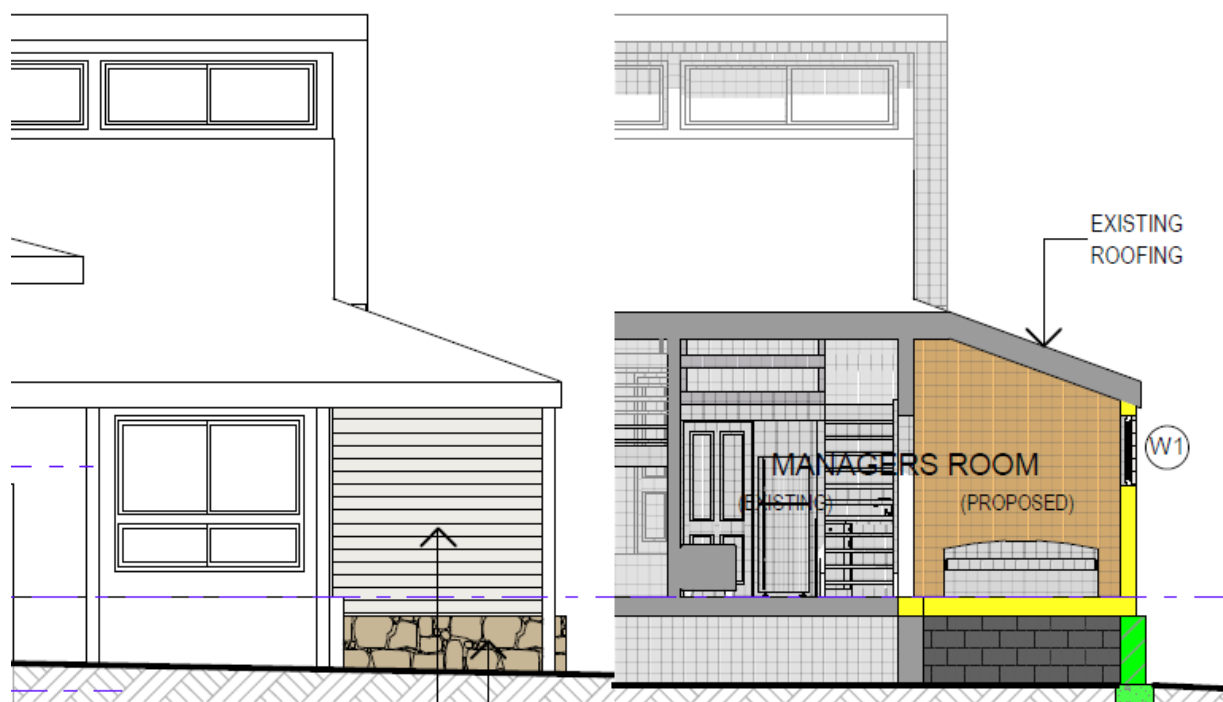
Figure 9 | Proposed managers room elevation and section plan (Source: Applicant's documentation)
