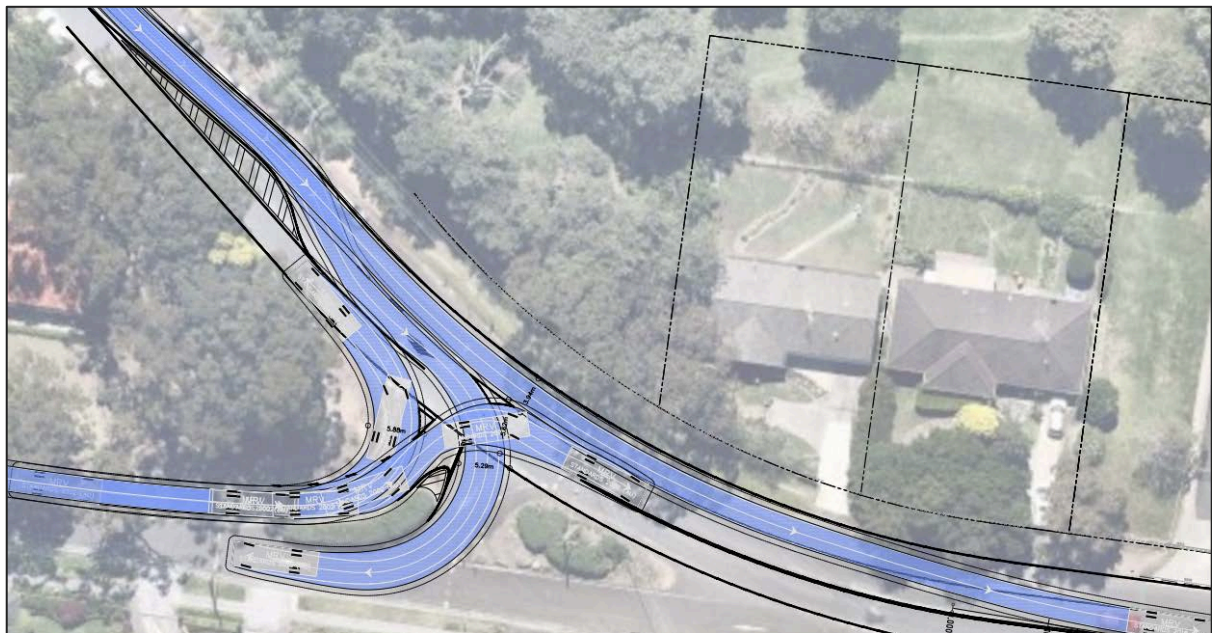
Figure 3 | Concept plan for seagull arrangement at intersection of Browns Road and The Comenarra Parkway (base image source: Amended Modification Applications, May 2022)
