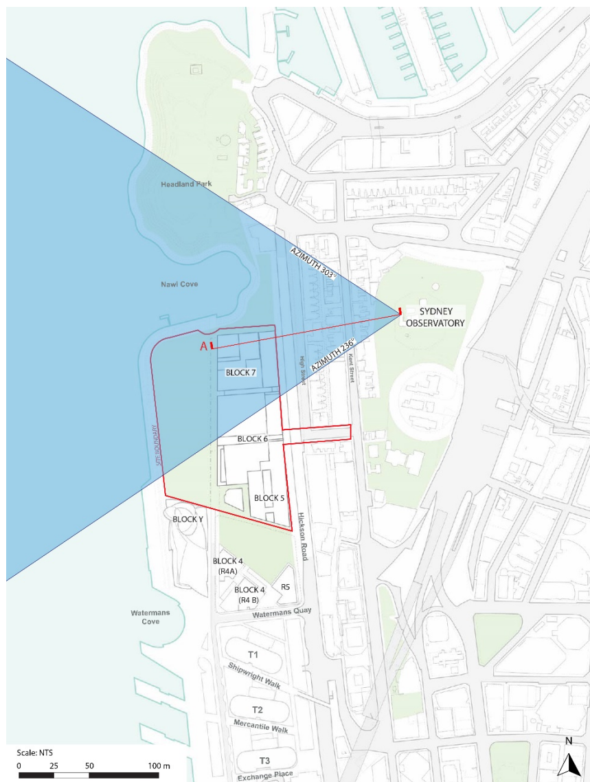
Figure 5. Azimuth clear zone range 236° to 303° in relation to the Barangaroo development. Source: amended by AECOM from figure prepared by Hassell, June 2021 .
