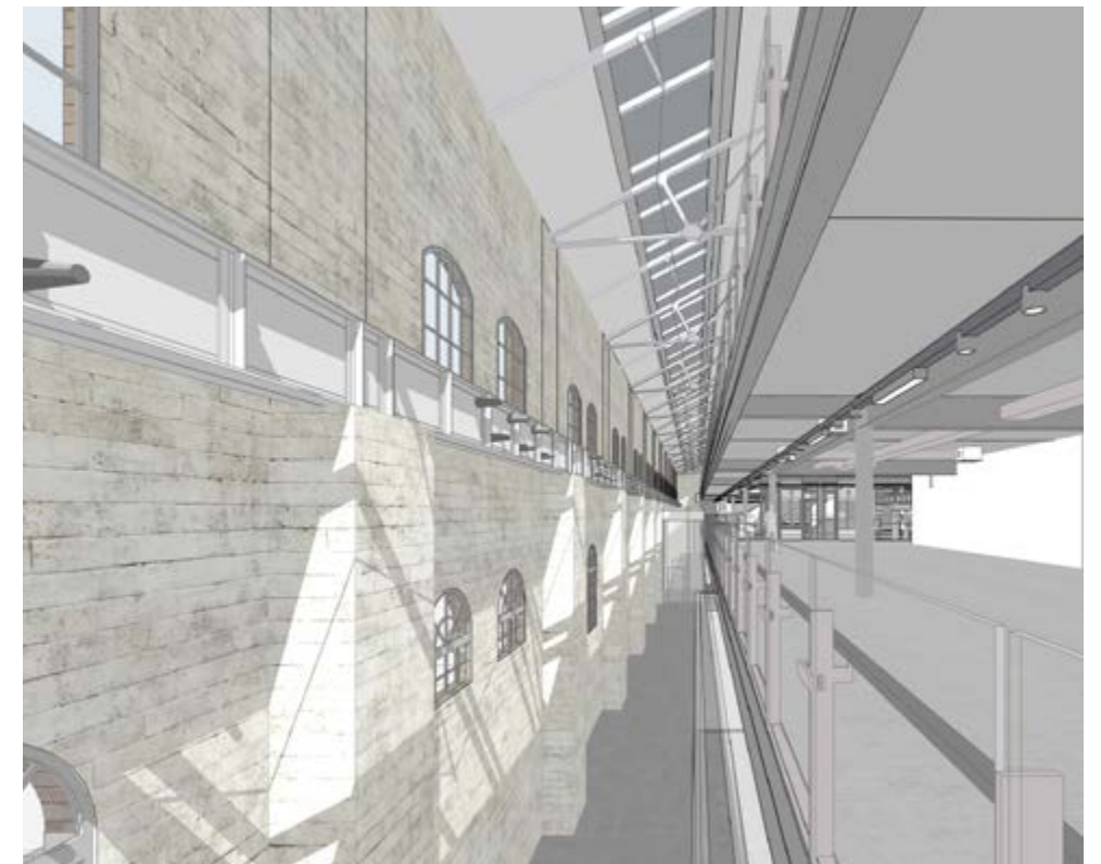
/ Southern void: offset between new and existing fabric (subject to detailed design and approvals)
