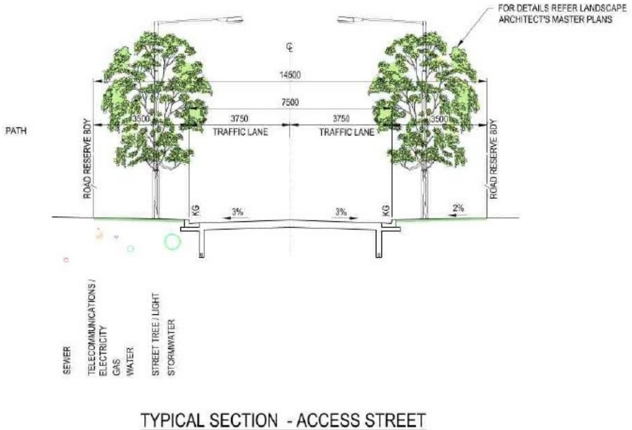
Figure 4.4 – Access Street Cross Section
