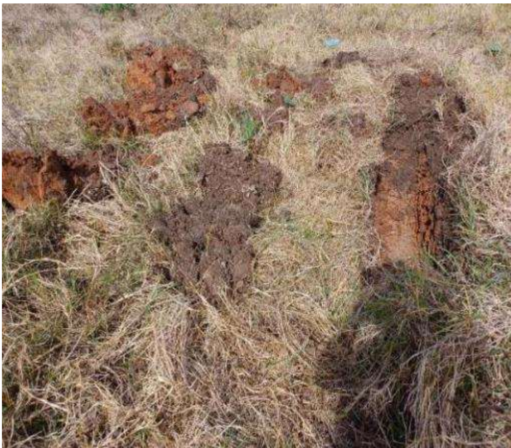
Image 10.1.2.1 View of topsoil (middle) and natural soils (left) encountered at TP61 (right)
