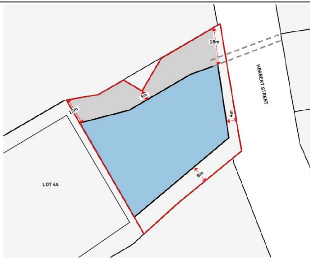
Figure 13: Podium envelop (source: Urbis)
