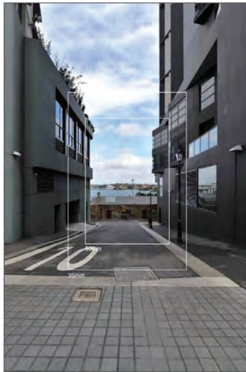
Original photo with crop marks to identify the field of view of longer lens sizes.
