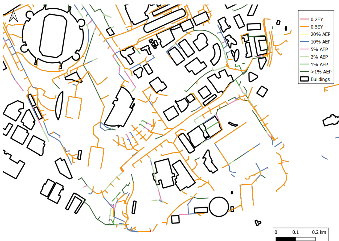
Figure 3.16: Constraints in pipe system capacity – Town Centre (south) and Parklands
