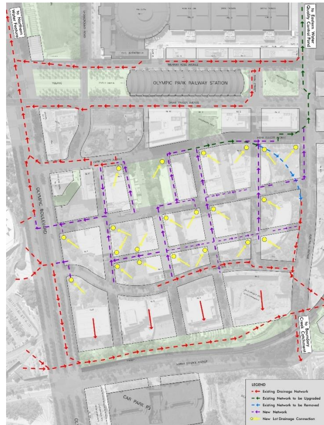
Figure 26. Drainage diversions in the Urban Centre Neighbourhood as proposed by SOPA
