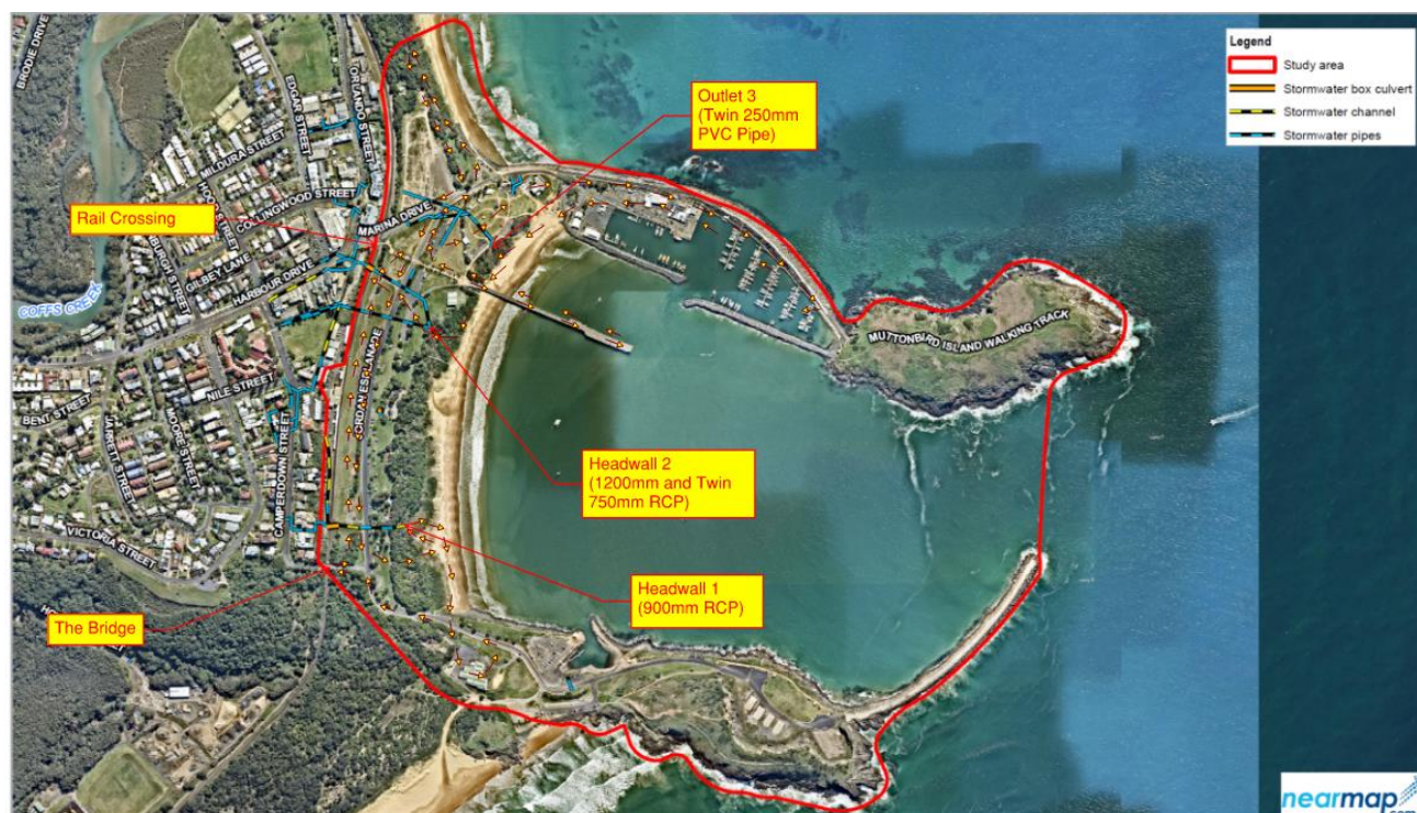
Figure 7 – Coffs Harbour City Council online map with existing stormwater infrastructure and key items inspected. (Source: Nearmap -True North)
