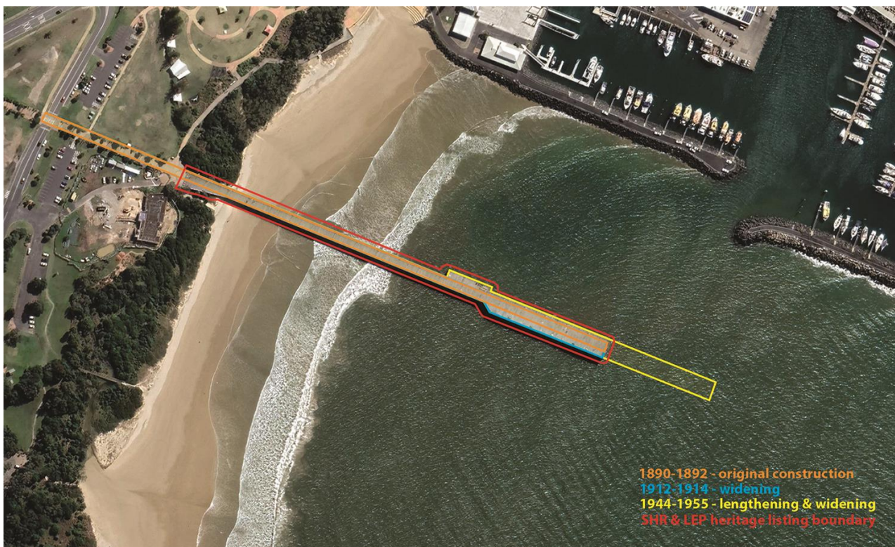
Figure 4.3: Footprint outlines of construction phases of Coffs Harbour jetty overlain on current aerial photograph – SHR and LEP heritage listing boundaries shown in red.
