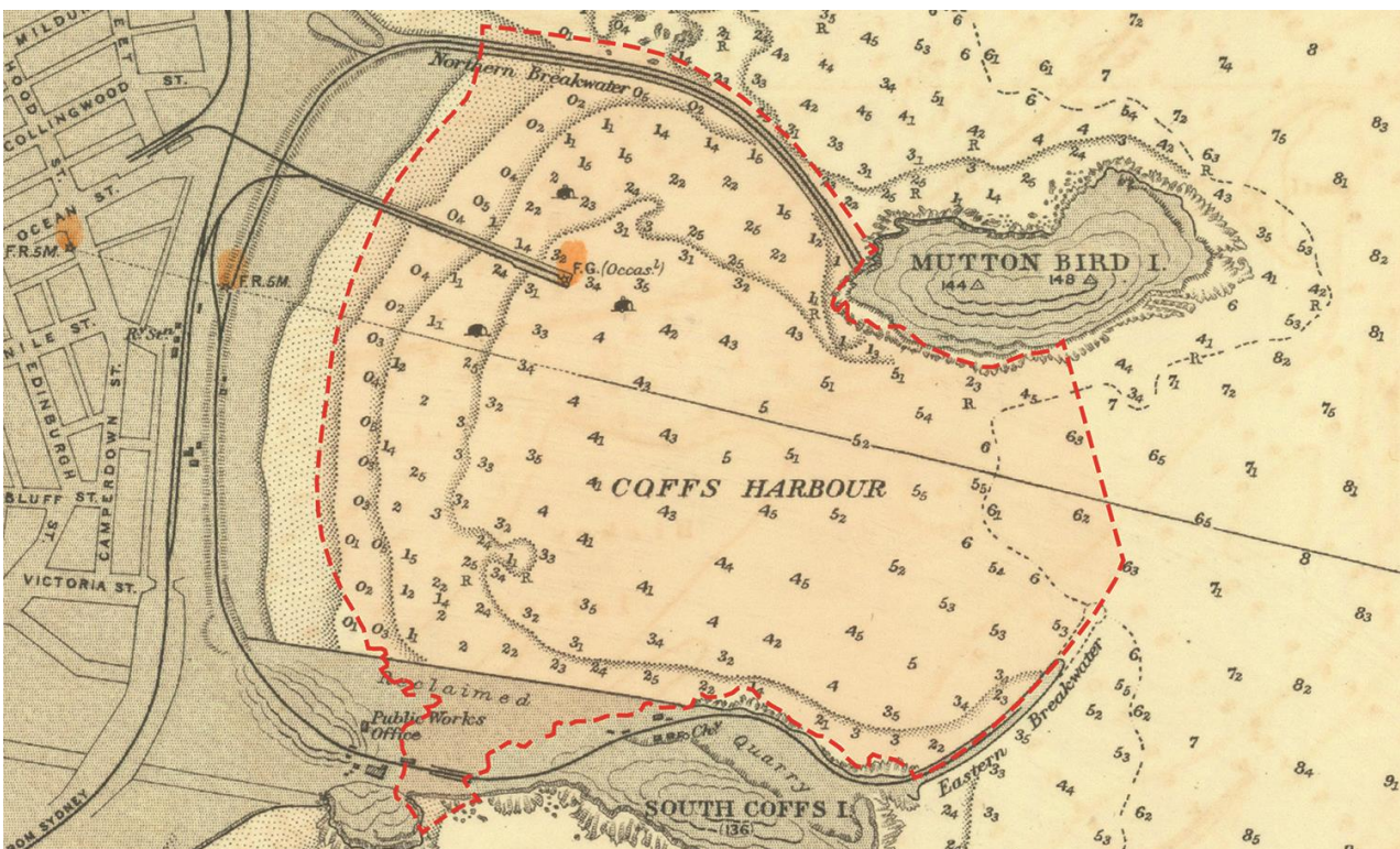
Figure 3.46: 1934 hydrographic chart of Coffs Harbour 82 – showing completed northern breakwater, partially completed eastern breakwater, quarry on South Coffs Island, and retaining wall and reclamation connecting South Coffs Island to the mainland; also expanded Coffs Harbour jetty and three mooring barrel buoys. Maritime archaeological assessment study area outlined in red.
