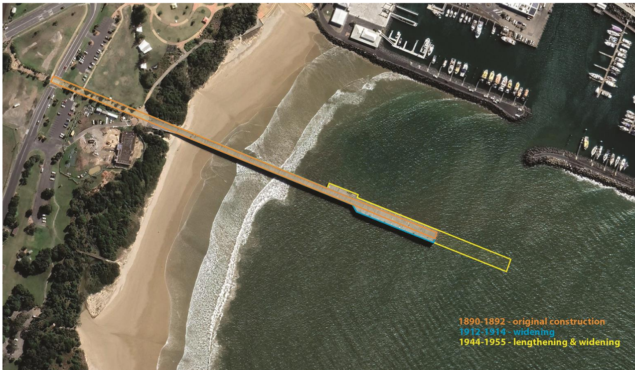
Figure 4.2: Footprint outlines of construction phases of Coffs Harbour jetty overlain on current aerial photograph.
