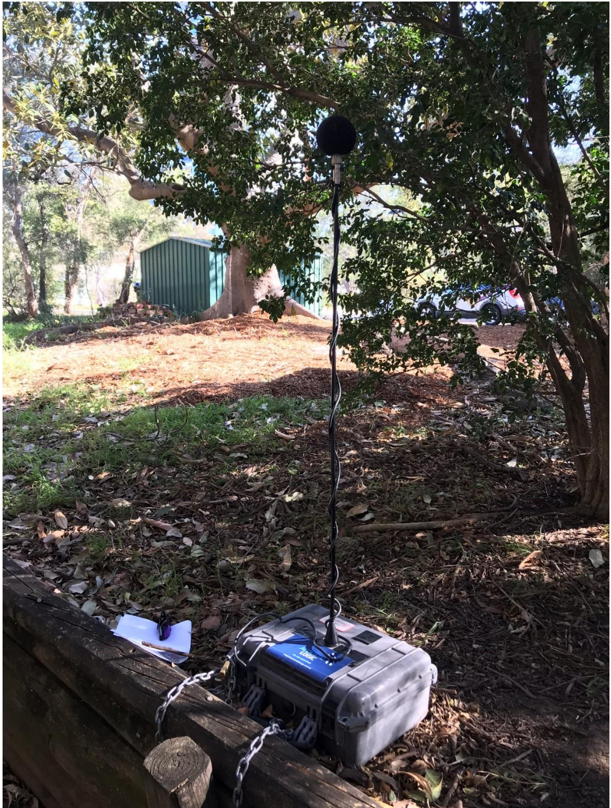
Figure C-1 – Unattended Noise Monitor Installation Photo.
