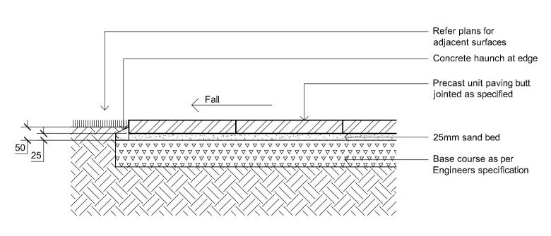
PRECAST UNIT PAVERS ON GRADE SCALE 1:10
