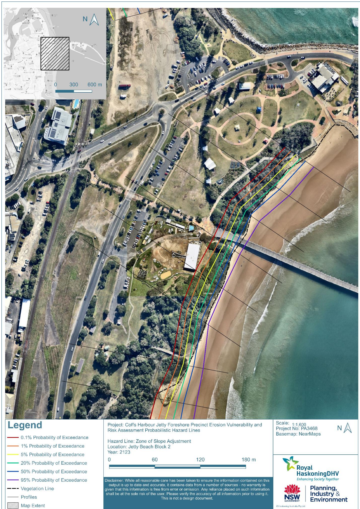
Figure B3-3: Zone of Slope Adjustment at Jetty Beach Block 2 (2123)
