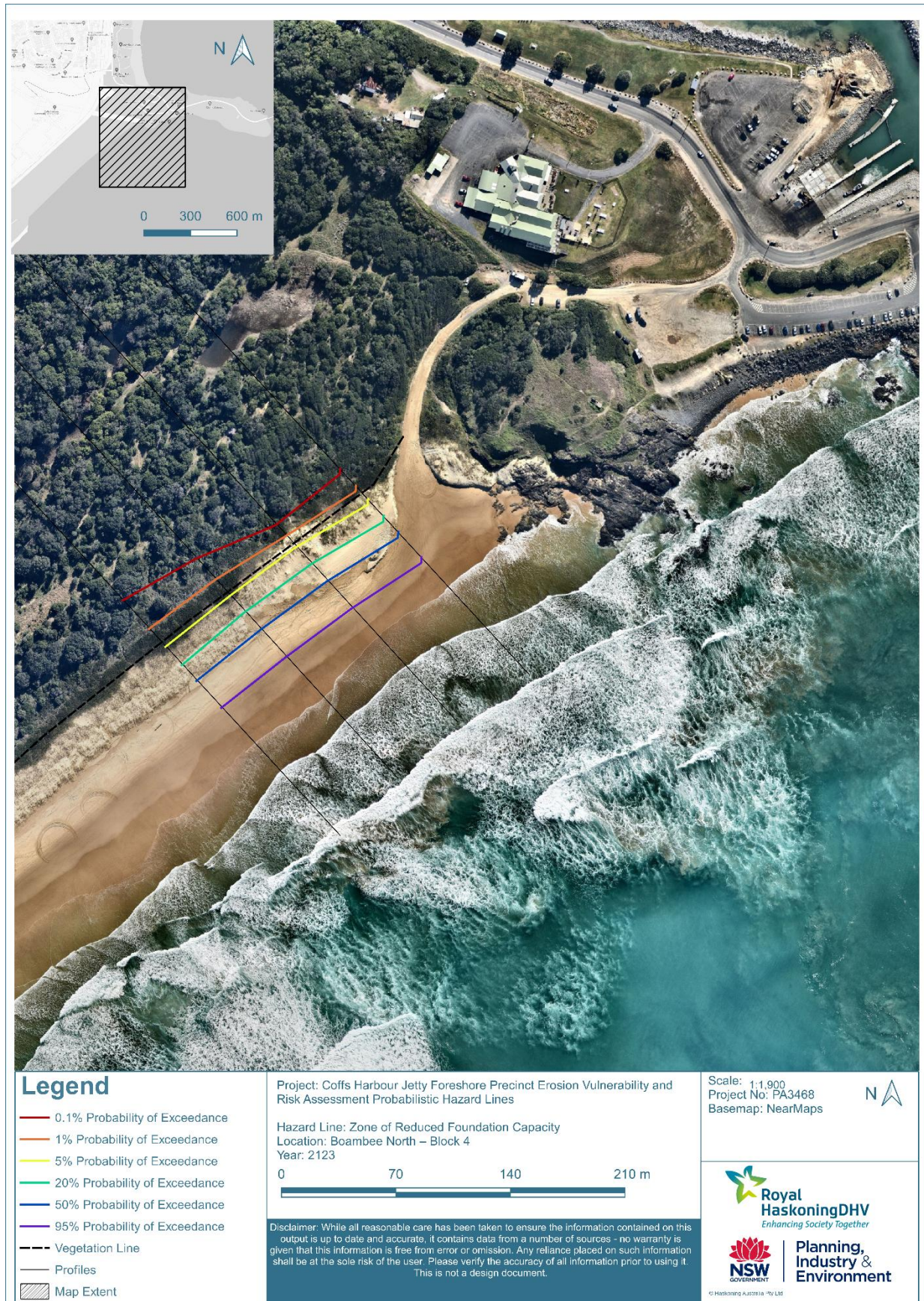
Figure B1-6: Zone of Reduced Foundation Capacity at Boambee North (2123)
