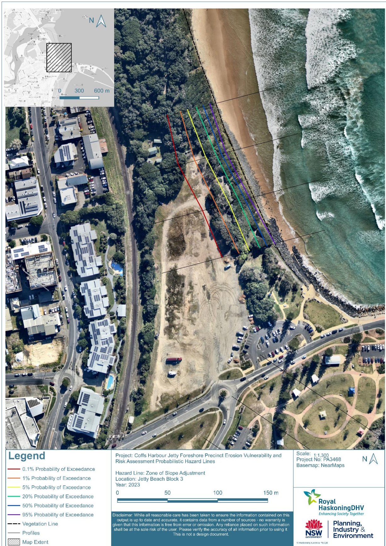
Figure B4-1: Zone of Slope Adjustment at Jetty Beach Block 3 (2023)
