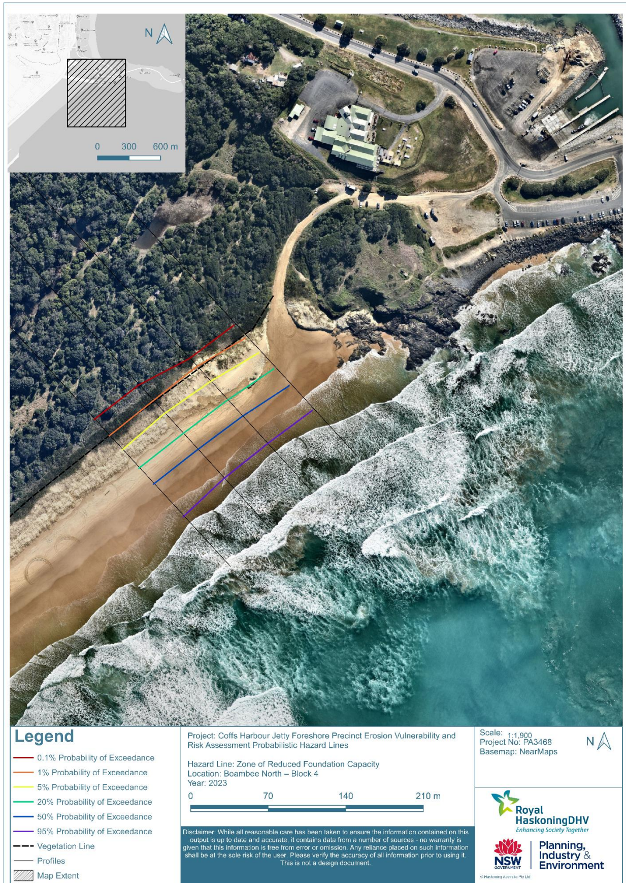
Figure B1-4: Zone of Reduced Foundation Capacity at Boambee North (2023)
