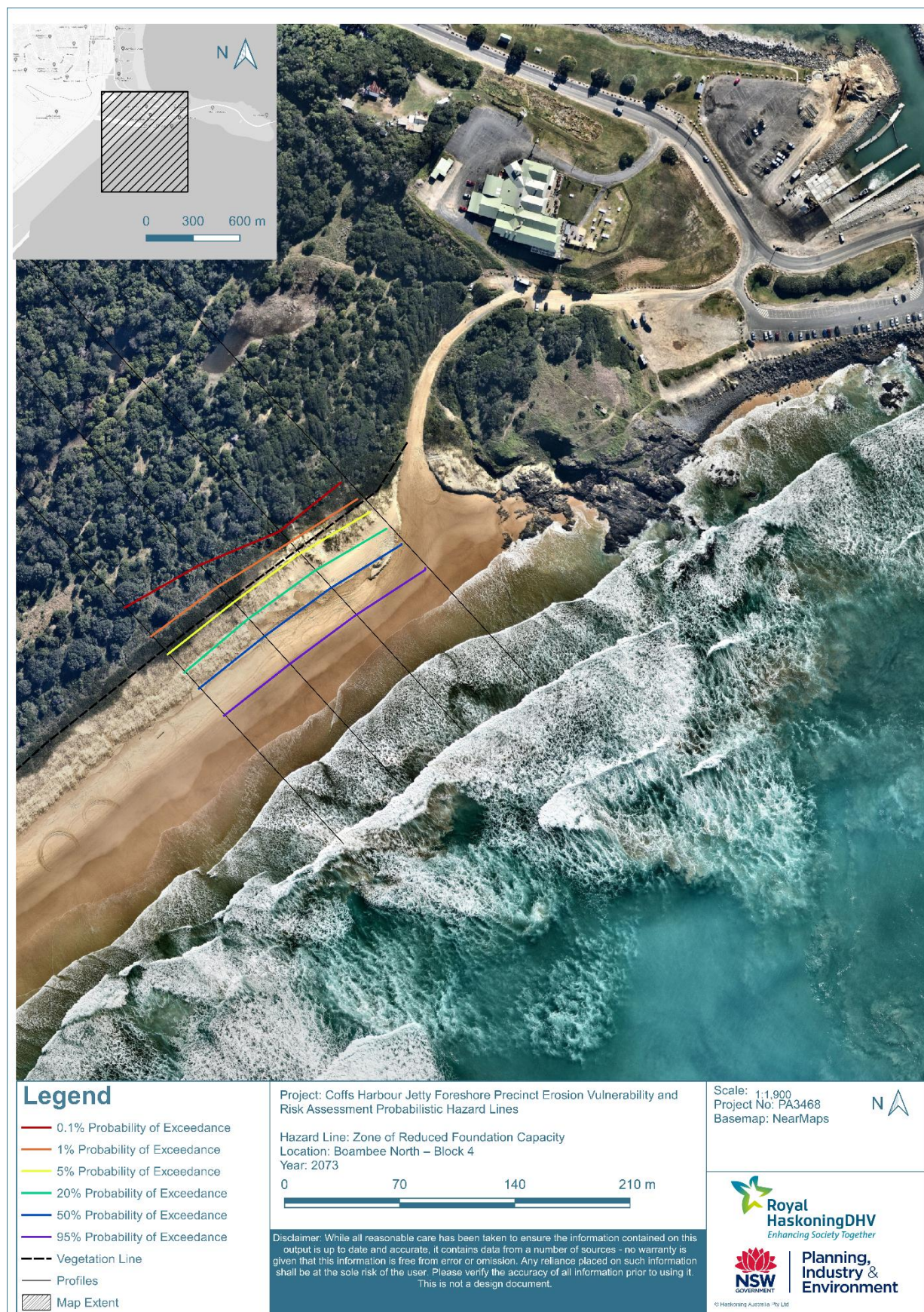
Figure B1-5: Zone of Reduced Foundation Capacity at Boambee North (2073)
