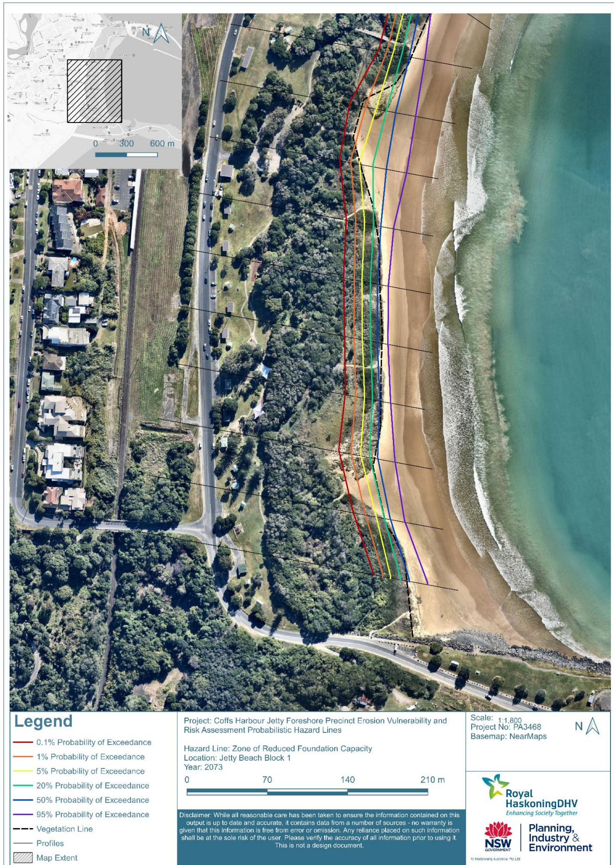
Figure B2-5: Zone of Reduced Foundation Capacity at Jetty Beach Block 1 (2073)
