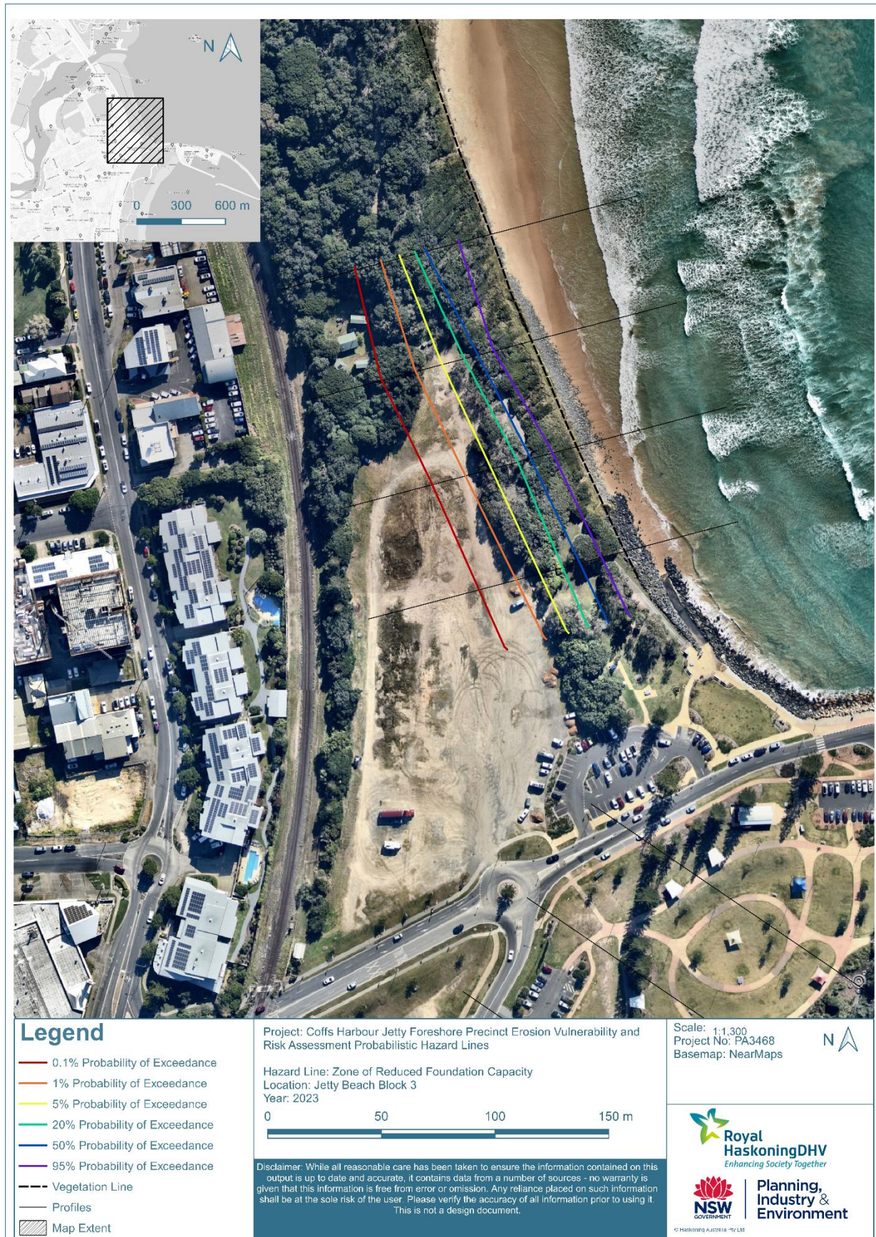
Figure B4-4: Zone of Reduced Foundation Capacity at Jetty Beach Block 3 (2023)
