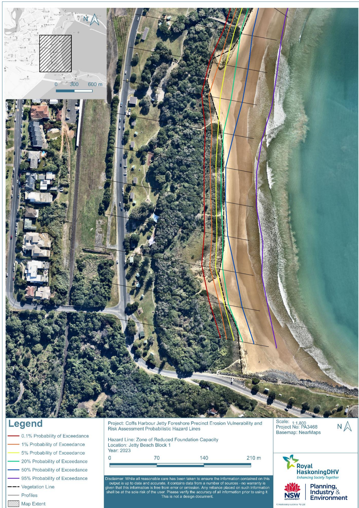
Figure B2-4: Zone of Reduced Foundation Capacity at Jetty Beach Block 1 (2023)
