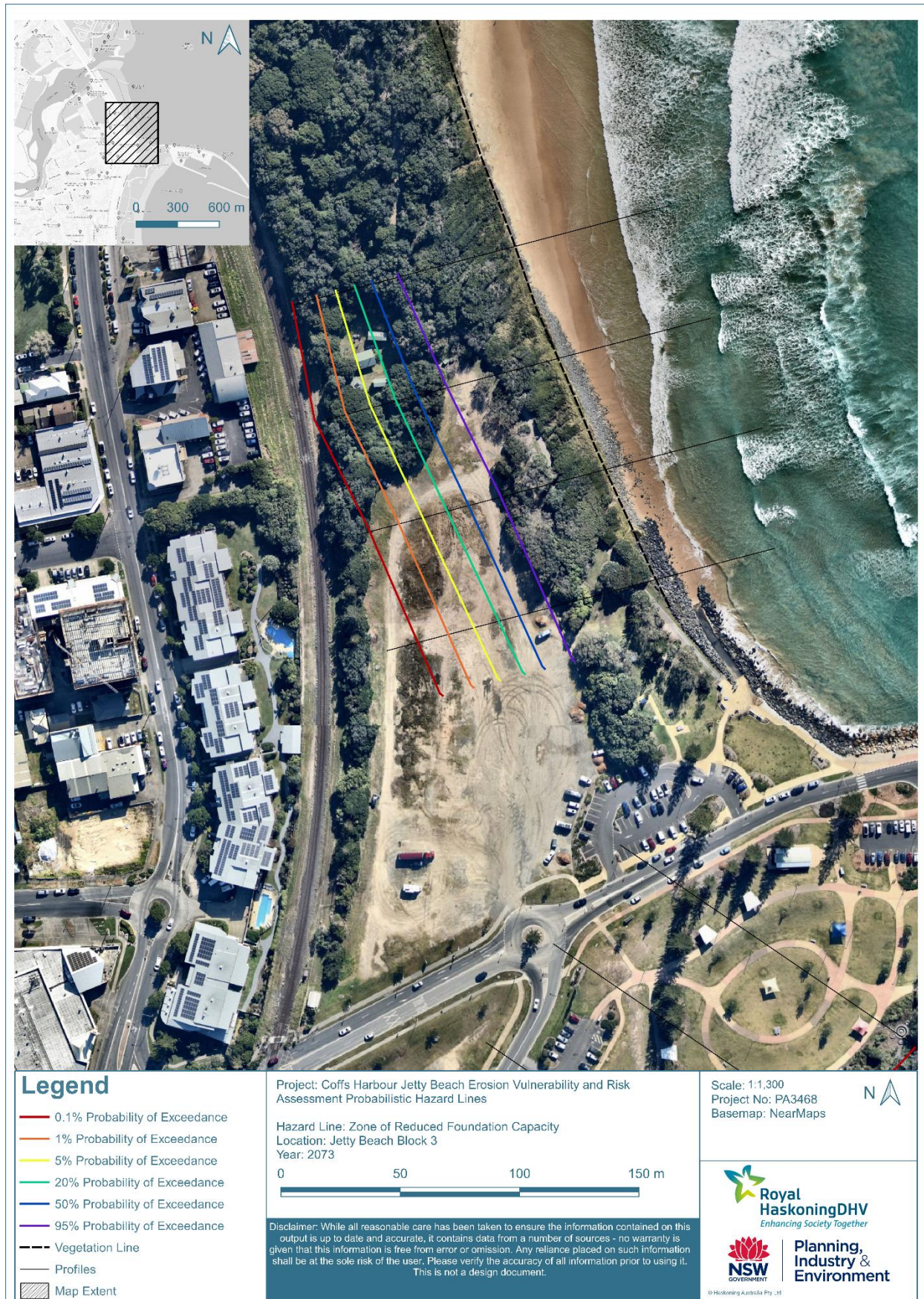
Figure B4-5: Zone of Reduced Foundation Capacity at Jetty Beach Block 3 (2073)
