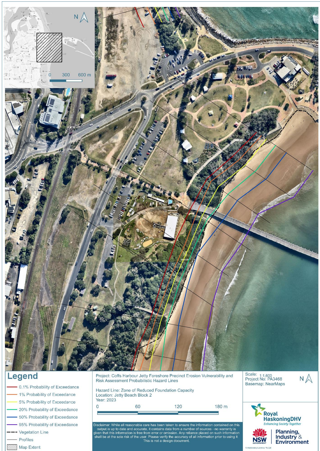
Figure B3-4: Zone of Reduced Foundation Capacity at Jetty Beach Block 2 (2023)
