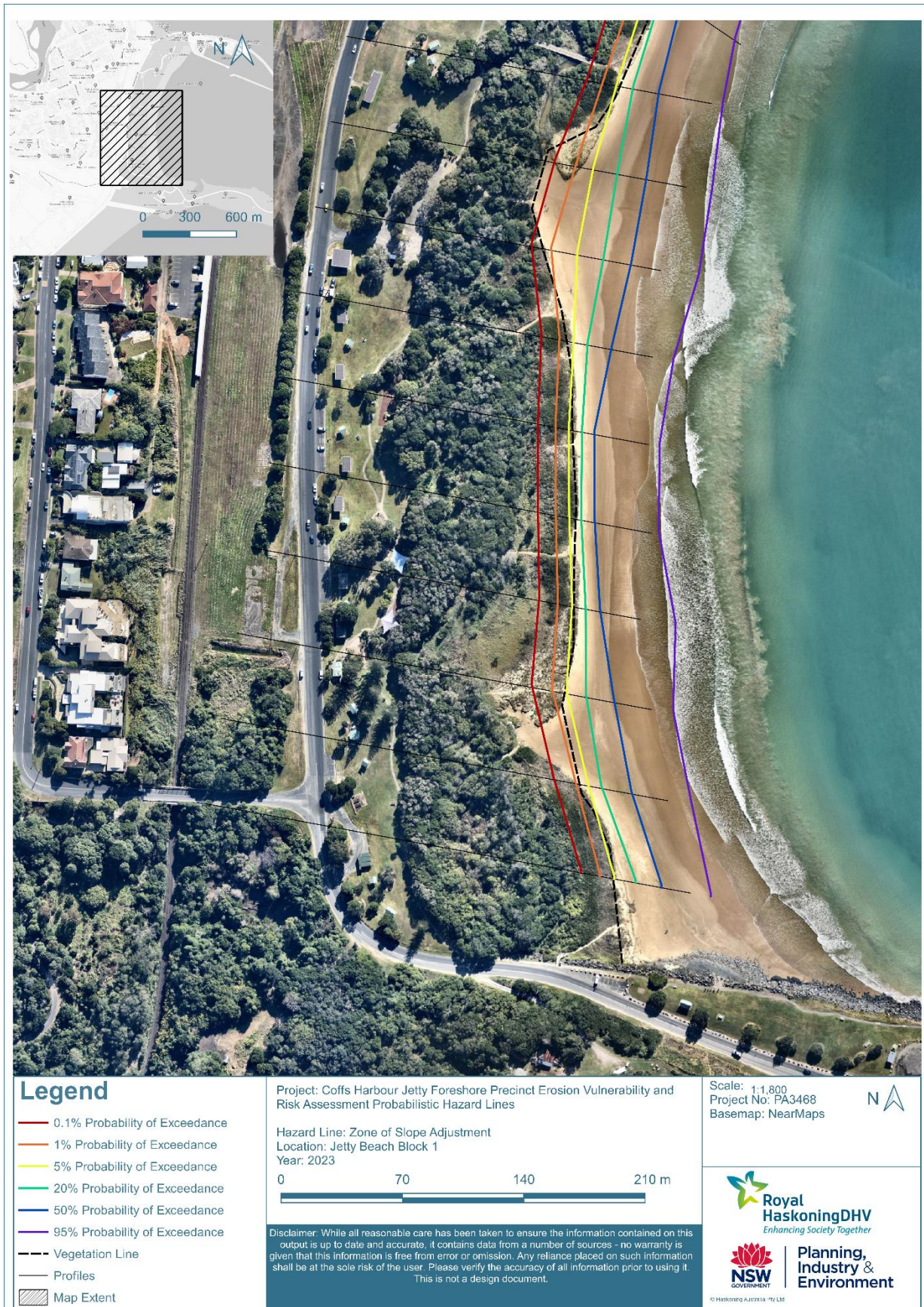
Figure B2-1: Zone of Slope Adjustment at Jetty Beach Block 1 (2023)
