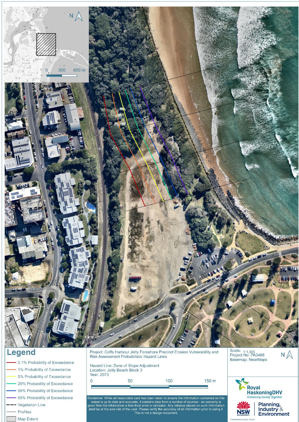
Figure B4-2: Zone of Slope Adjustment at Jetty Beach Block 3 (2073)
