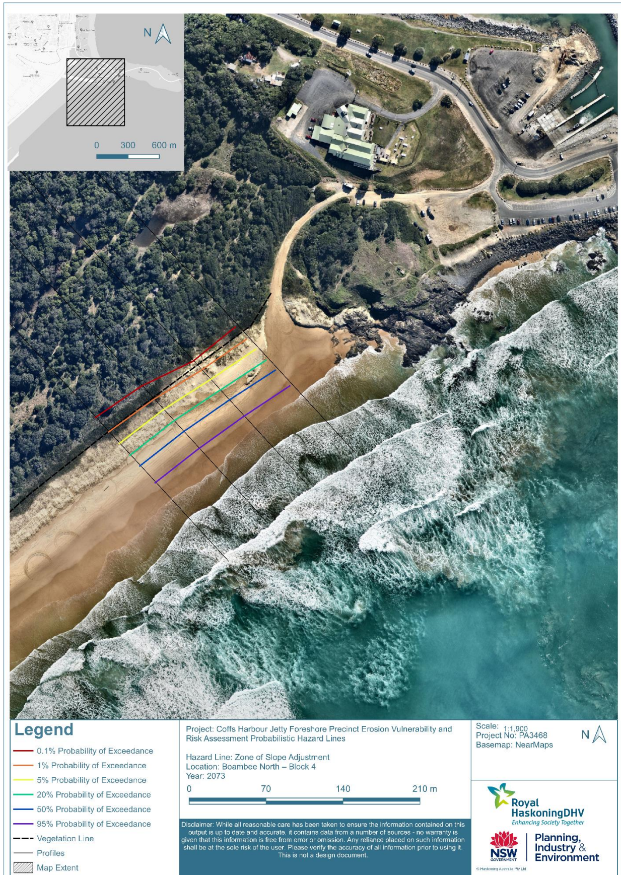
Figure B1-2: Zone of Slope Adjustment at Boambee North (2073)
