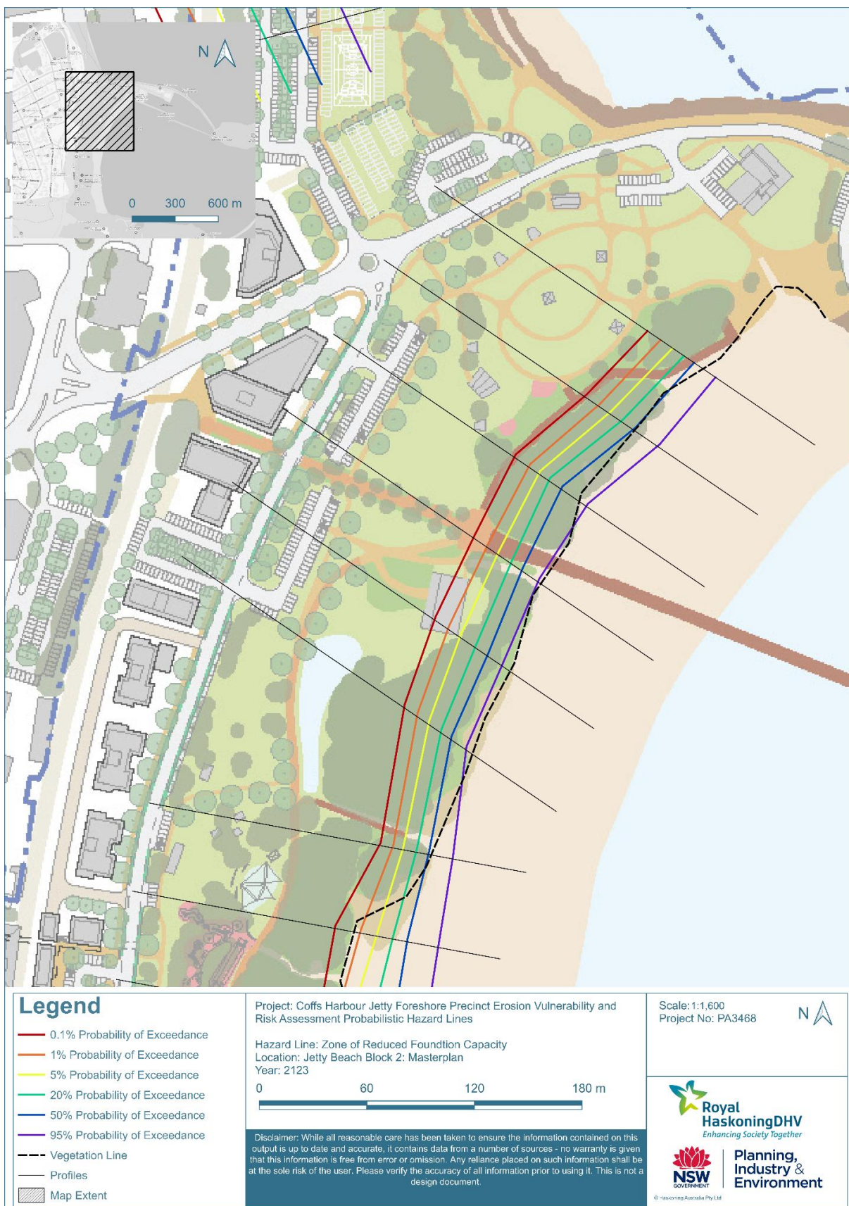
Figure 3-4: Zone of Reduced Foundation Capacity at Jetty Beach Block 2 for the 2123 planning period overlain on the Illustrative Masterplan
