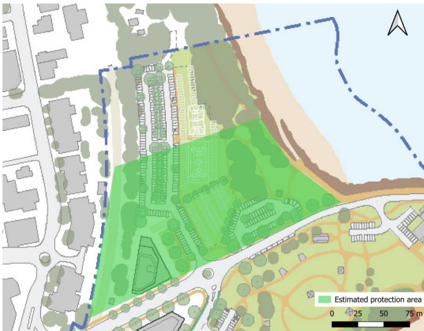
Figure 3-1: Estimated erosion protection area due to revetment wall
