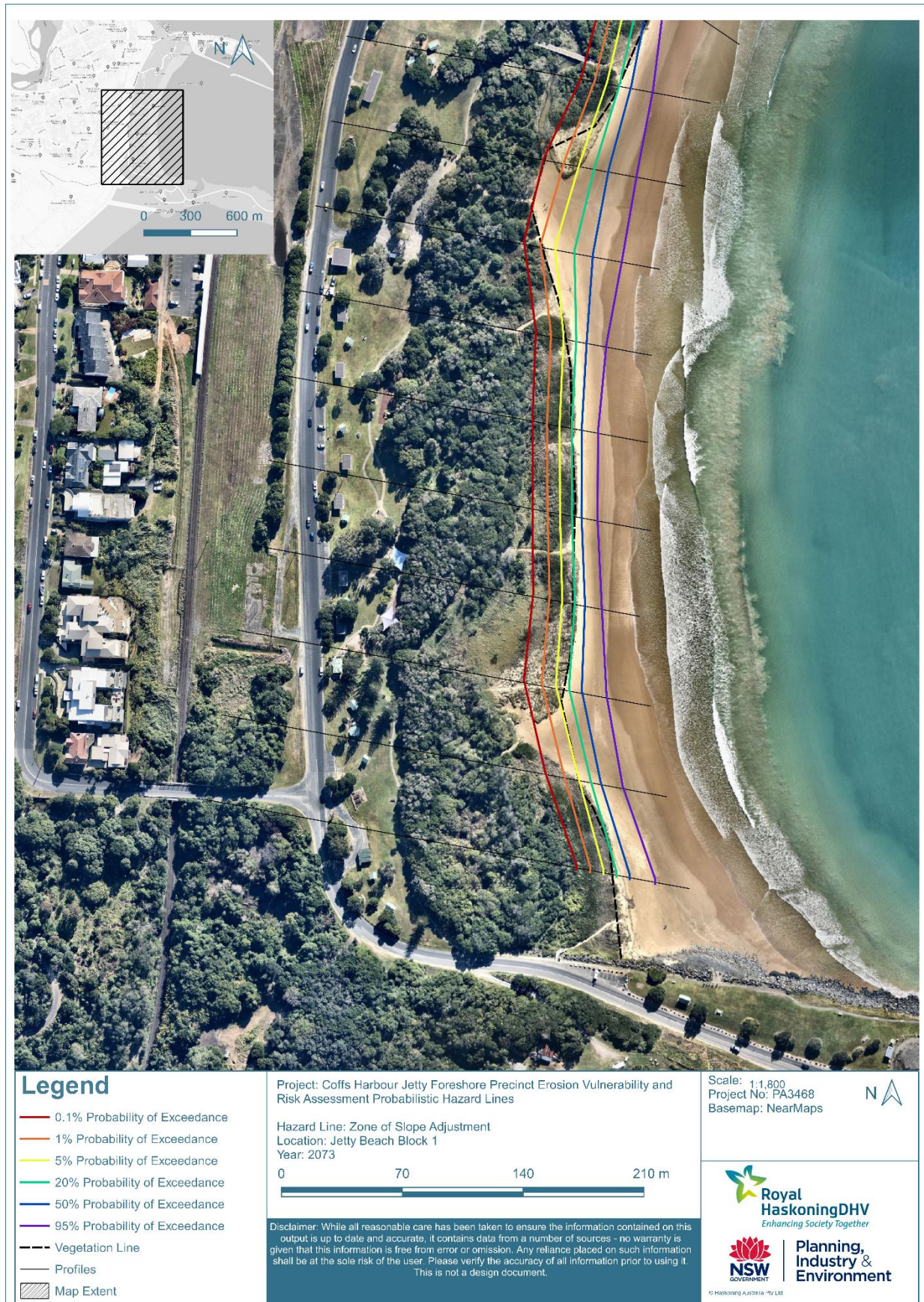
Figure B2-2: Zone of Slope Adjustment at Jetty Beach Block 1 (2073)
