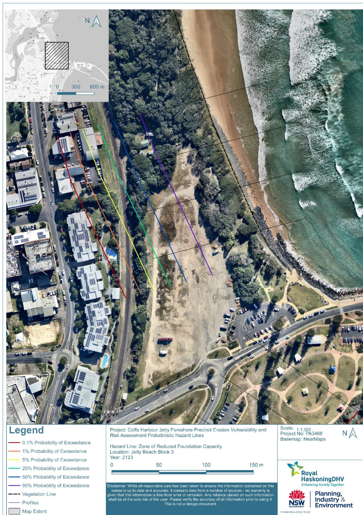
Figure B4-6: Zone of Reduced Foundation Capacity at Jetty Beach Block 3 (2123)
