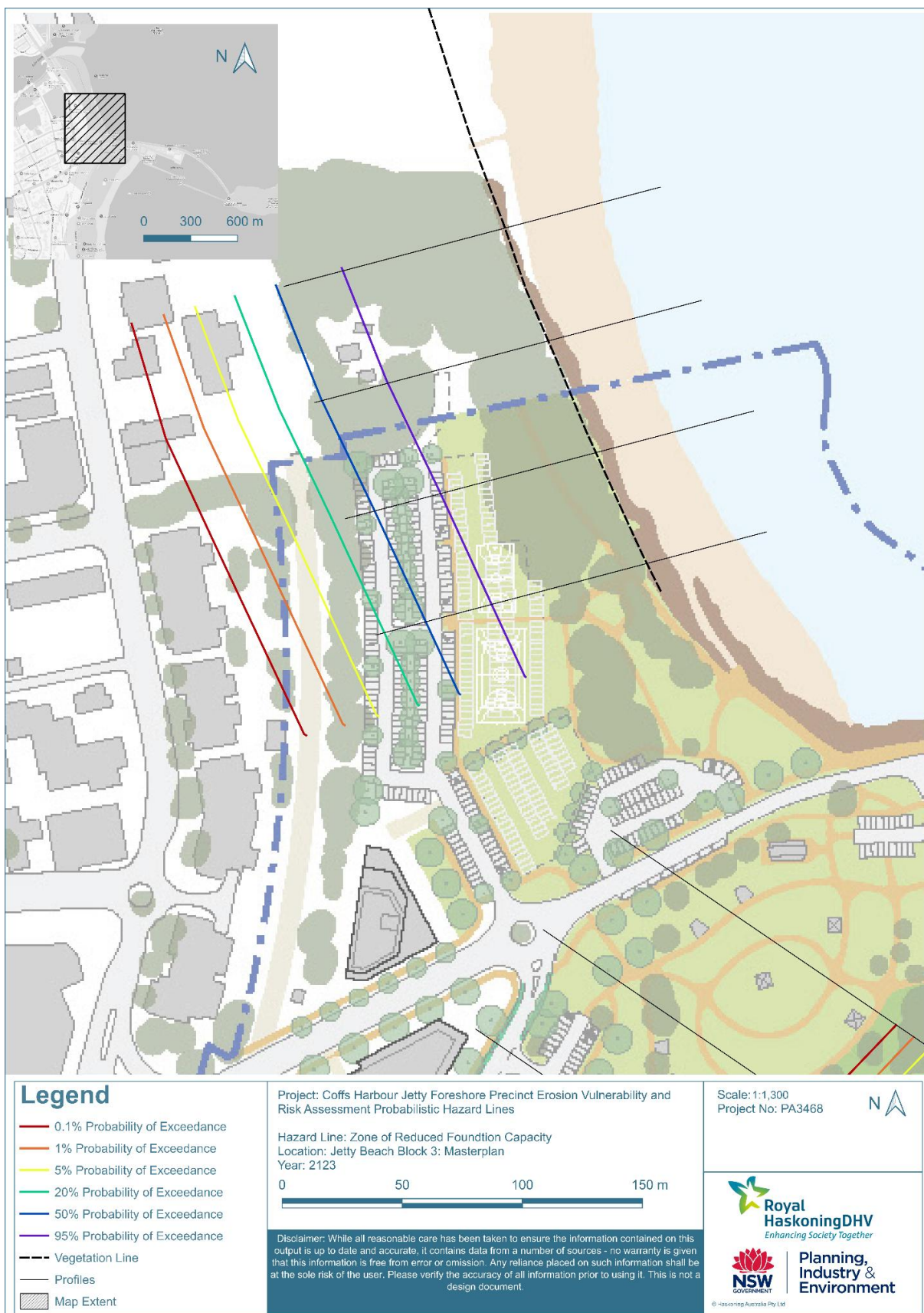
Figure 3-5: Zone of Reduced Foundation Capacity at Jetty Beach Block 3 for the 2123 planning period overlain on the Illustrative Masterplan
