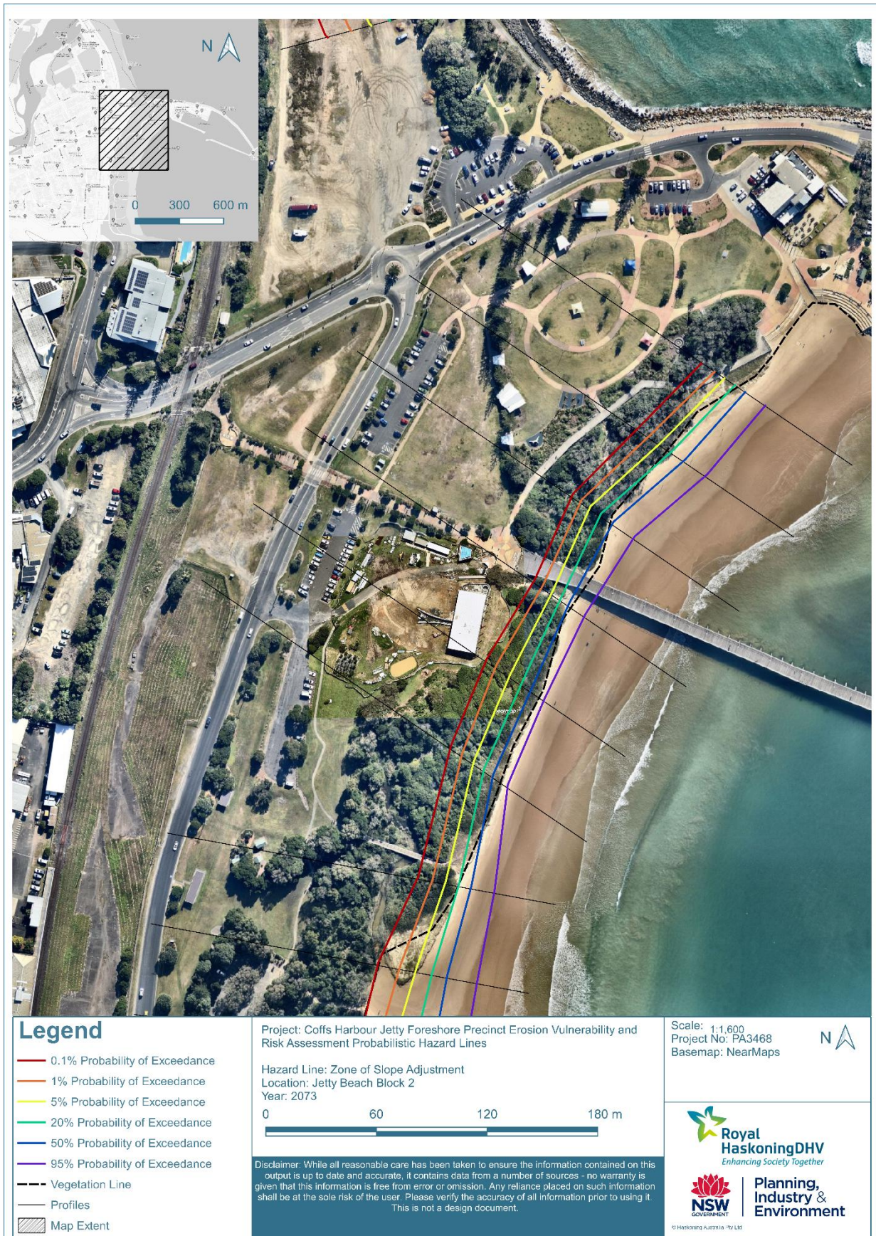
Figure B3-2: Zone of Slope Adjustment at Jetty Beach Block 2 (2073)
