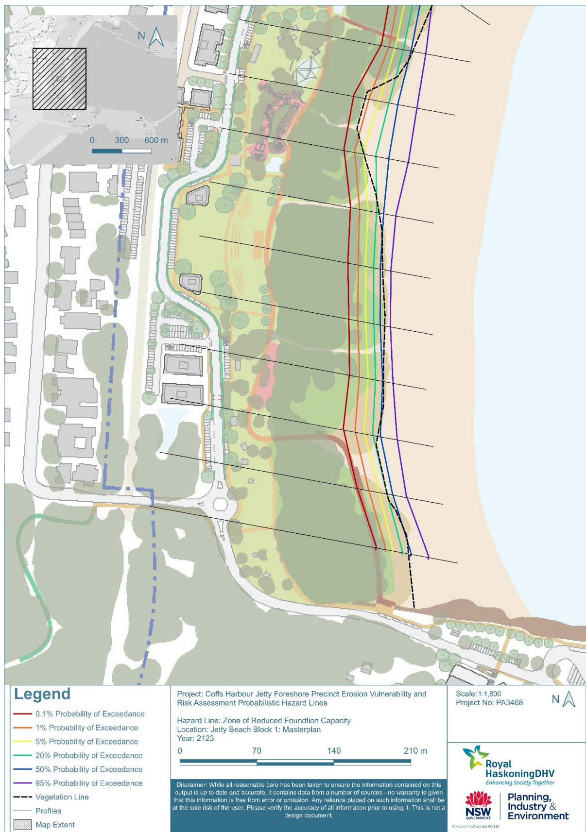
Figure 3-3: Zone of Reduced Foundation Capacity at Jetty Beach Block 1 for the 2123 planning period overlain on the Illustrative Masterplan
