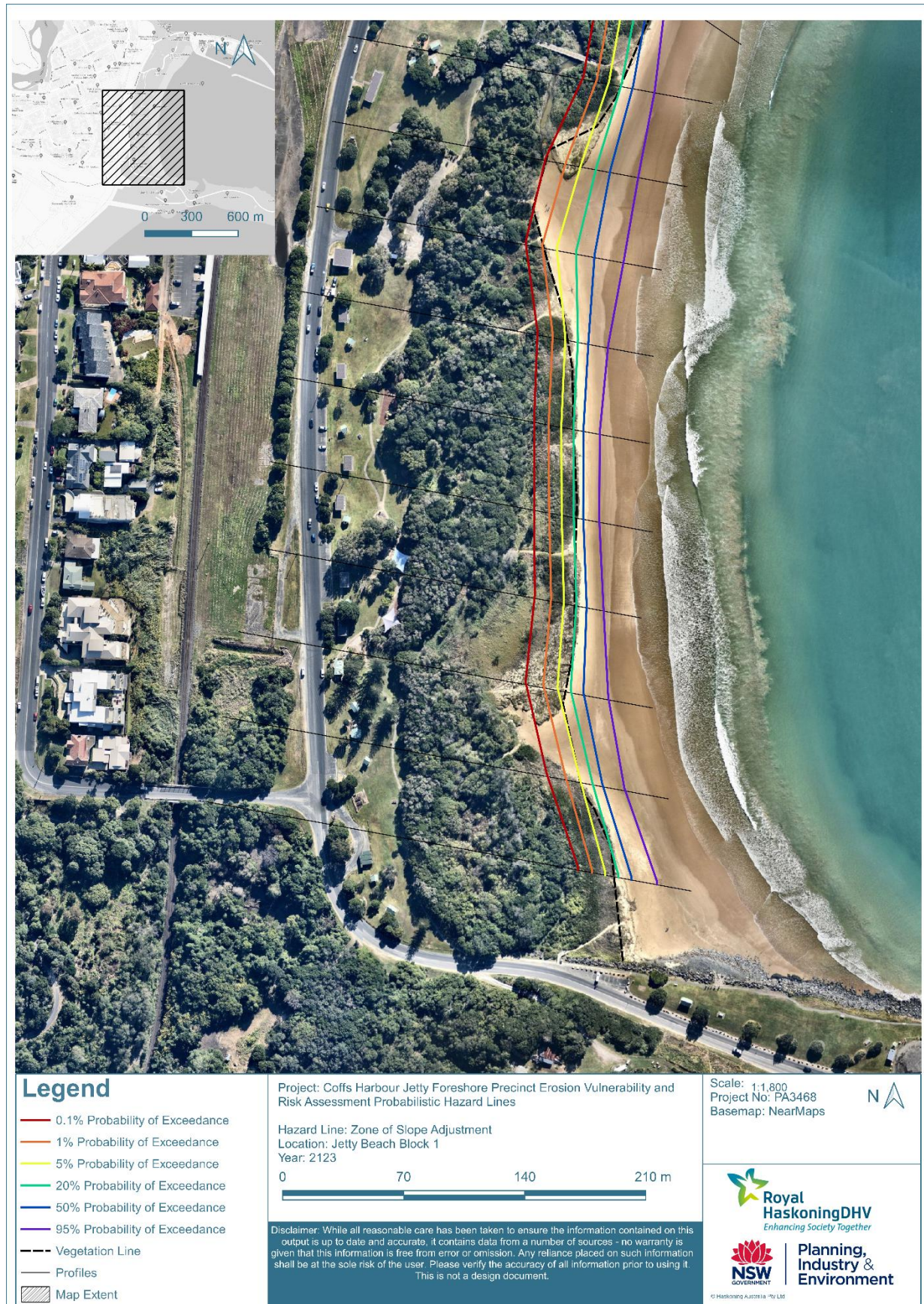
Figure B2-3: Zone of Slope Adjustment at Jetty Beach Block 1 (2123)
