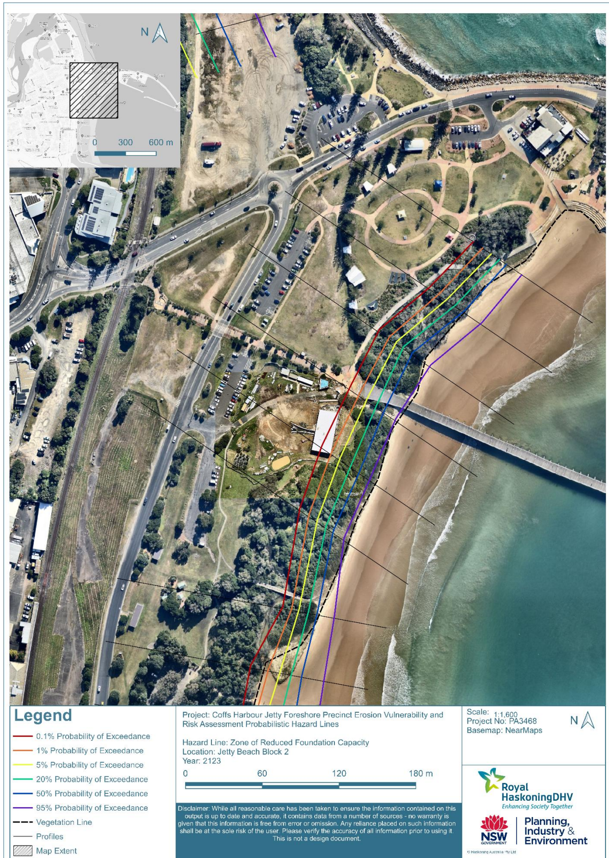
Figure B3-6: Zone of Reduced Foundation Capacity at Jetty Beach Block 2 (2123)
