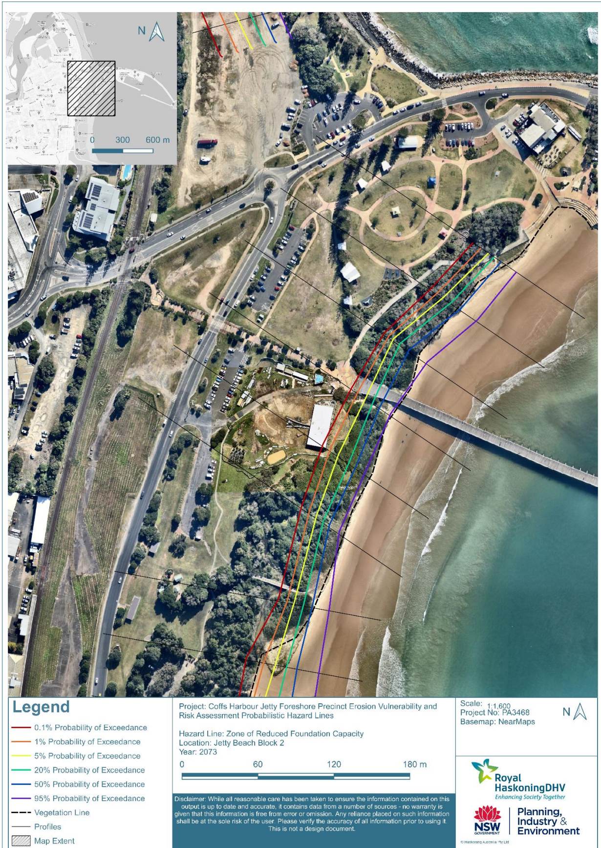
Figure B3-5: Zone of Reduced Foundation Capacity at Jetty Beach Block 2 (2073)
