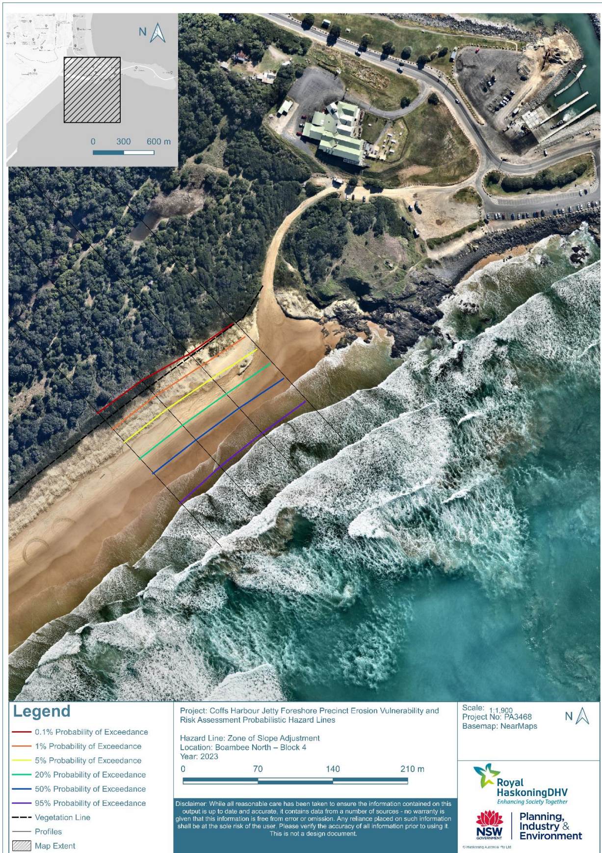
Figure B1-1: Zone of Slope Adjustment at Boambee North (2023)
