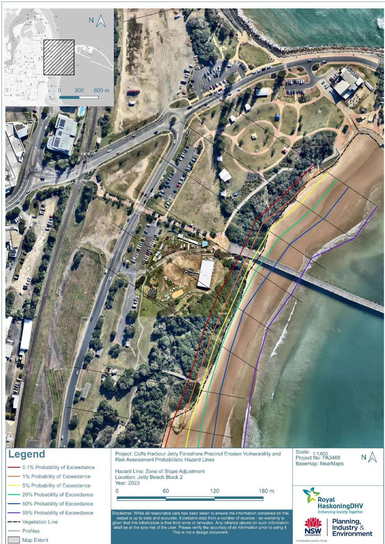
Figure B3-1: Zone of Slope Adjustment at Jetty Beach Block 2 (2023)
