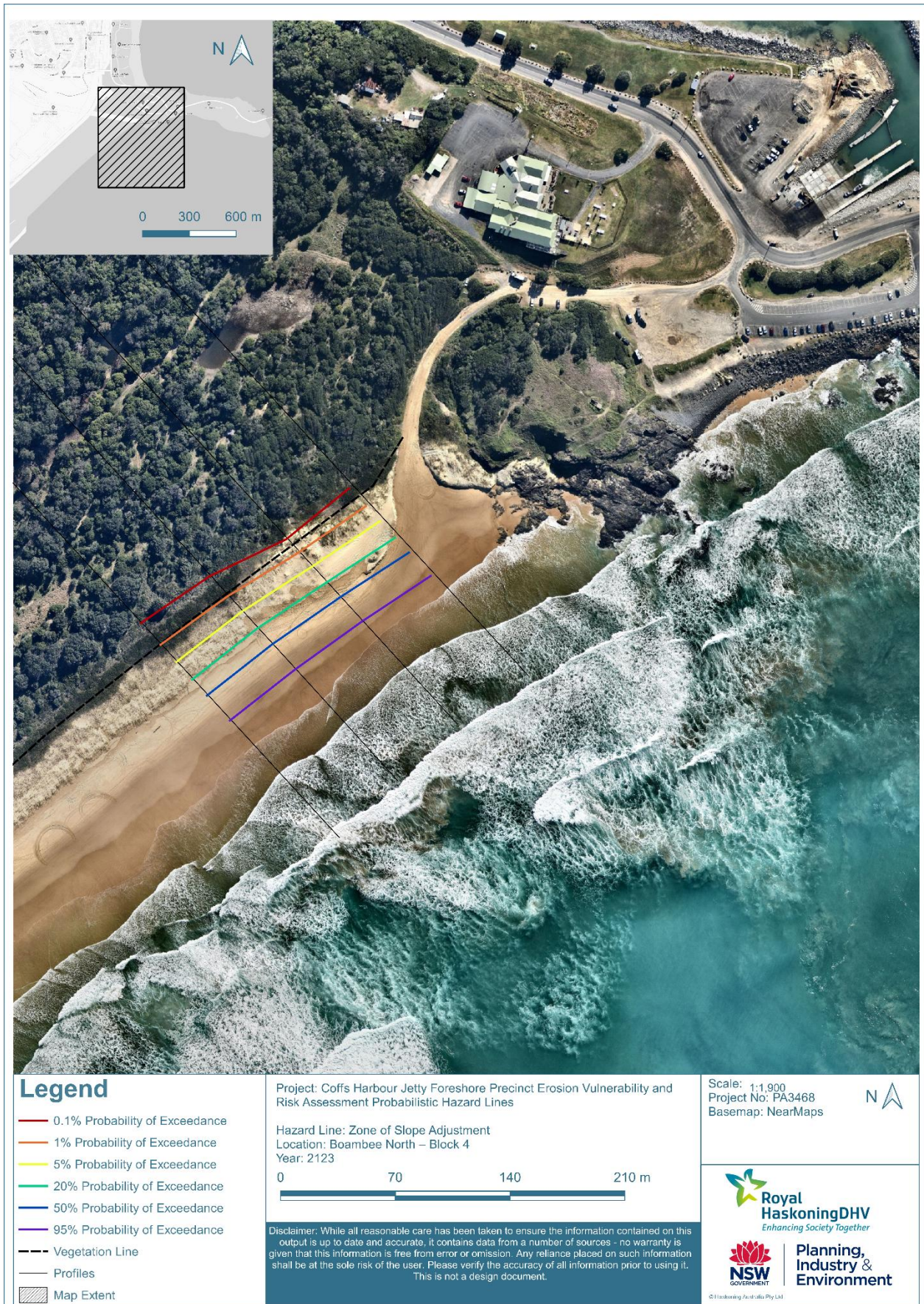
Figure B1-3: Zone of Slope Adjustment at Boambee North (2123)
