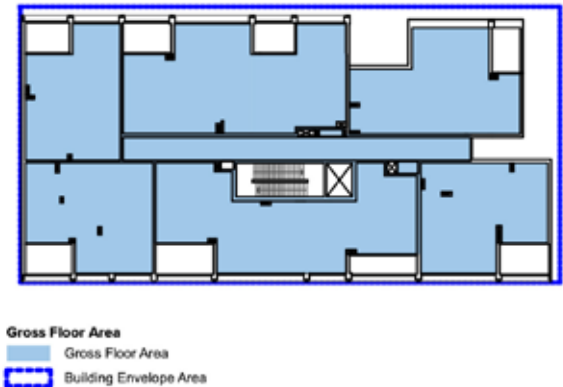
Diagram illustrating Building Envelope Area and Gross Floor Area for a residential floorplate
