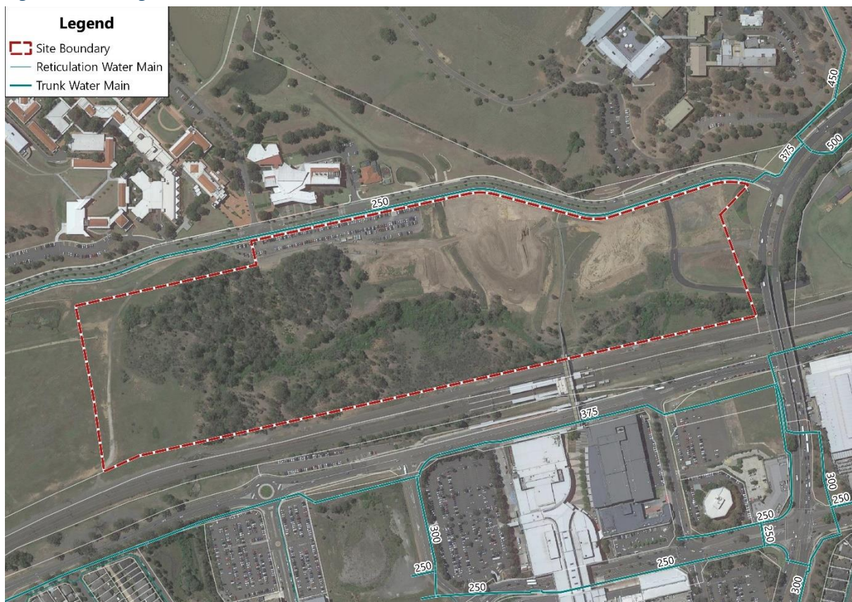
Figure 2 - Existing Potable Water Network
