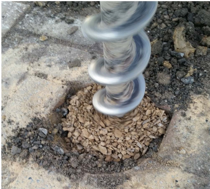
Photo 4 - Chips of weathered shale visible in auger spoil (BH04)
