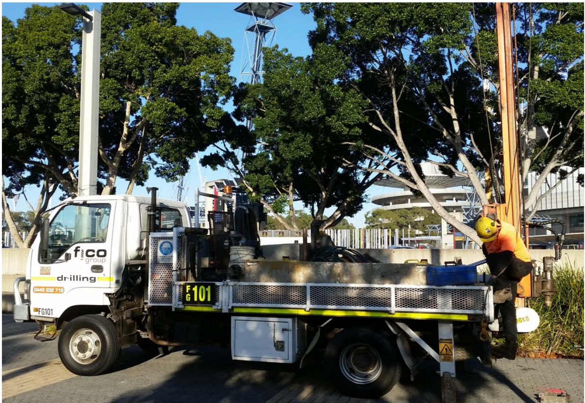
Photo 2 - FG101 drill rig used for augering each borehole
