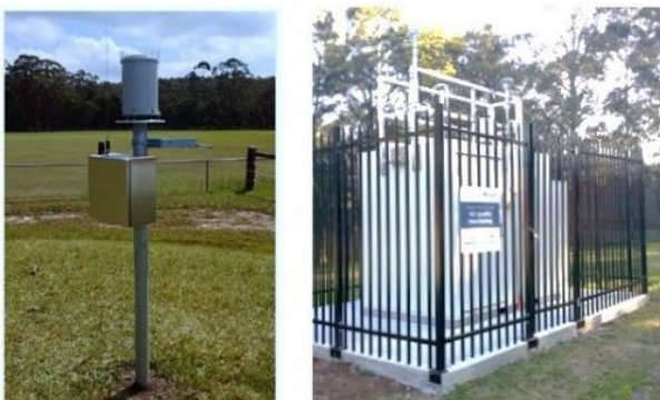
Figure 13 Flood (left) and air quality (right) monitoring stations
