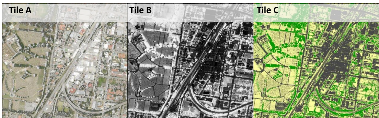
Figure 3: Example combining NDVI assessment with multi-spectral imagery and LiDAR to delineate land cover (ELA 2018)
