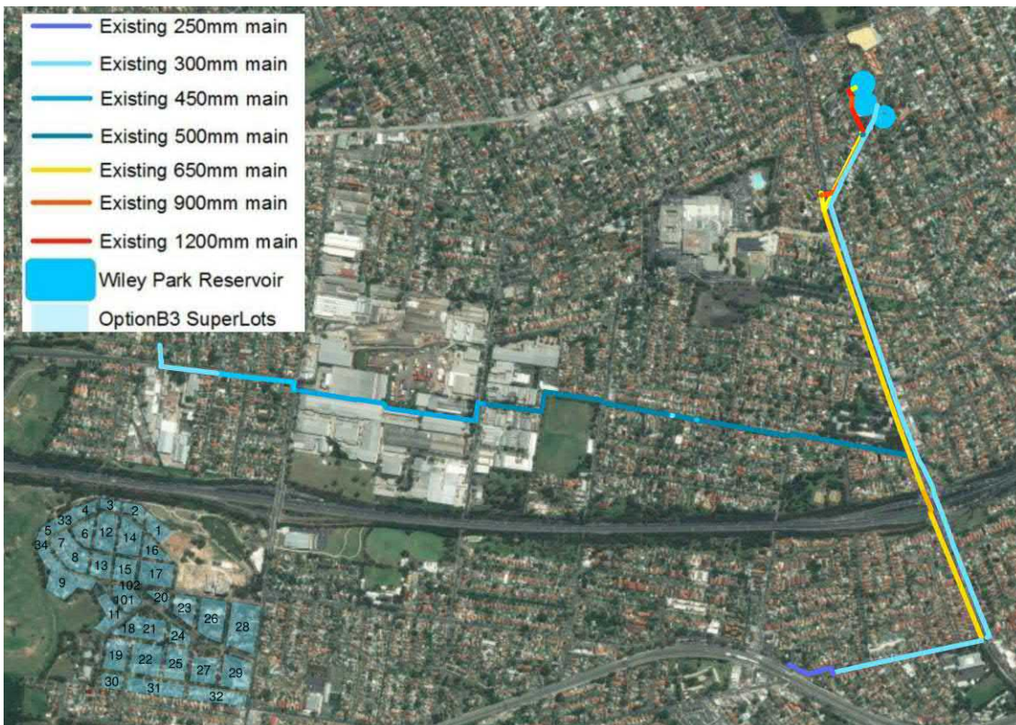
Figure 13: Existing Trunk Water Mains
