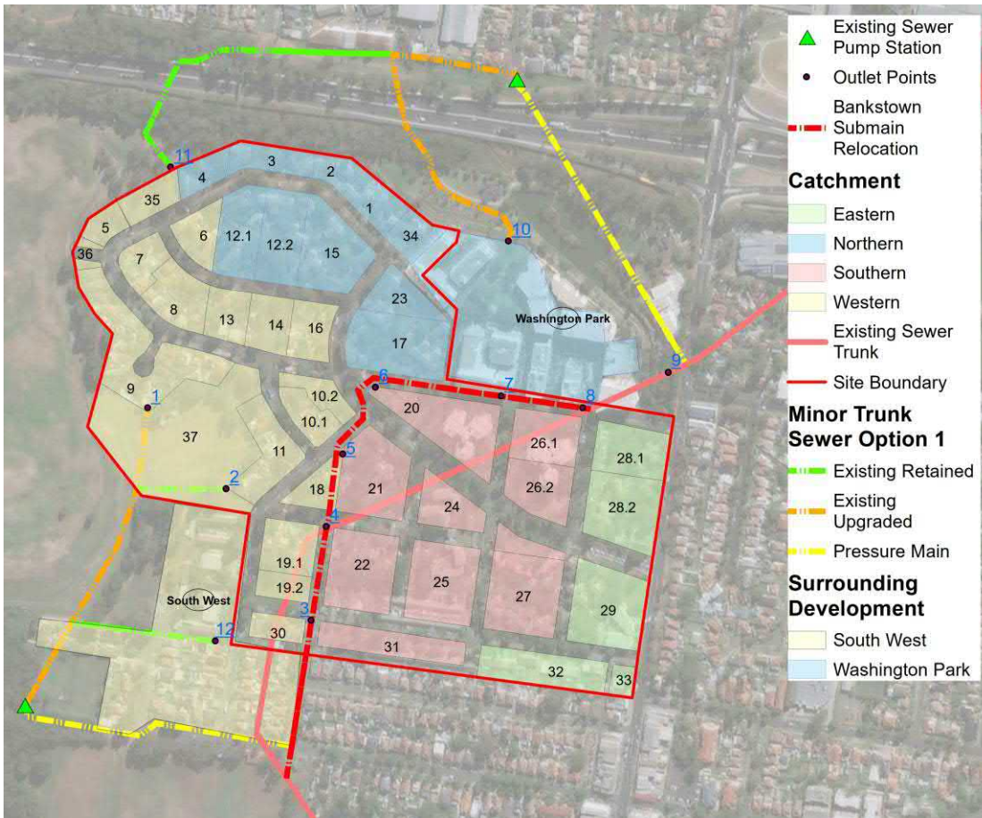
Figure 19: Sewer Upgrades – Option 1
