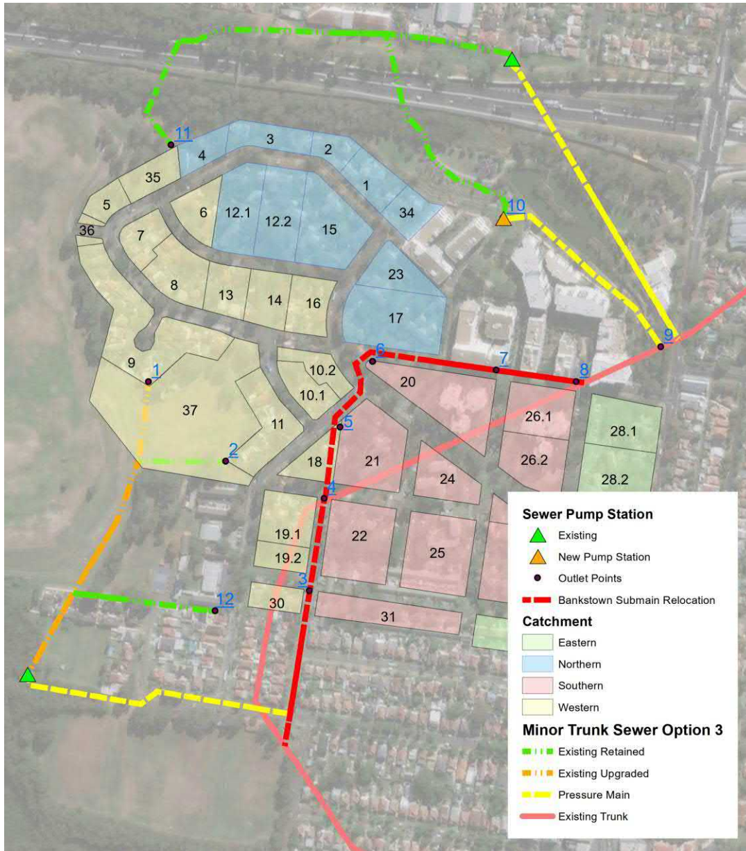
Figure 20: Sewer Upgrades – Option 3
