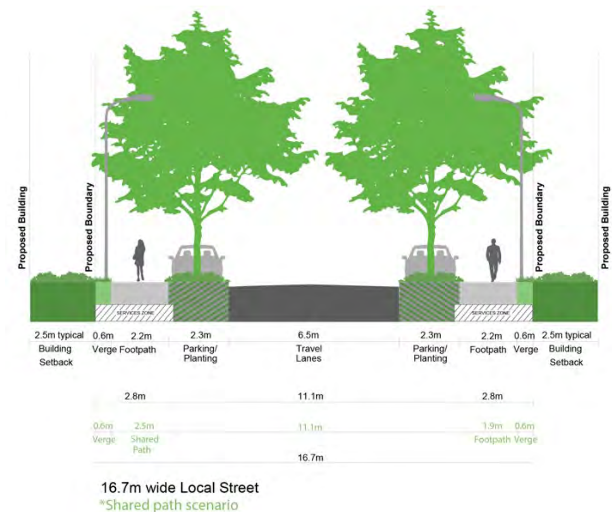
Figure 6.12: Proposed Road Section – Local Street
