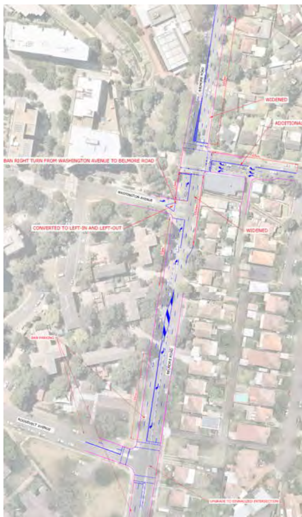
Figure 2-3: Proposed Geometric Layout for Belmore Road North
