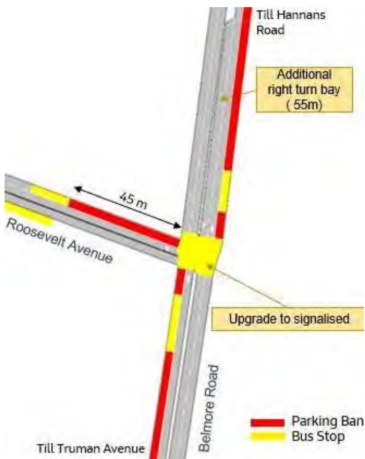
Figure 3-1: Proposed Intersection Layout Belmore Road / Roosevelt Avenue
