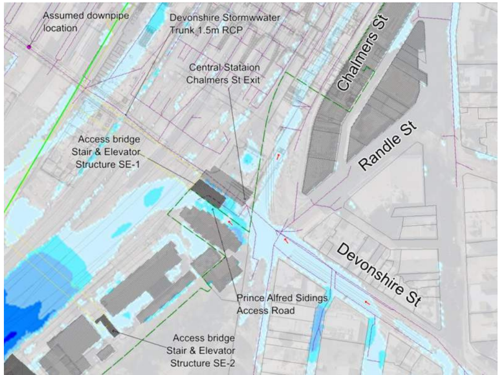
Figure 8-3: Flood Regime - Devonshire St/Chalmers St Intersection - Proposed Conditions (1% AEP)
