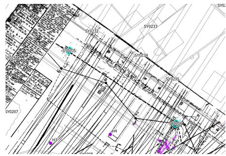
Figure 406. c.1925 N.S.W.G.R. Chief Electrical Engineer's Office plan of the Western Carriage Shed and the surrounding railway tracks, showing the location of the electrical pits. Source: Sydney Trains VPR.
