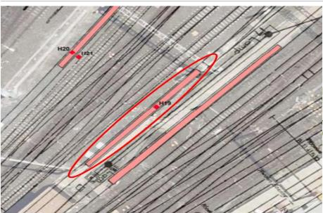
Figure 344. An overlay of the 1928 plan of Sydney Yard showing the location of the ash pit to the south of Platform 8 and the identified remains found during MTMS 2 excavations (H19). Source: Overlay of Mountains Heritage 2021 Sydney Trains VPR.
