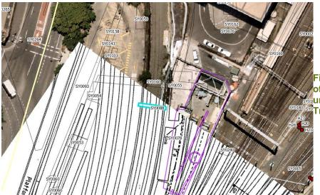
Figure 192. 1992 tracing of a 1954 plan of Sydney Yard, showing the underground services. Source: Sydney Trains VPR.
