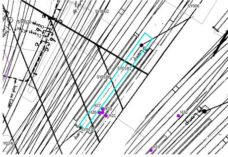
Figure 365. A c.1925 N.S.W.G.R. Chief Electrical Engineer's Office plan of the Western Carriage Shed and the surrounding railway tracks, showing the location of the ash pit. Source: Sydney Trains, B/27846, 0045989\_T0C.
