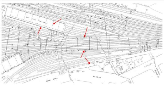
Figure 246. 1992 tracing of a 1954 plan of Sydney Yard, showing the underground track drains and grated pits. Source: Sydney Trains VPR
