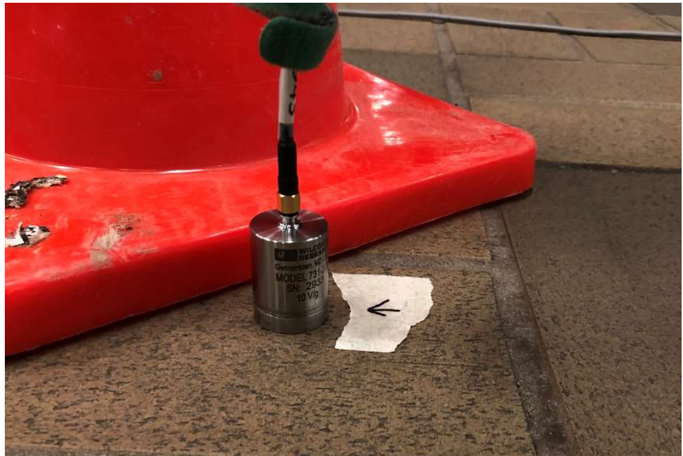
Figure 4-4 Typical Accelerometer Mounting Arrangement
