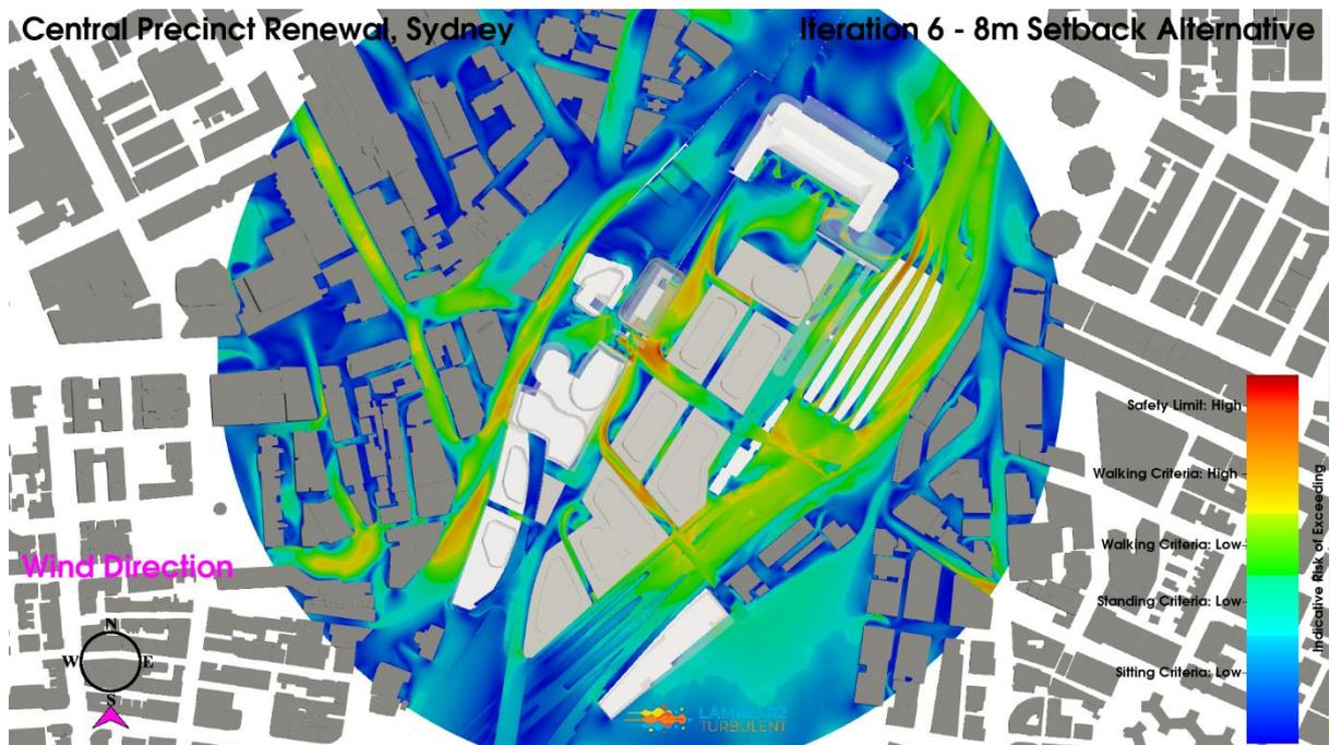
**Figure 160: Iteration 6 – 8m Setback Alternative Configuration, South Wind Direction, Planview, Pedestrian Level Environmental Wind Risk Contour Plot**
