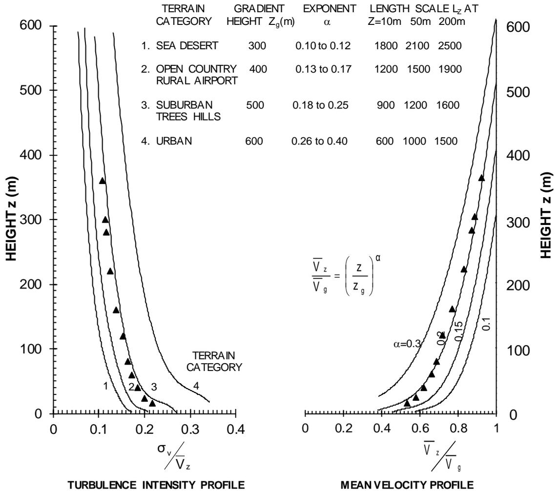
Figure 2 – 1/400 scale TC3 boundary layer turbulence intensity and mean velocity profiles in the MEL Consultants Boundary Layer Wind Tunnel 4.8 m x 2.2 m working section, scaled to full-scale dimensions.
