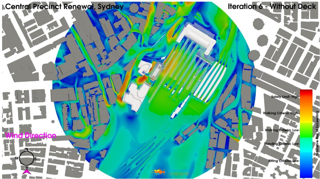
**Figure 112: Iteration 6 – Without Deck Configuration, South Wind Direction, Planview, Pedestrian Level Environmental Wind Risk Contour Plot**
