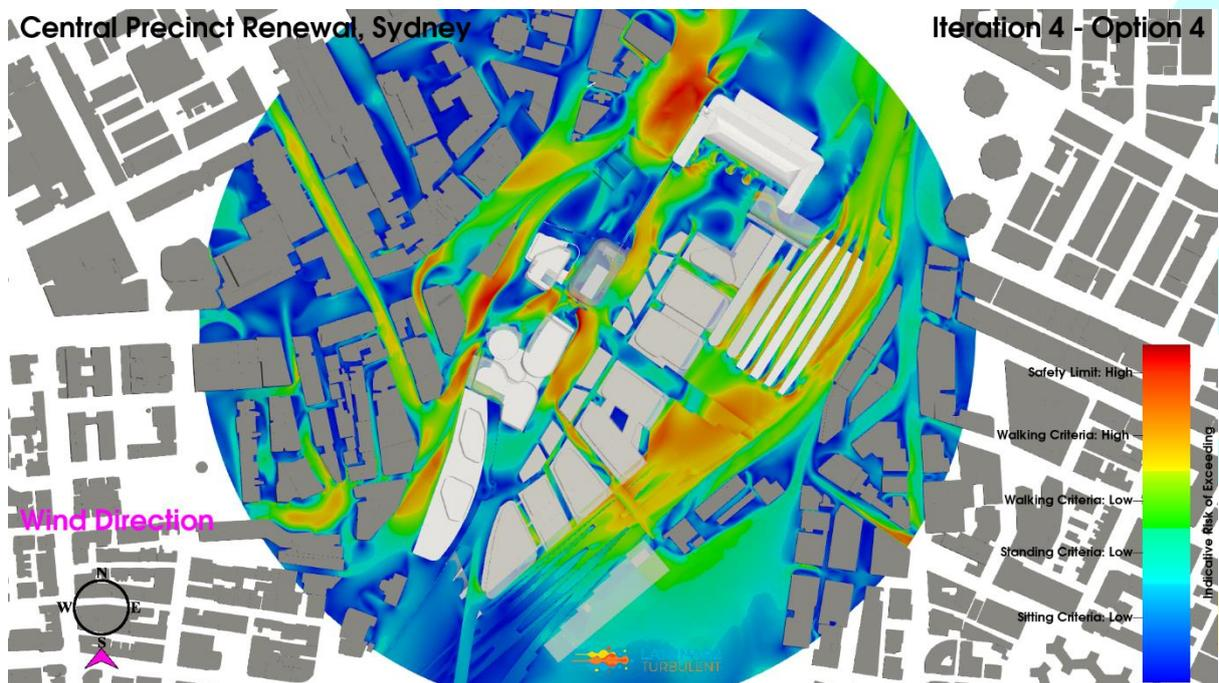
**Figure 68: Iteration 4 – Option 4 Configuration, South Wind Direction, Planview, Pedestrian Level Environmental Wind Risk Contour Plot**
