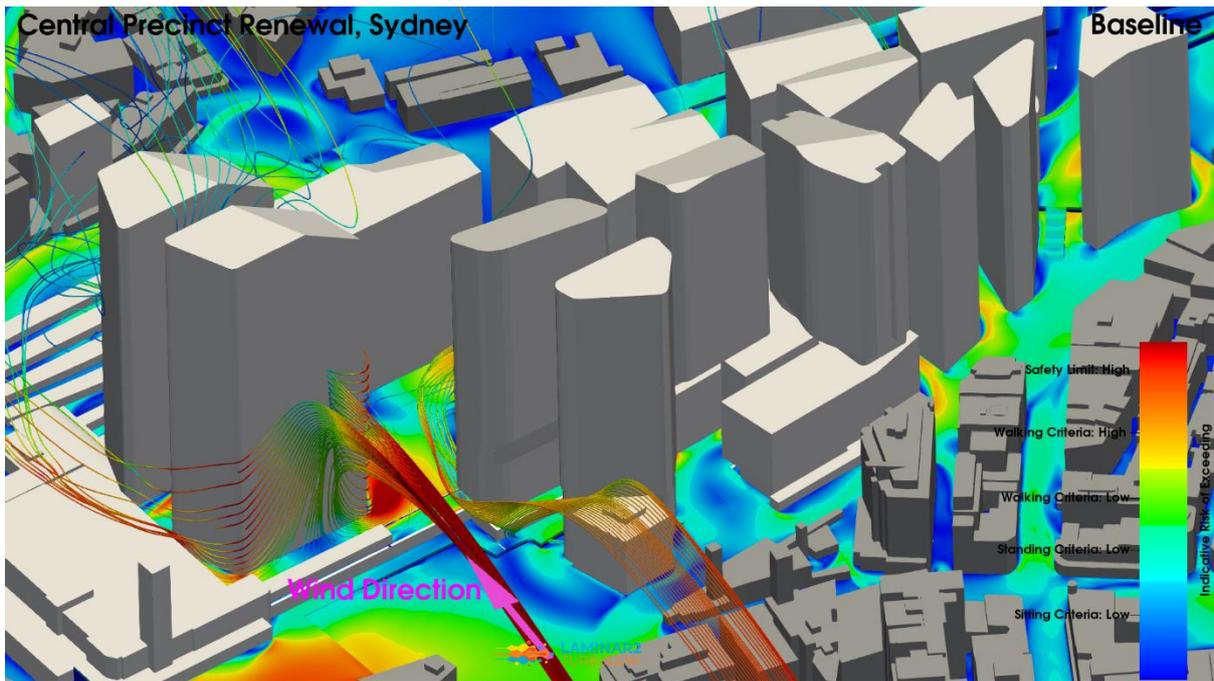
**Figure 16: Baseline Configuration, Northwest Wind Direction, Streamlines, Pedestrian Level Environmental Wind Risk Contour Plot**
