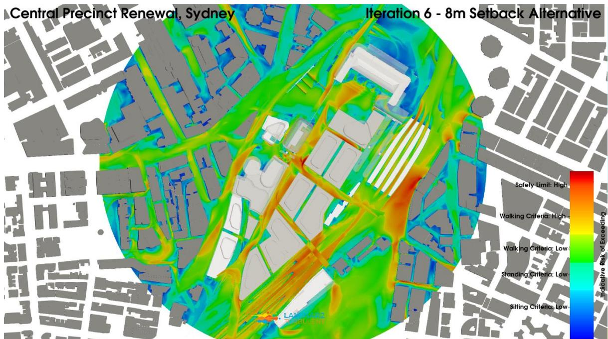
**Figure 164: Iteration 6 – 8m Setback Alternative Configuration, Combined Wind Directions, Planview, Maximum Pedestrian Level Environmental Wind Risk Contour Plot**
