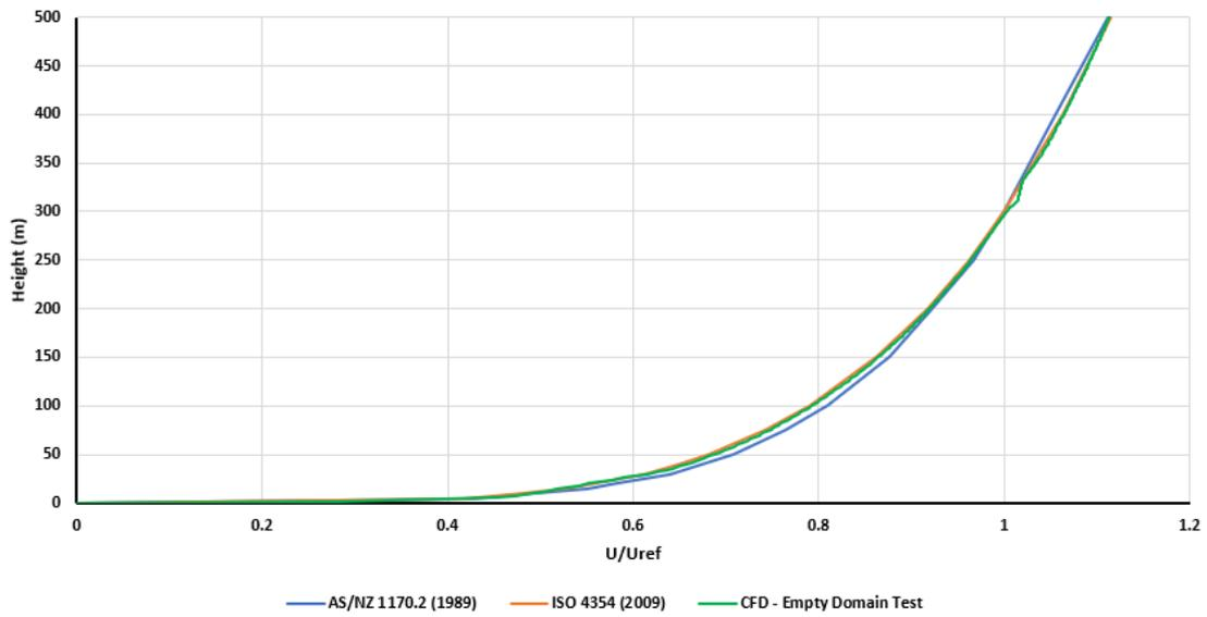
**Figure 2: Full scale TC3 boundary layer mean velocity profile for all wind directions**
