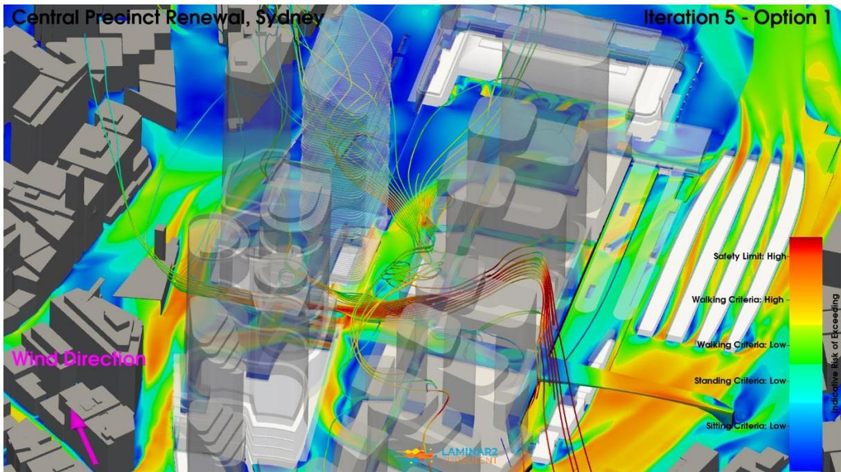
**Figure 86: Iteration 5 – Option 1 Configuration, South Wind Direction, Streamlines & Pedestrian Level Environmental Wind Risk Contour Plot**
