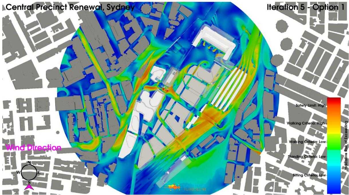
**Figure 84: Iteration 5 - Option 1 Configuration, South Wind Direction, Planview, Pedestrian Level Environmental Wind Risk Contour Plot**
