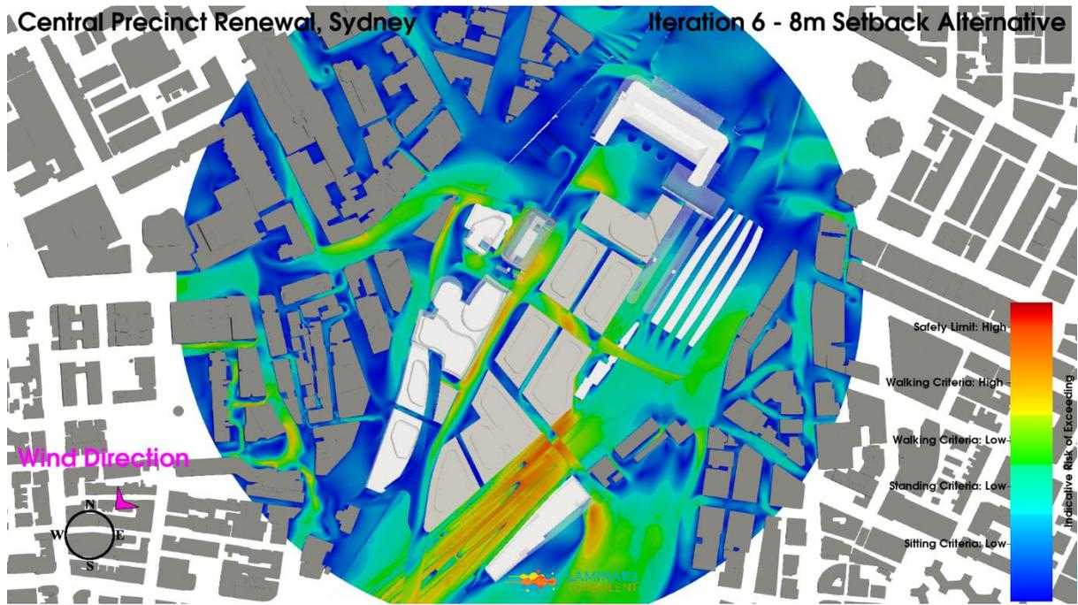
**Figure 157: Iteration 6 - 8m Setback Alternative Configuration, Northeast Wind Direction, Planview, Pedestrian Level Environmental Wind Risk Contour Plot**
