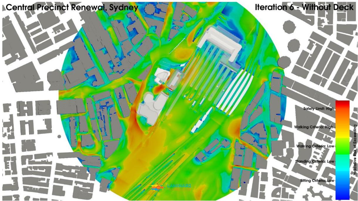
**Figure 116: Iteration 6 – Baseline Without Deck Configuration, Combined Wind Directions, Planview, Maximum Pedestrian Level Environmental Wind Risk**
