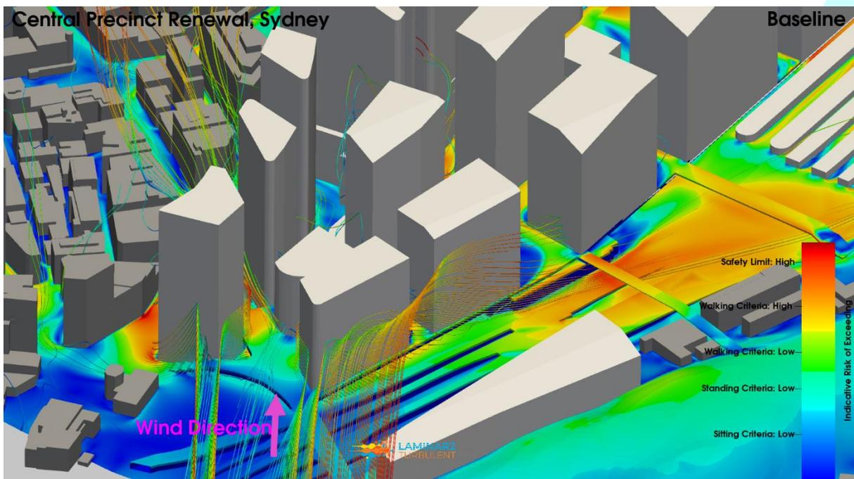
**Figure 15: Baseline Configuration, South Wind Direction, Streamlines, Pedestrian Level Environmental Wind Risk Contour Plot**
