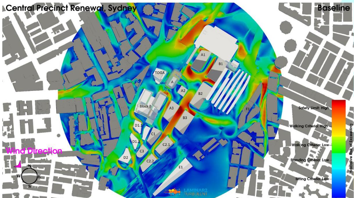
**Figure 13: Baseline Configuration, Northwest Wind Direction, Planview, Ground Level Pedestrian Environmental Wind Risk Contour Plot**
