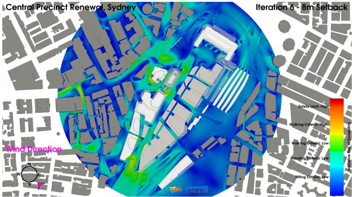
**Figure 146: Iteration 6 – 8m Setback Configuration, Southeast Wind Direction, Planview, Pedestrian Level Environmental Wind Risk Contour Plot**
