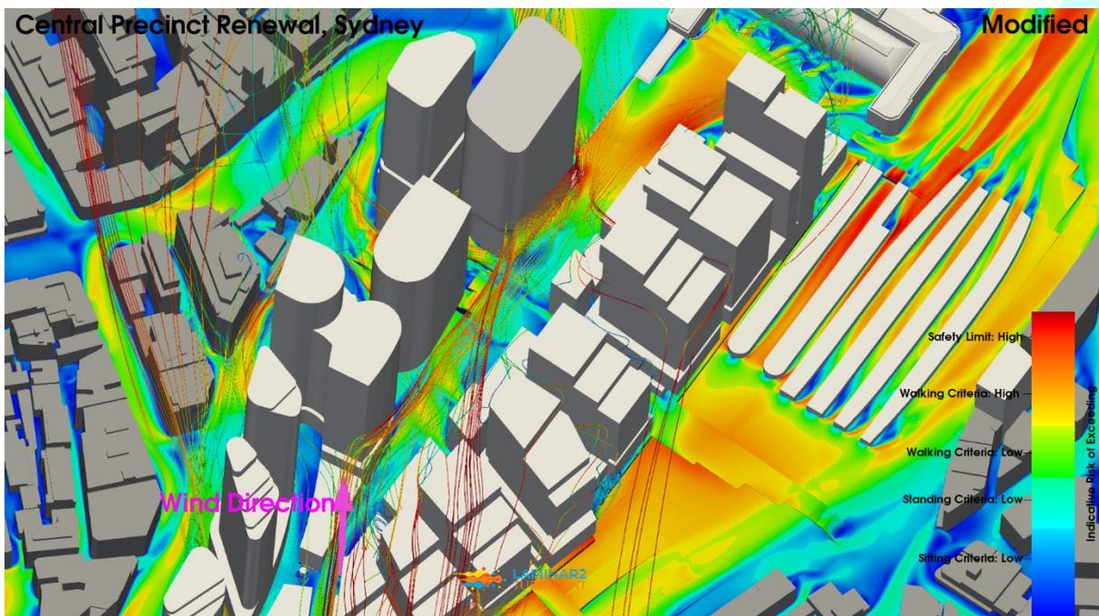
**Figure 33: Iteration 1 Configuration, South Wind Direction (alternate view), Streamlines, Pedestrian Level Environmental Wind Risk Contour Plot**
