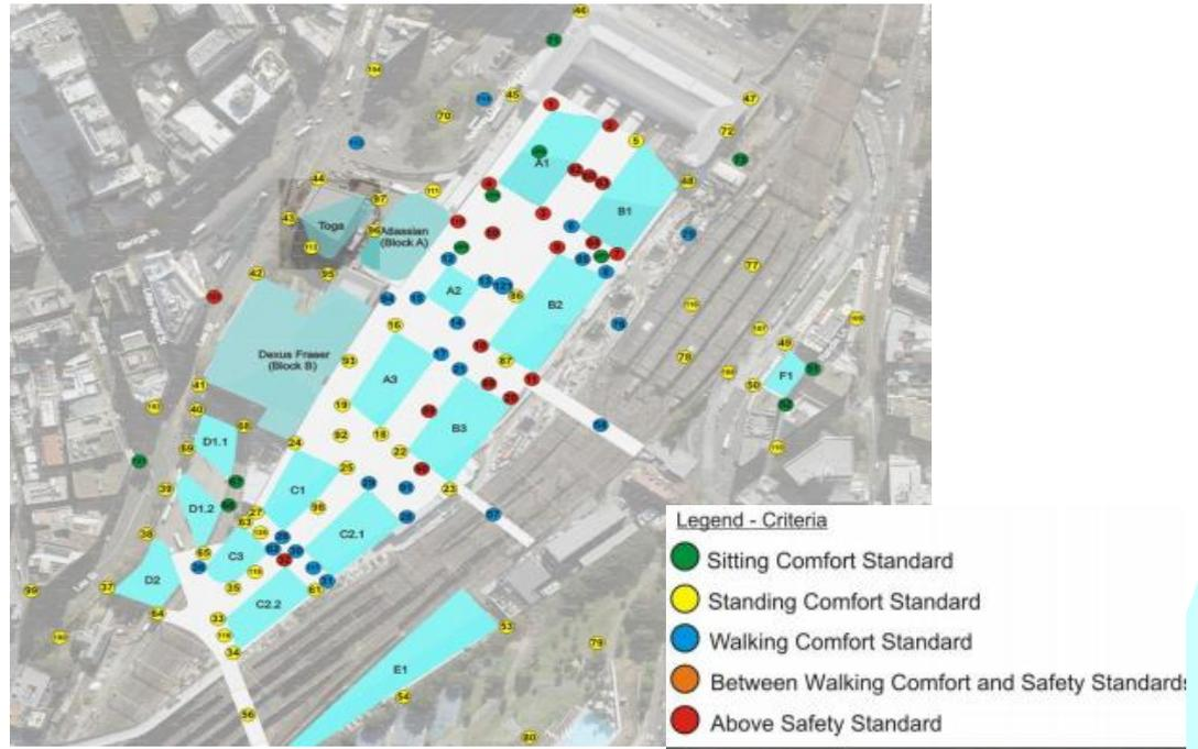
**Figure 18: Wind Tunnel Results, Baseline Configuration, Combined Wind Directions, Planview, Ground Level Maximum Pedestrian Environmental Wind Risk Contour Plot**
