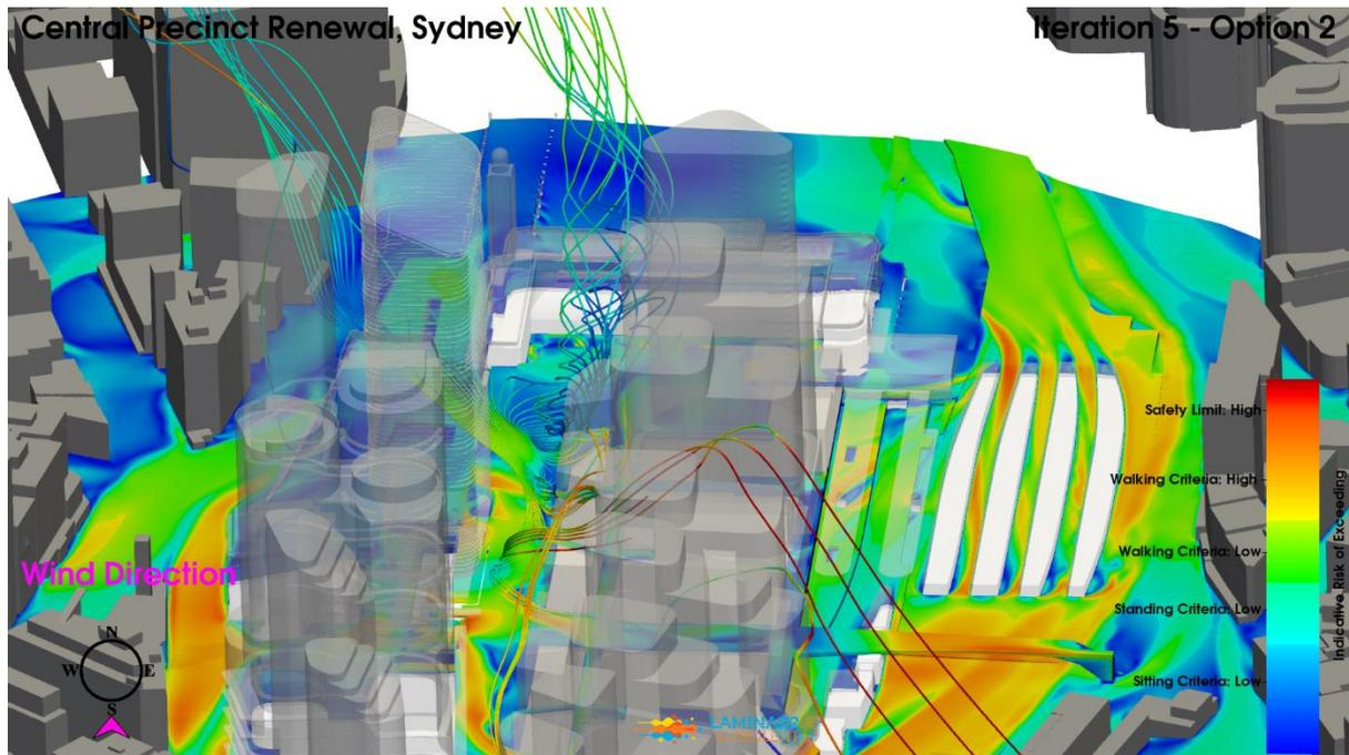
**Figure 94: Iteration 5 – Option 2 Configuration, South Wind Direction, Streamlines & Pedestrian Level Environmental Wind Risk Contour Plot**
