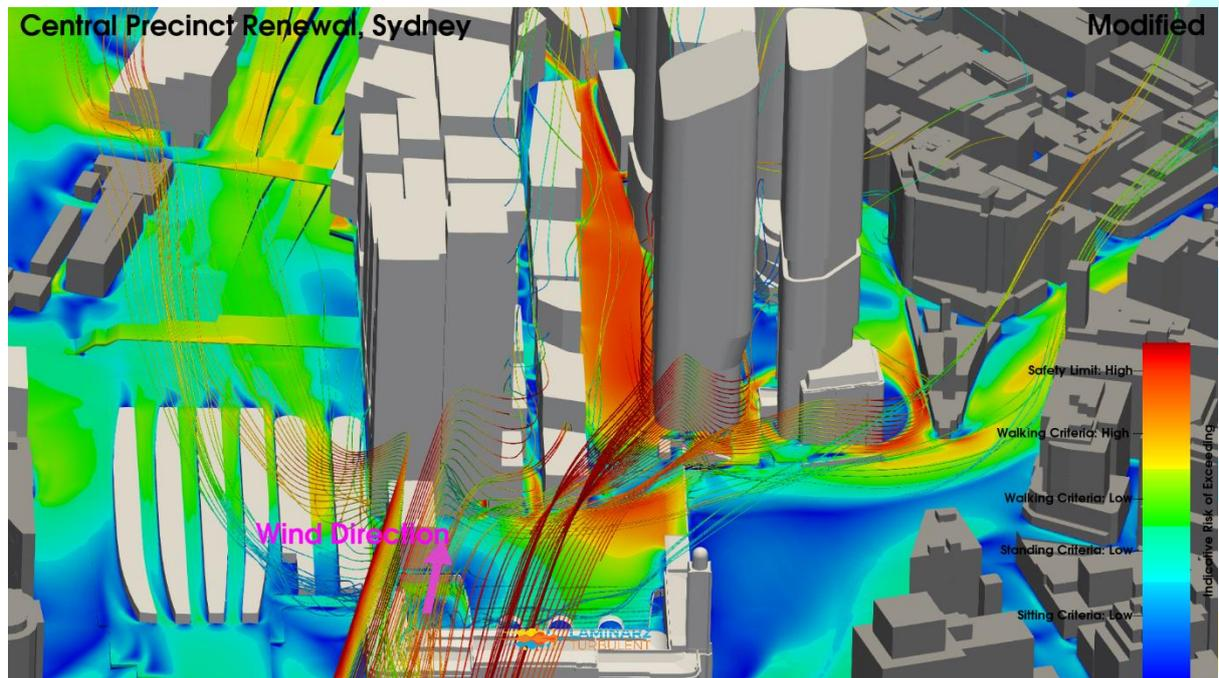
**Figure 31: Iteration 1 Configuration, Northeast Wind Direction, Streamlines, Pedestrian Level Environmental Wind Risk Contour Plot**
