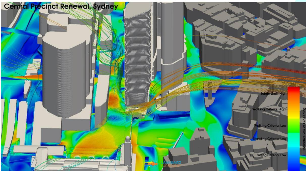
**Figure 133: Iteration 6 – Revised Preferred Massing Configuration, Northwest Wind Direction, Streamlines & Pedestrian Level Environmental Wind Risk Contour Plot**
