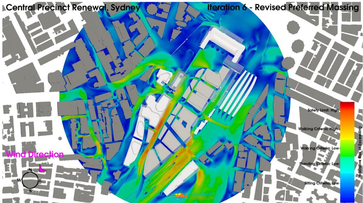
**Figure 122: Iteration 6 - Revised Preferred Massing Configuration, Northeast Wind Direction, Planview, Pedestrian Level Environmental Wind Risk Contour**
