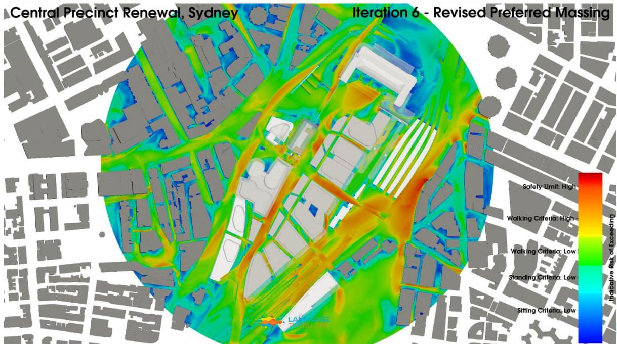
**Figure 130: Iteration 6 - Revised Preferred Massing Configuration, Combined Wind Directions, Planview, Maximum Pedestrian Level Environmental Wind Risk Contour Plot**
