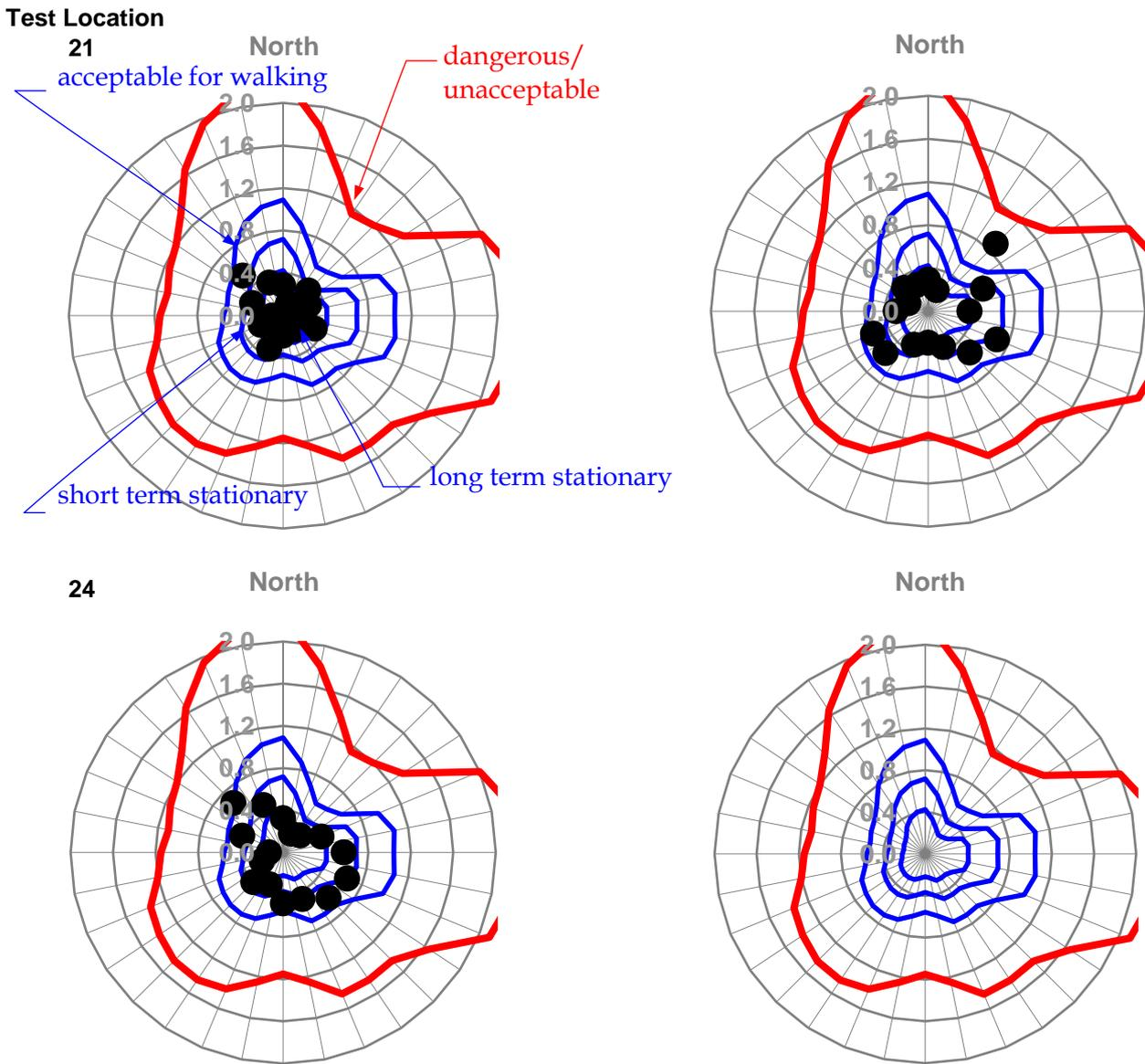
Peak velocity squared ratio  $\left| \frac{\widehat{V}_{local}}{\widehat{V}_{300m}} \right|^2$  as a function of wind direction
