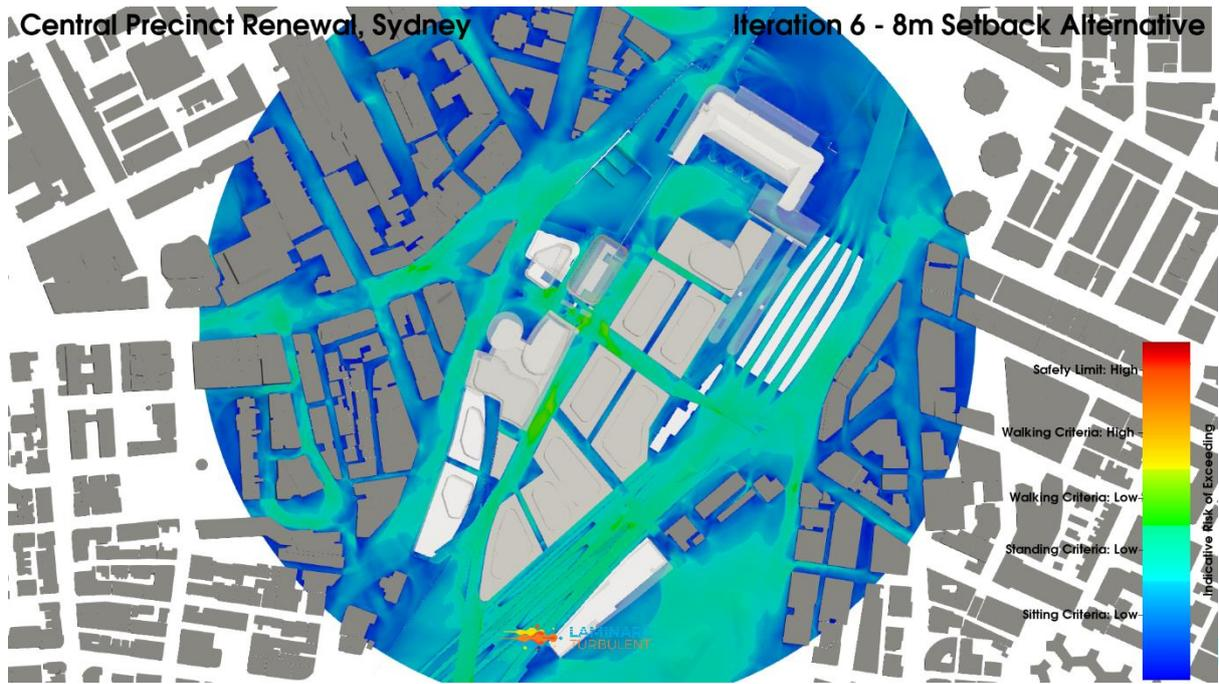
**Figure 165: Iteration 6 – 8m Setback Alternative Configuration, Combined Wind Directions, Planview, Average Pedestrian Level Environmental Wind Risk Contour Plot**
