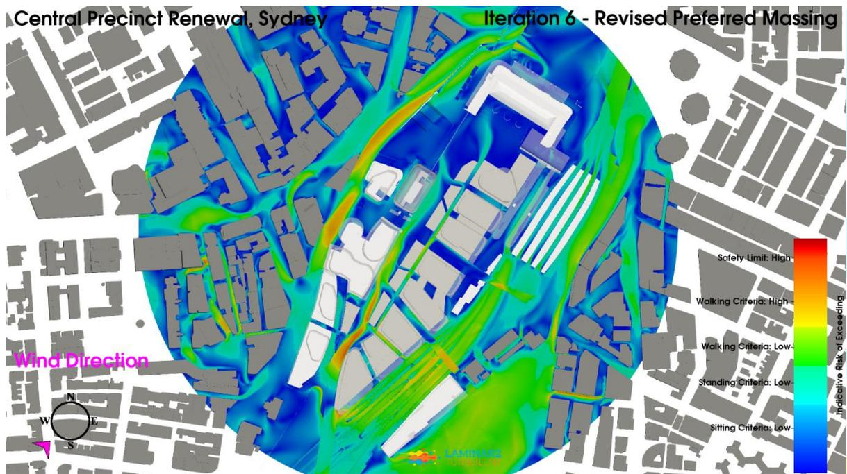
**Figure 127: Iteration 6 – Revised Preferred Massing Configuration, Southwest Wind Direction, Planview, Pedestrian Level Environmental Wind Risk Contour Plot**
