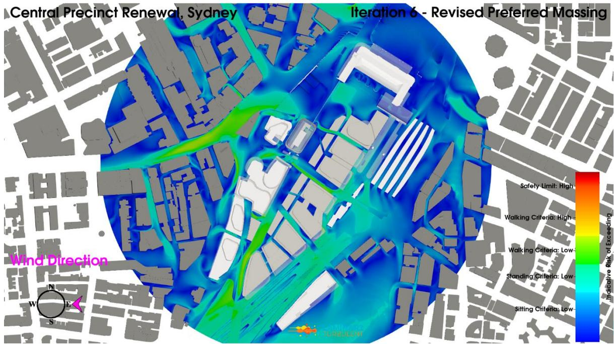
**Figure 124: Iteration 6 – Revised Preferred Massing Configuration, East Wind Direction, Planview, Pedestrian Level Environmental Wind Risk Contour Plot**
