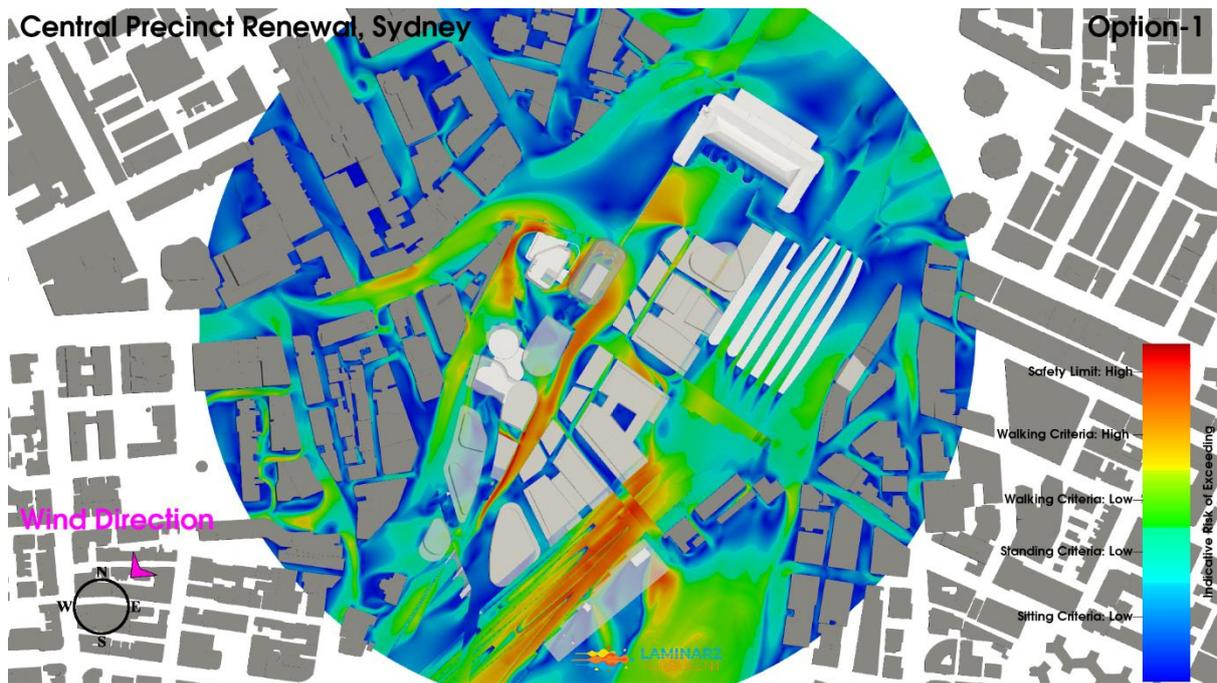
**Figure 38: Iteration 2 – Option 1 Configuration, Northeast Wind Direction, Planview, Ground Level Pedestrian Environmental Wind Risk Contour Plot**
