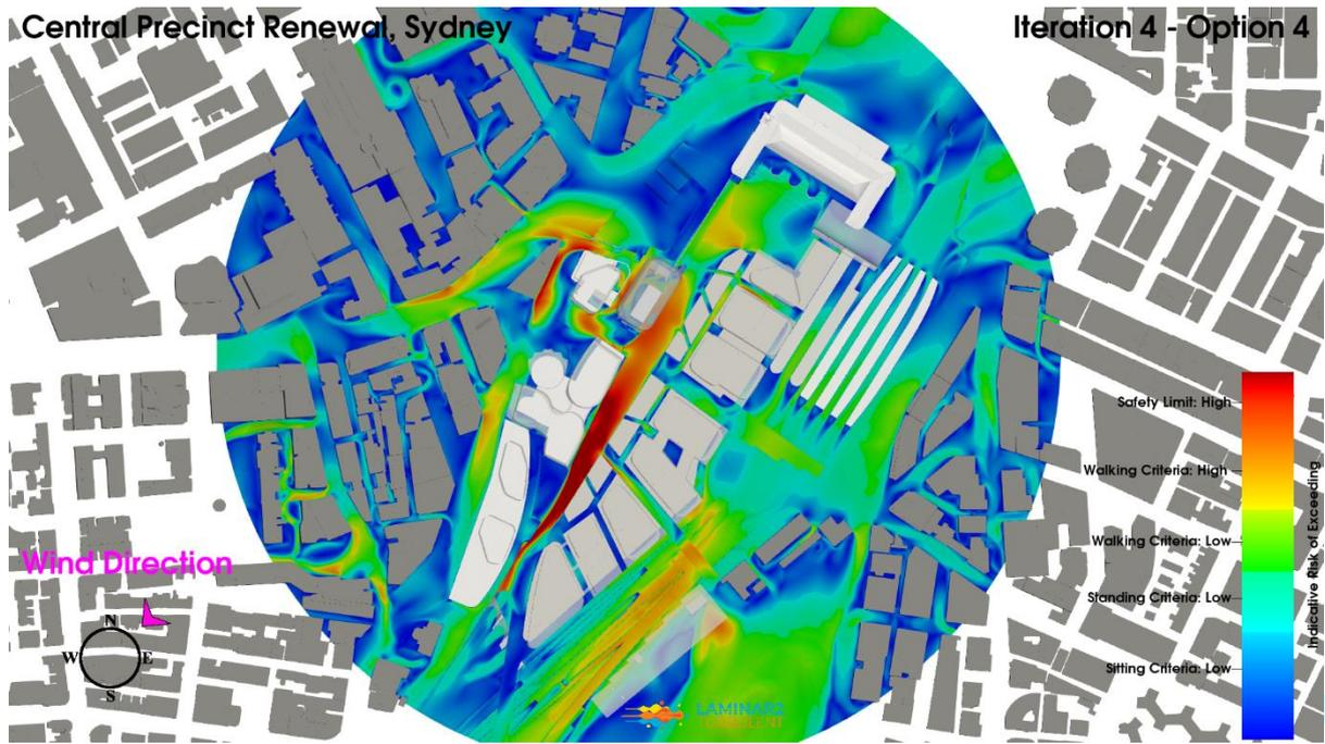
**Figure 67: Iteration 4 – Option 4 Configuration, Northeast Wind Direction, Planview, Pedestrian Level Environmental Wind Risk Contour Plot**
