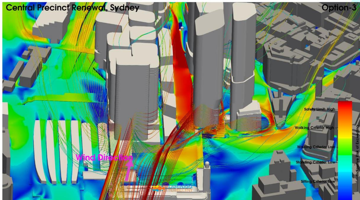
**Figure 60: Iteration 3 – Option 3 Configuration, Northeast Wind Direction, Streamlines, Pedestrian Level Environmental Wind Risk Contour Plot**
