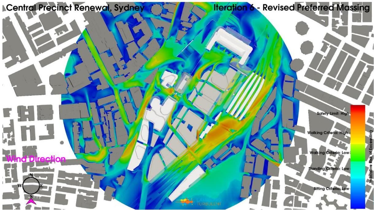
**Figure 126: Iteration 6 – Revised Preferred Massing Configuration, South Wind Direction, Planview, Pedestrian Level Environmental Wind Risk Contour Plot**
