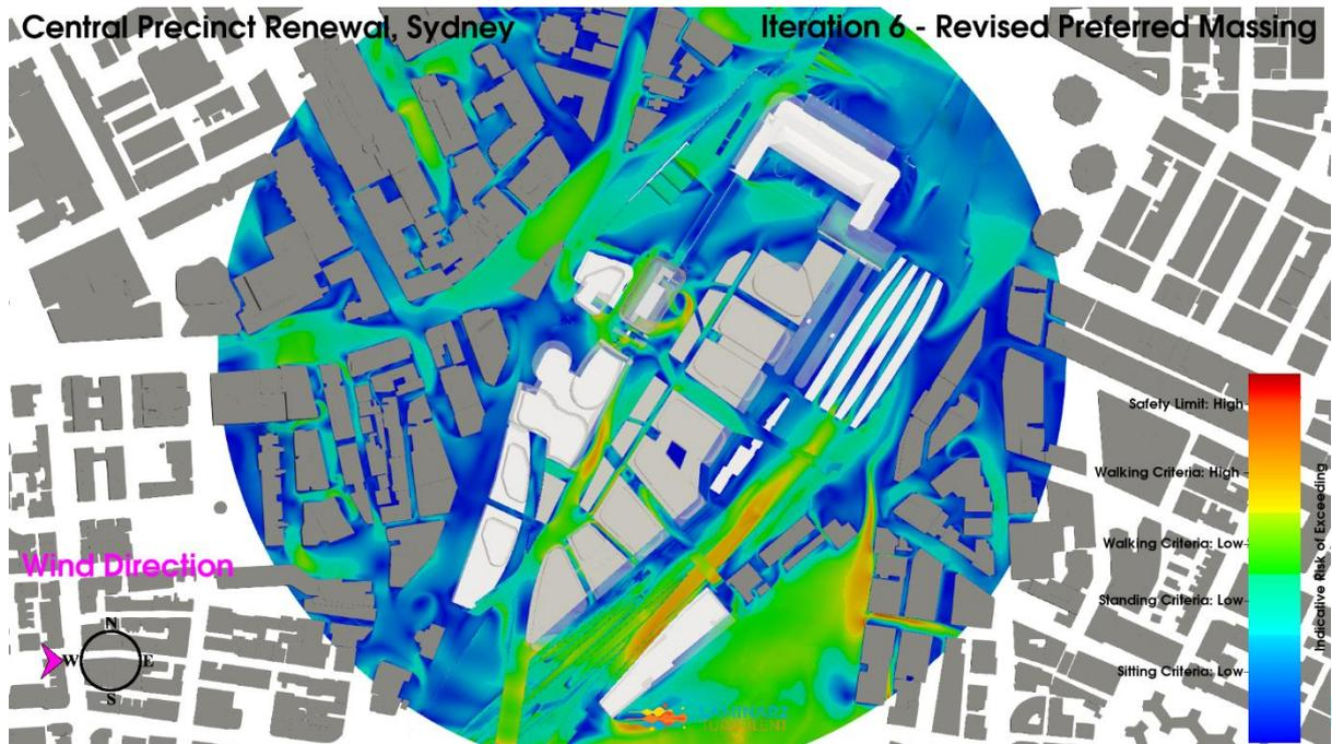
**Figure 128: Iteration 6 - Revised Preferred Massing Configuration, West Wind Direction, Planview, Pedestrian Level Environmental Wind Risk Contour Plot**
