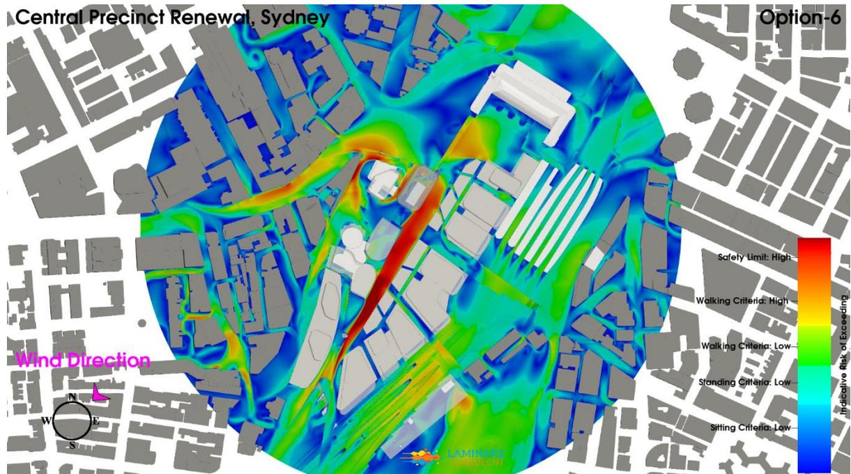
**Figure 64: Iteration 3 - Option 6 Configuration, Northeast Wind Direction, Planview, Ground Level Pedestrian Environmental Wind Risk Contour Plot**
