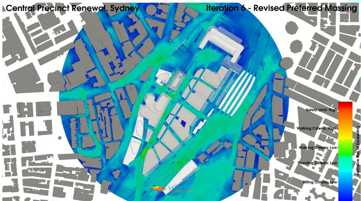
**Figure 131: Iteration 6 - Revised Preferred Massing Configuration, Combined Wind Directions, Planview, Average Pedestrian Level Environmental Wind Risk Contour Plot**
