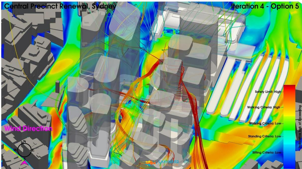
**Figure 78: Iteration 4 – Option 5 Configuration, South Wind Direction, Streamlines & Pedestrian Level Environmental Wind Risk Contour Plot**
