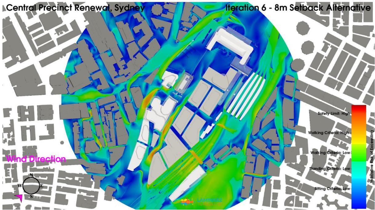
**Figure 161: Iteration 6 – 8m Setback Alternative Configuration, Southwest Wind Direction, Planview, Pedestrian Level Environmental Wind Risk Contour Plot**
