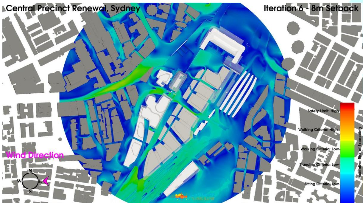
**Figure 145: Iteration 6 – 8m Setback Configuration, East Wind Direction, Planview, Pedestrian Level Environmental Wind Risk Contour Plot**
