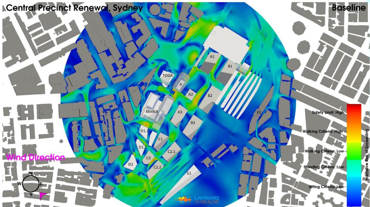
**Figure 9: Baseline Configuration, Southeast Wind Direction, Planview, Ground Level Pedestrian Environmental Wind Risk Contour Plot**
