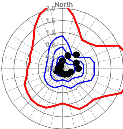
Peak velocity squared ratio  $\left| \frac{\overline{V}_{local}}{\overline{V}_{300m}} \right|^2$  as a function of wind direction
