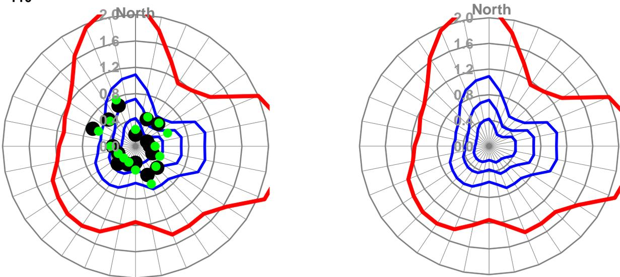
Peak velocity squared ratio  $\left| \frac{\widehat{V}_{local}}{\widehat{V}_{300m}} \right|^2$  as a function of wind direction
