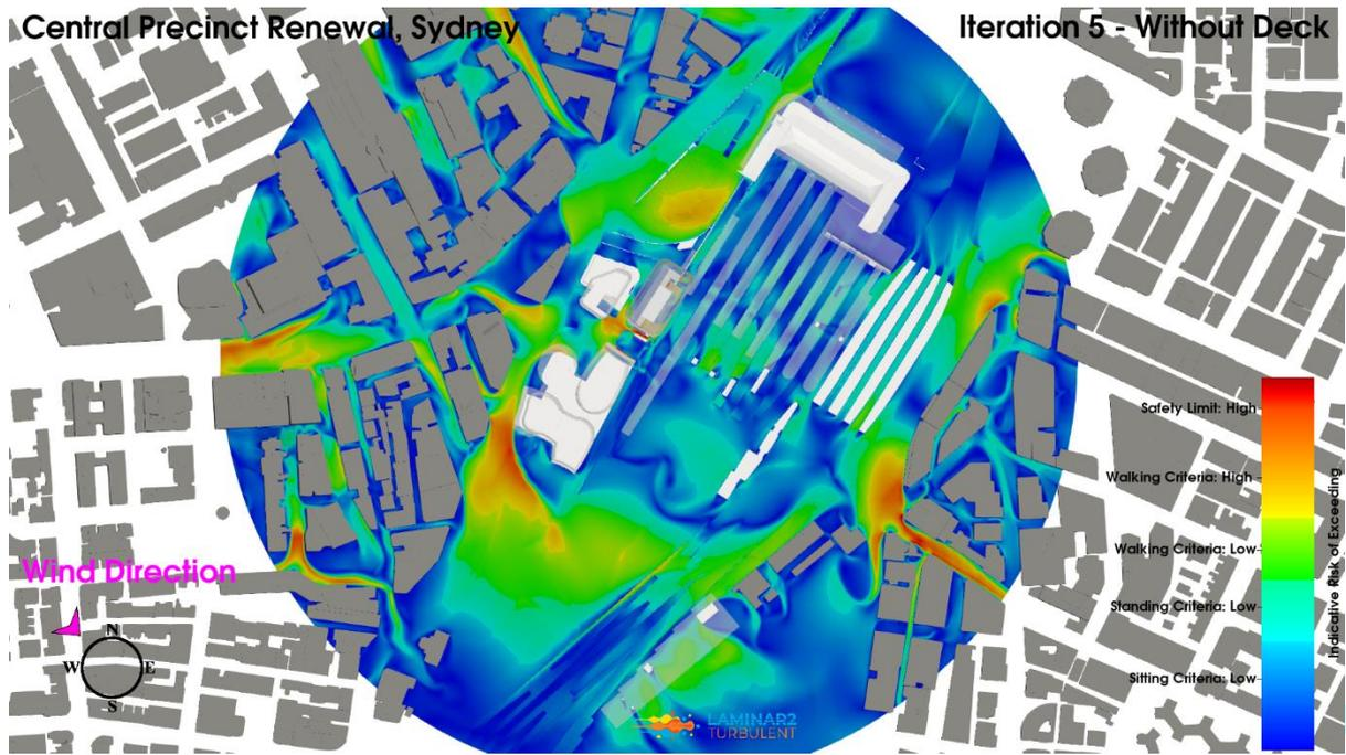
**Figure 103: Iteration 5 – Baseline Without Deck Configuration, Northwest Wind Direction, Planview, Pedestrian Level Environmental Wind Risk Contour Plot**
