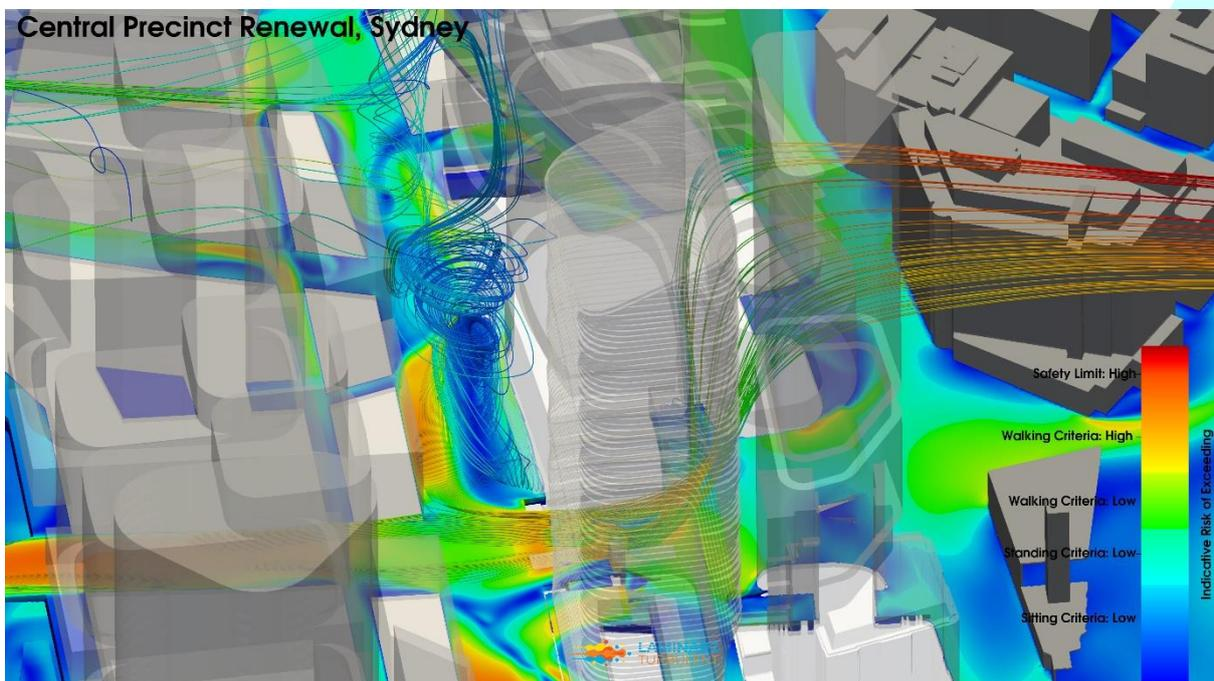
**Figure 137: Iteration 6 – Revised Preferred Massing Configuration, Northwest Wind Direction, Streamlines & Pedestrian Level Environmental Wind Risk Contour Plot**
