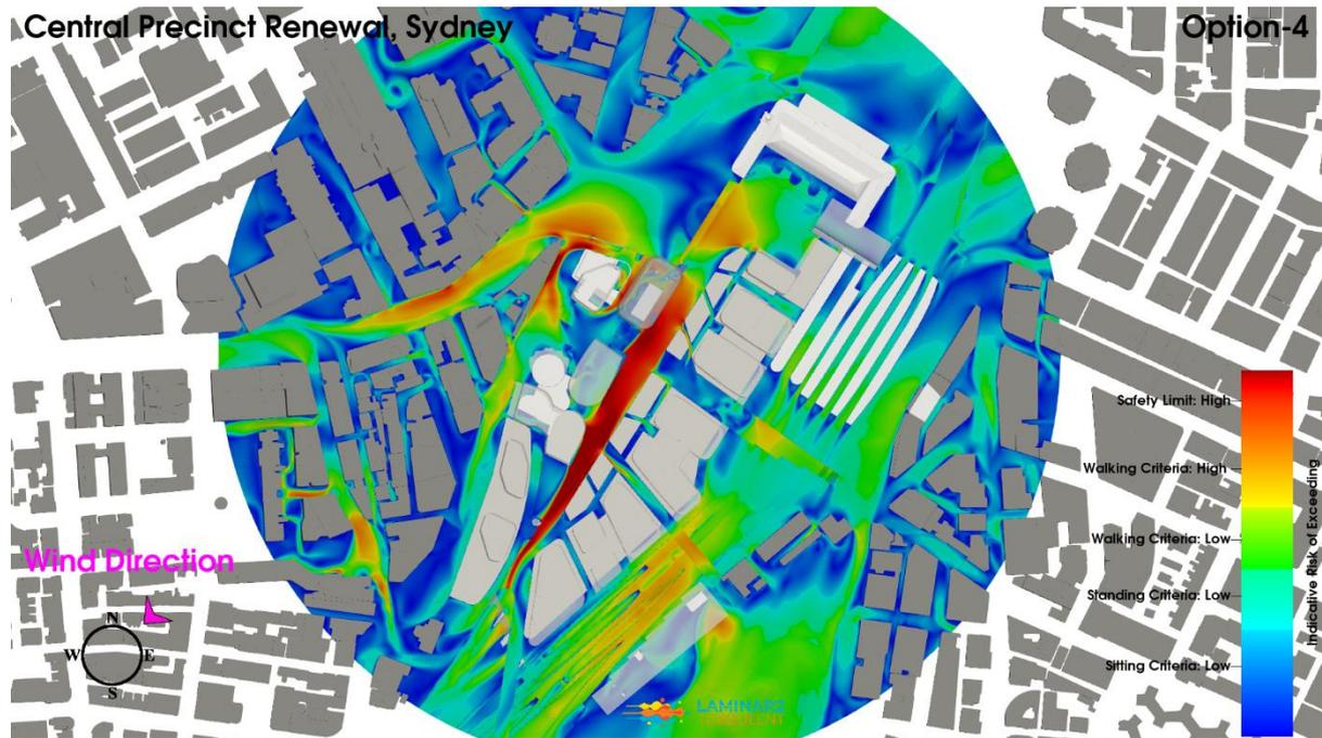
**Figure 62: Iteration 3 - Option 4 Configuration, Northeast Wind Direction, Planview, Ground Level Pedestrian Environmental Wind Risk Contour Plot**
