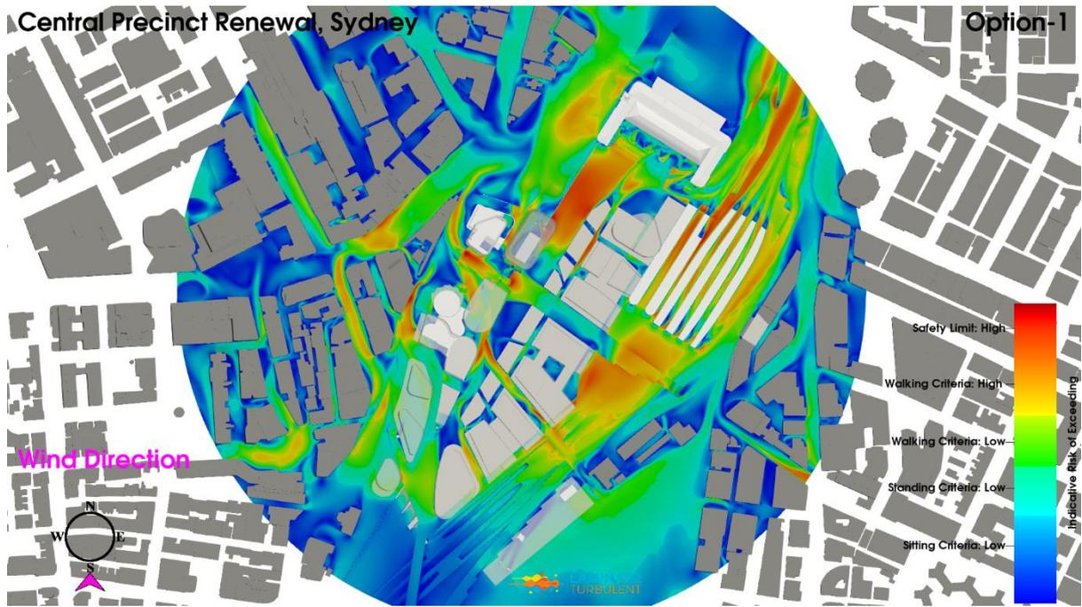
**Figure 39: Iteration 2 – Option 1 Configuration, South Wind Direction, Planview, Ground Level Pedestrian Environmental Wind Risk Contour Plot**
