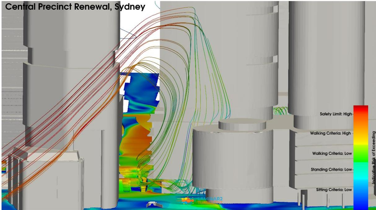
**Figure 138: Iteration 6 – Revised Preferred Massing Configuration, Northwest Wind Direction, Streamlines & Pedestrian Level Environmental Wind Risk Contour Plot**
