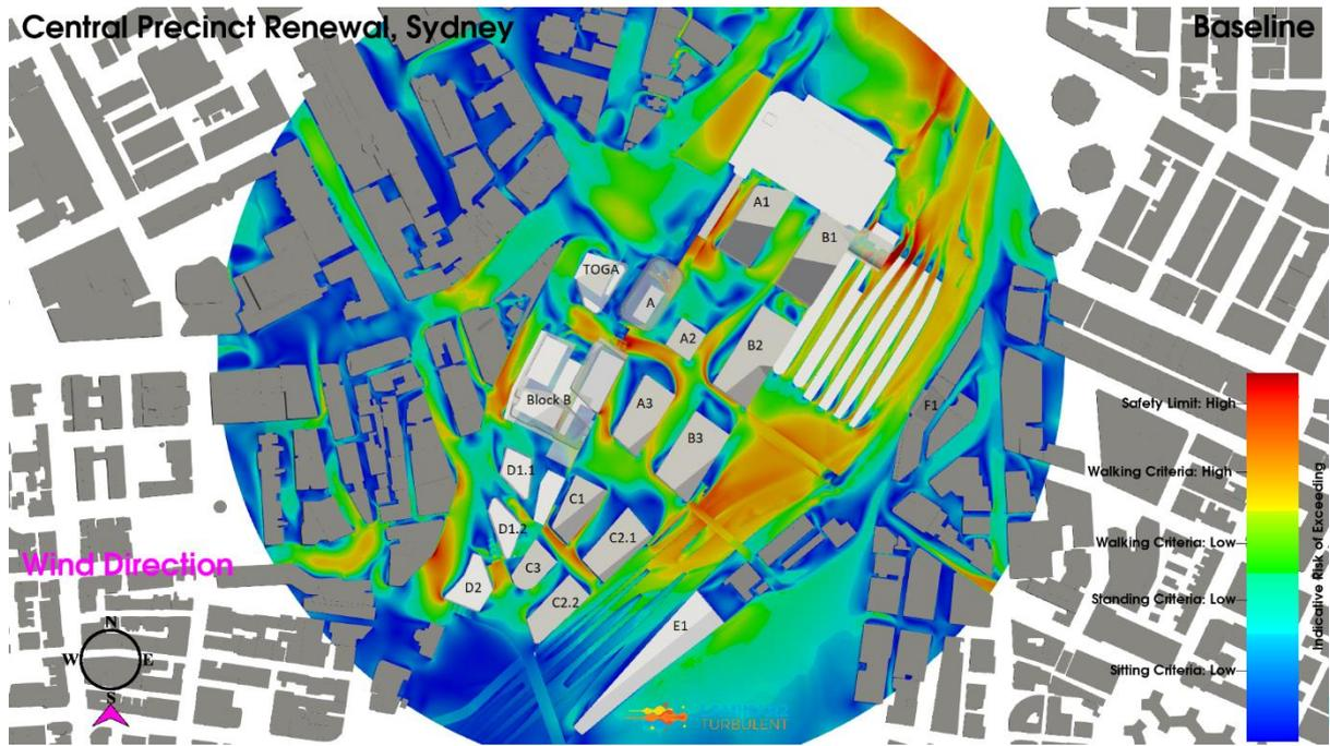
**Figure 10: Baseline Configuration, South Wind Direction, Planview, Ground Level Pedestrian Environmental Wind Risk Contour Plot**
