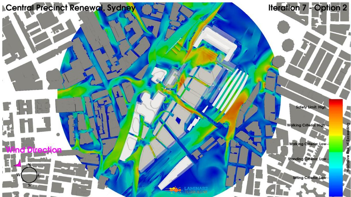
**Figure 185: Iteration 7 Option 2, Northwest Wind Direction, Planview, Pedestrian Level Environmental Wind Risk Contour Plot**
