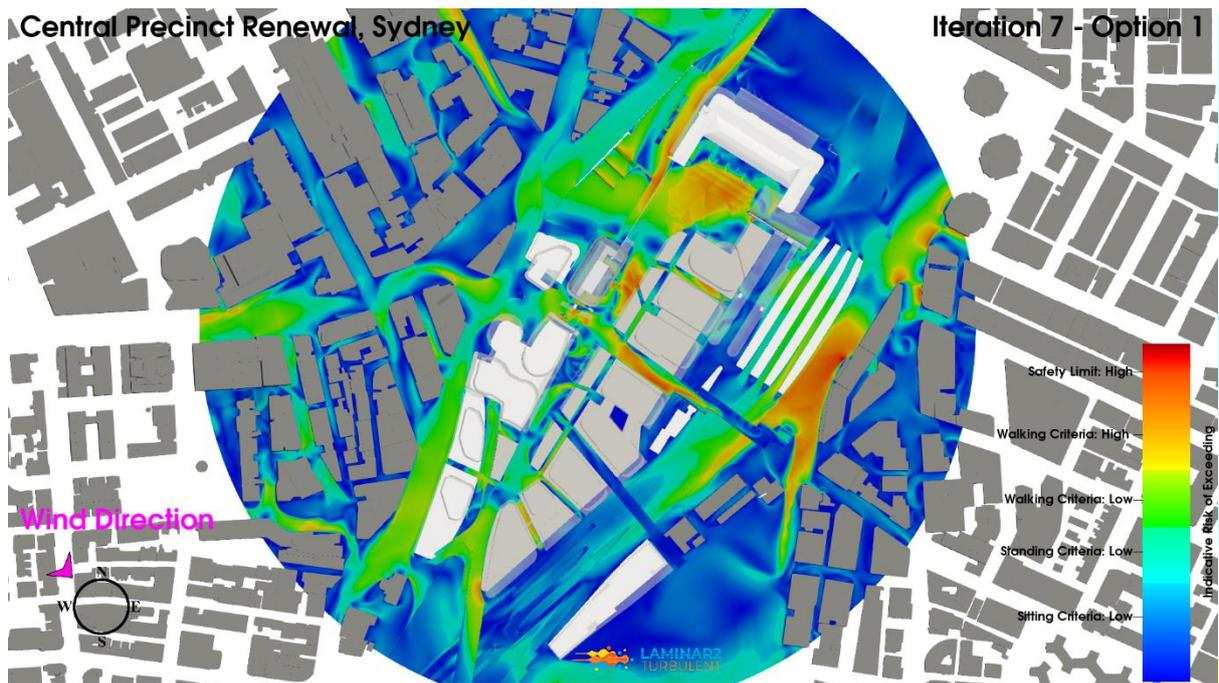
**Figure 183: Iteration 7 Option 1, Northwest Wind Direction, Planview, Pedestrian Level Environmental Wind Risk Contour Plot**
