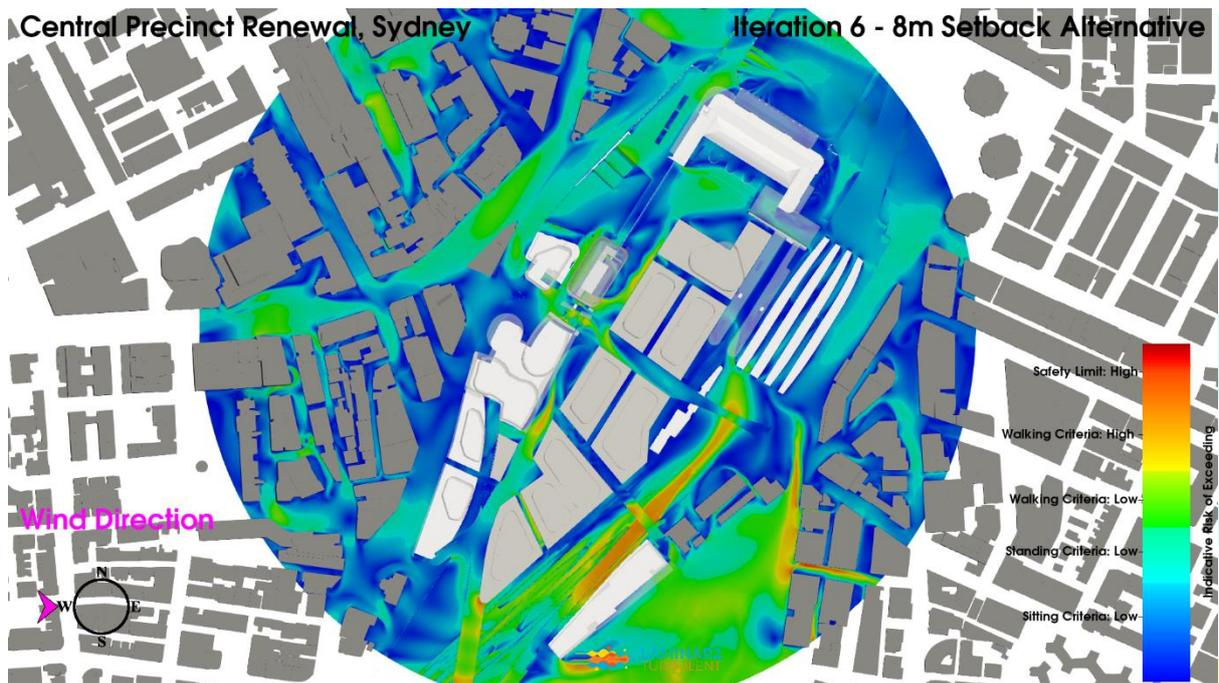
**Figure 162: Iteration 6 – 8m Setback Alternative Configuration, West Wind Direction, Planview, Pedestrian Level Environmental Wind Risk Contour Plot**
