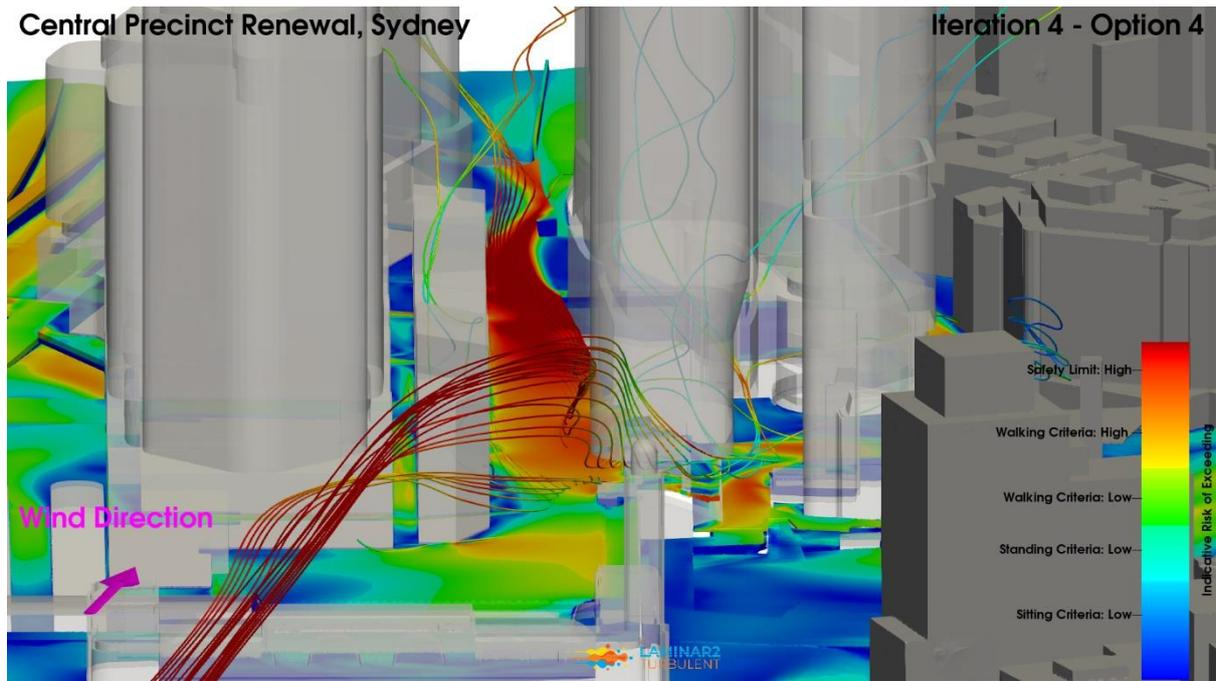
**Figure 71: Iteration 4 – Option 4 Configuration, Northeast Wind Direction, Streamlines & Pedestrian Level Environmental Wind Risk Contour Plot**
