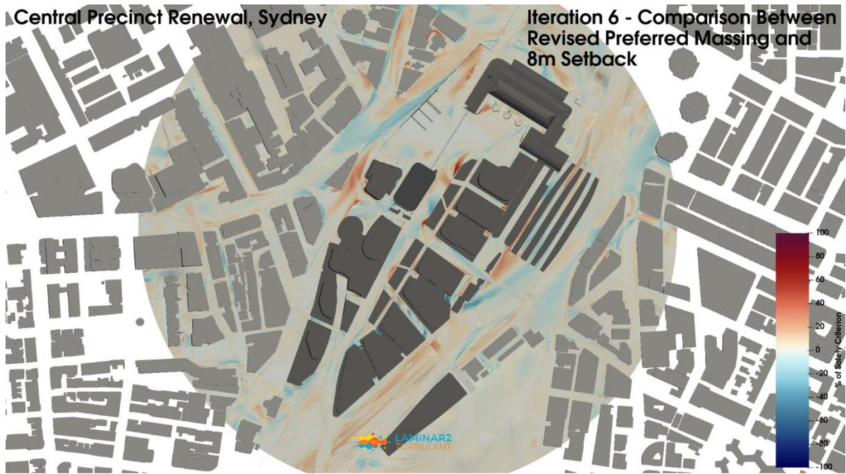
**Figure 167: Comparison of Maximum Pedestrian Level Environmental Wind Risk between Iteration 6 - Revised Preferred Massing and Iteration 6 - 8m Setback, Planview.**
