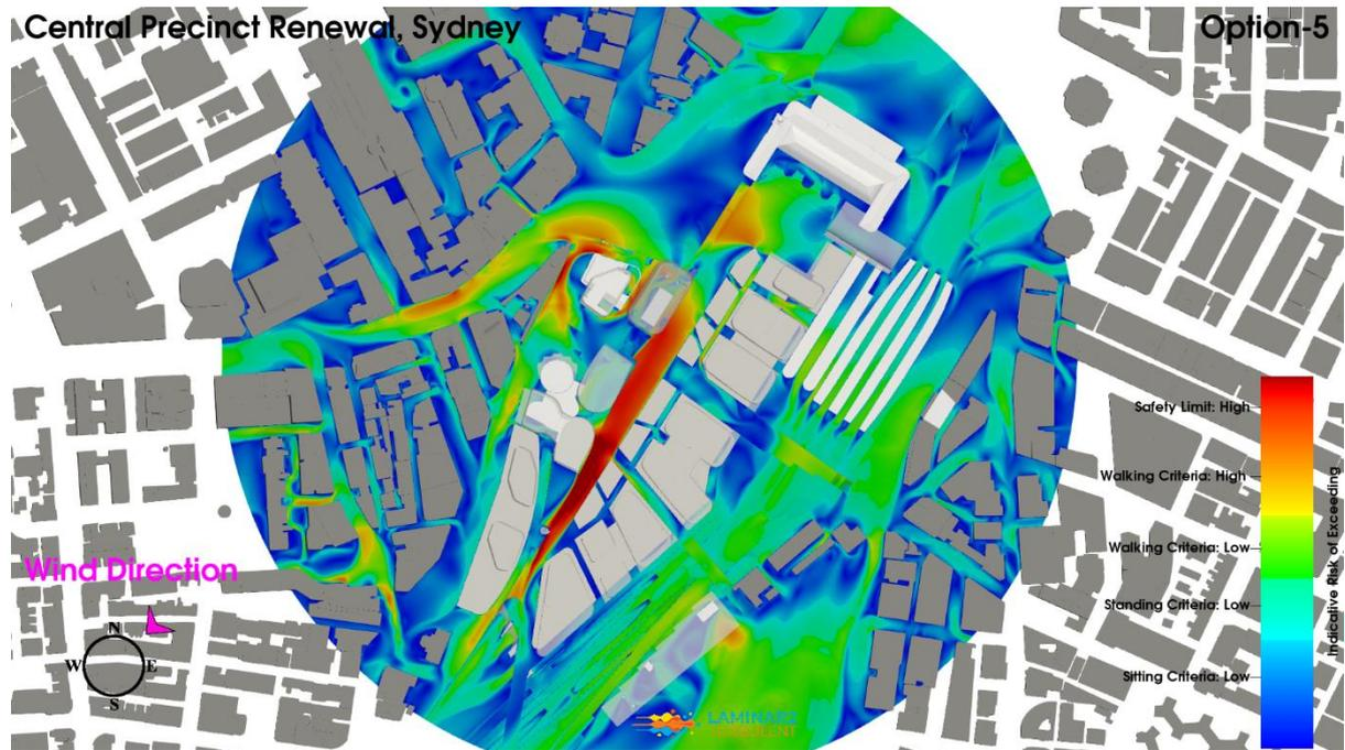
**Figure 63: Iteration 3 – Option 5 Configuration, Northeast Wind Direction, Planview, Ground Level Pedestrian Environmental Wind Risk Contour Plot**
