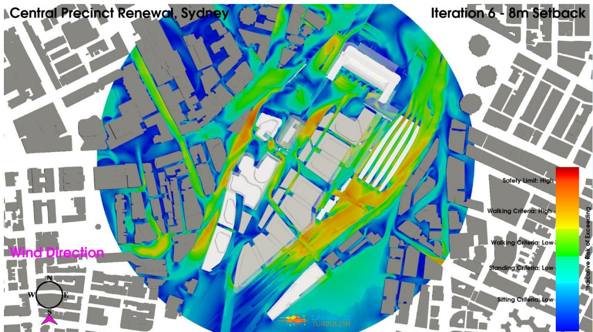
**Figure 147: Iteration 6 – 8m Setback Configuration, South Wind Direction, Planview, Pedestrian Level Environmental Wind Risk Contour Plot**
