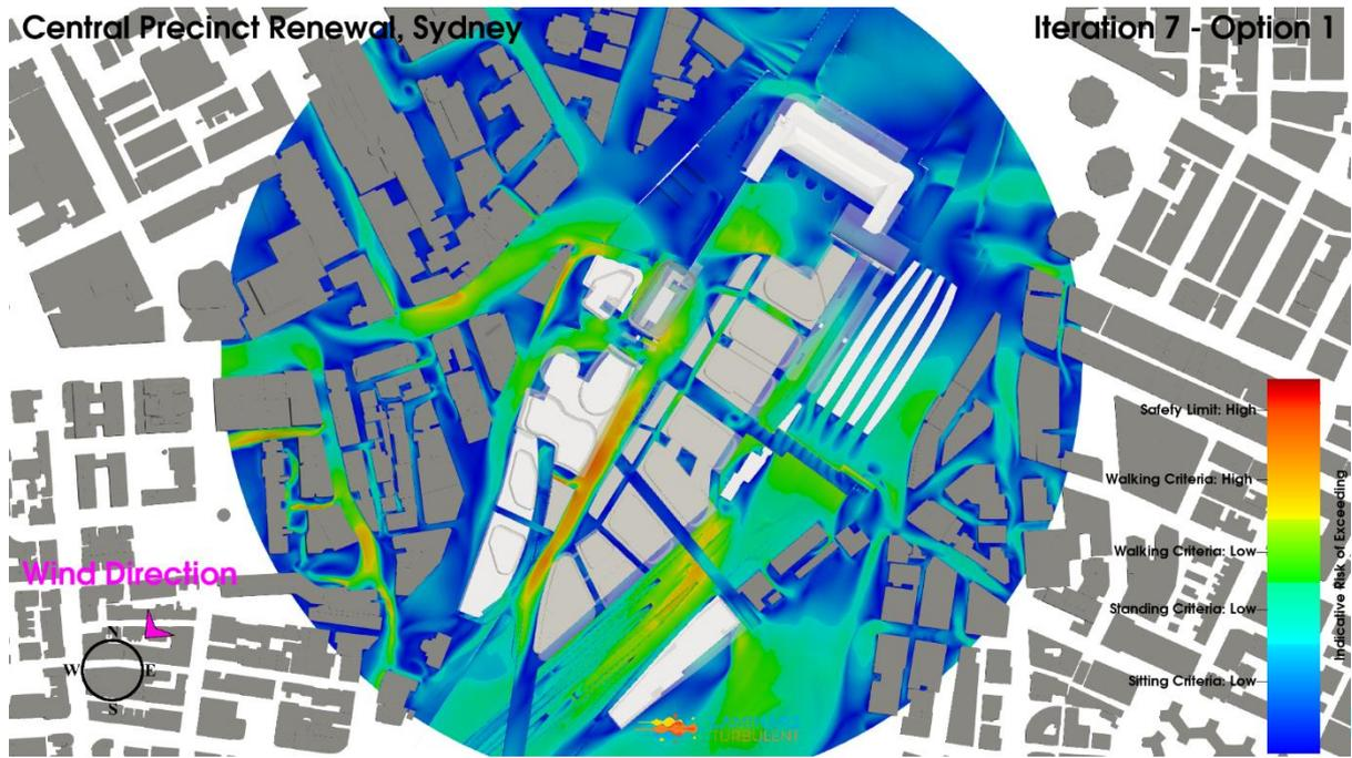
**Figure 182: Iteration 7 Option 1, Northeast Wind Direction, Planview, Pedestrian Level Environmental Wind Risk Contour Plot**
