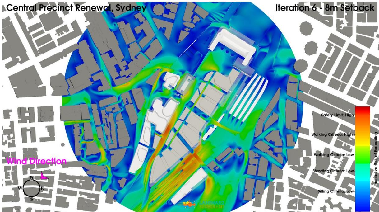
**Figure 144: Iteration 6 – 8m Setback Configuration, Northeast Wind Direction, Planview, Pedestrian Level Environmental Wind Risk Contour Plot**
