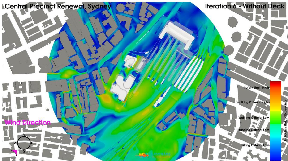
**Figure 113: Iteration 6 – Without Deck Configuration, Southwest Wind Direction, Planview, Pedestrian Level Environmental Wind Risk Contour Plot**
