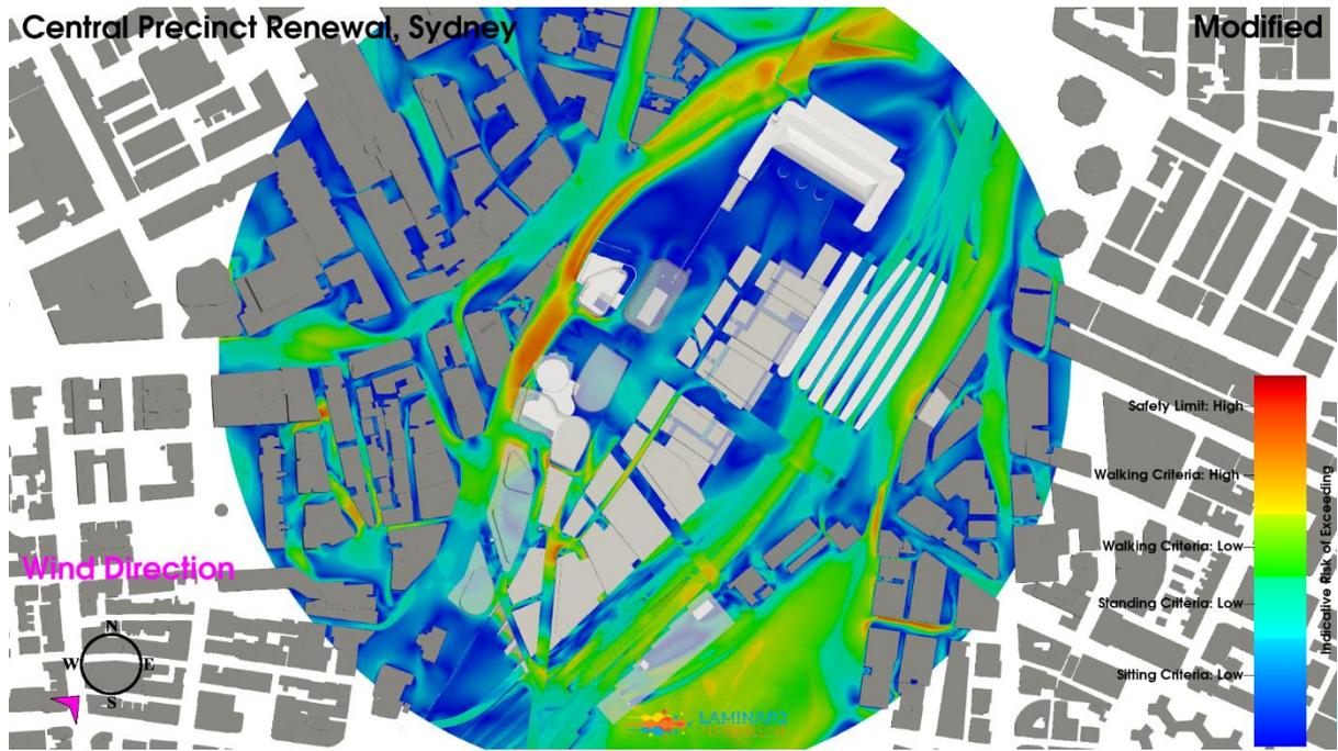
**Figure 28: Iteration 1 Configuration, Southwest Wind Direction, Planview, Ground Level Pedestrian Environmental Wind Risk Contour Plot**
