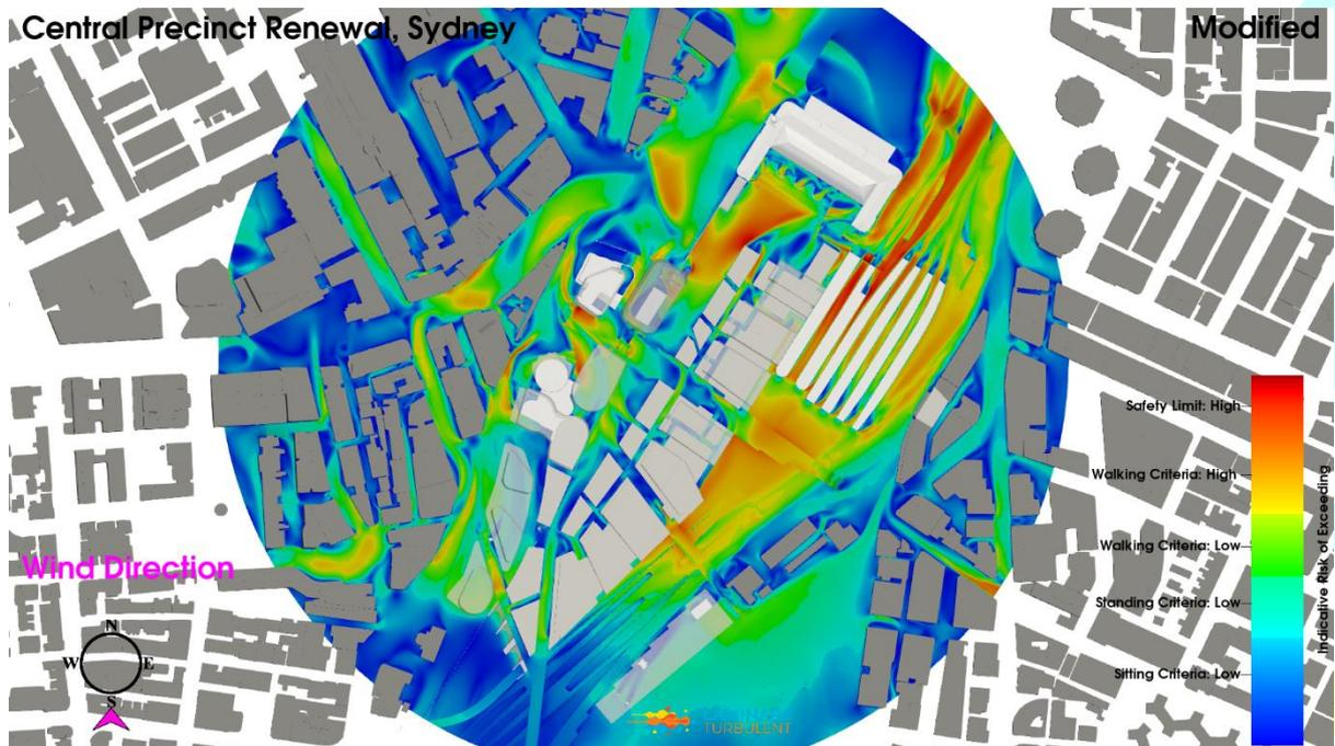
**Figure 27: Iteration 1 Configuration, South Wind Direction, Planview, Ground Level Pedestrian Environmental Wind Risk Contour Plot**
