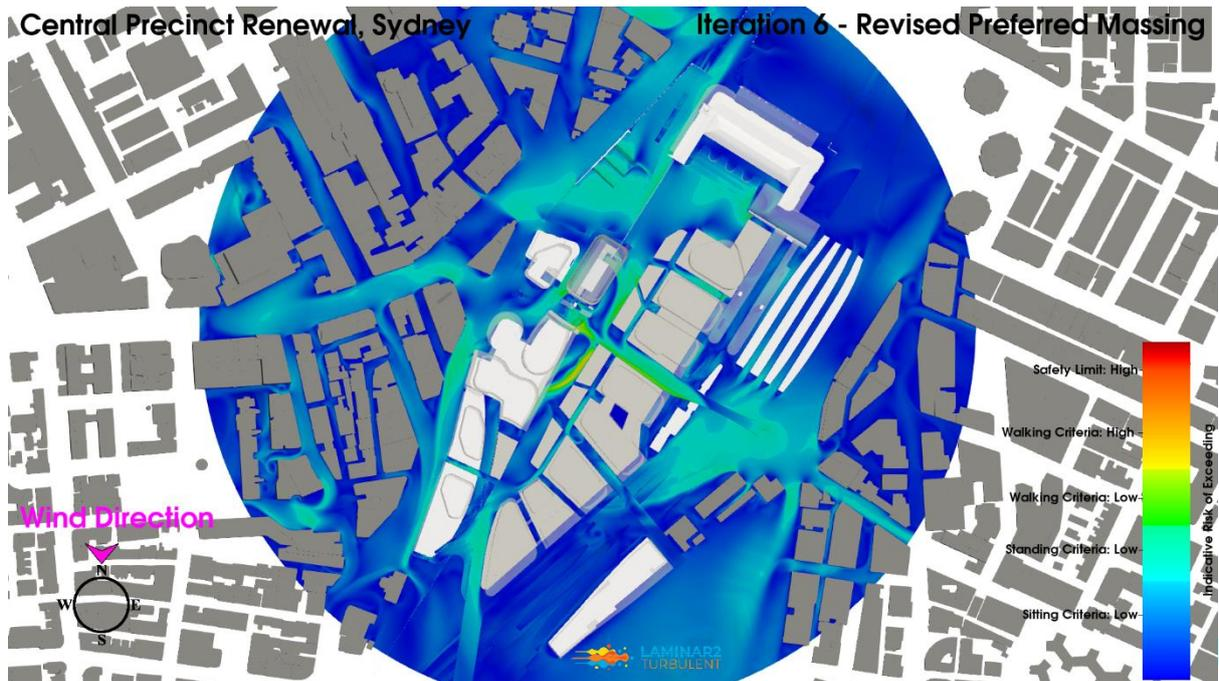
**Figure 120: Iteration 6 – Revised Preferred Massing Configuration, North Wind Direction, Planview, Pedestrian Level Environmental Wind Risk Contour Plot**
