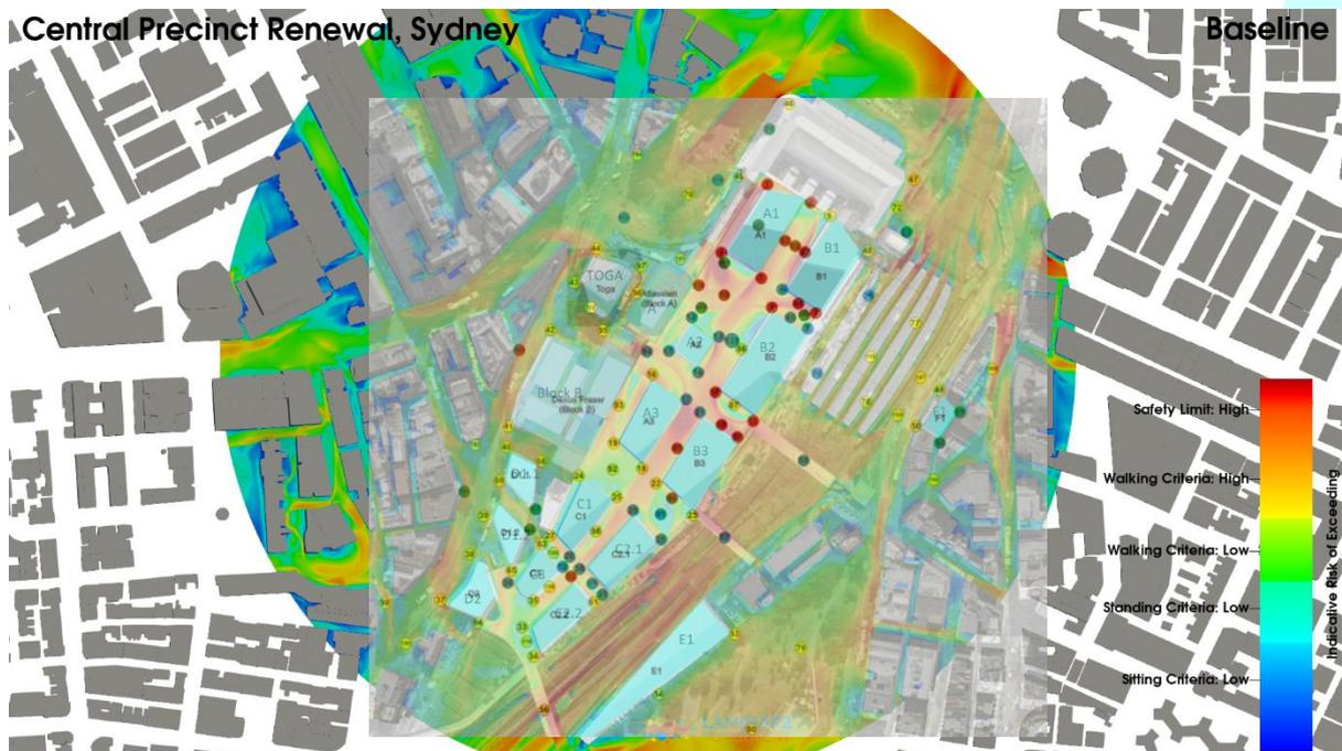
**Figure 19: Comparison Between Baseline CFD and Wind Tunnel Results, Combined Wind Directions, Planview, Ground Level Maximum Pedestrian Environmental Wind Risk Contour Plot**
