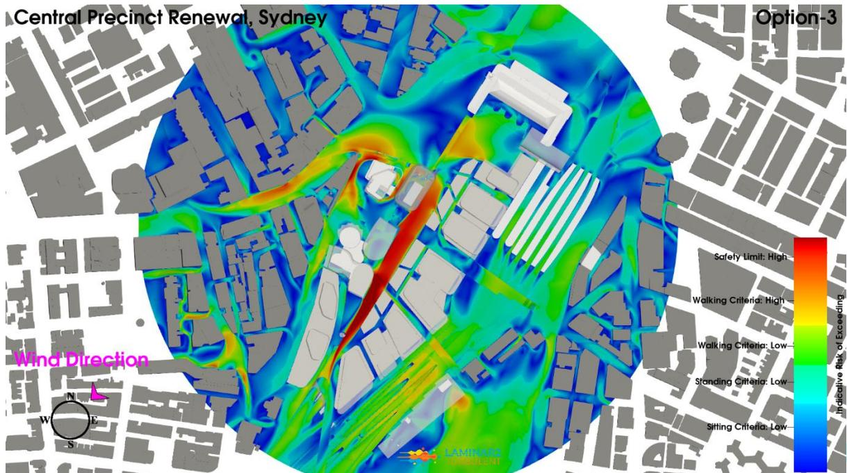
**Figure 57: Iteration 3 – Option 3 Configuration, Northeast Wind Direction, Planview, Ground Level Pedestrian Environmental Wind Risk Contour Plot**
