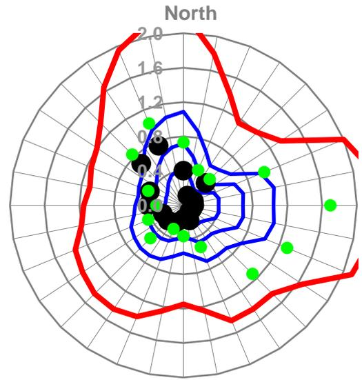
Peak velocity squared ratio  $\left| \frac{\hat{V}_{local}}{\hat{V}_{300m}} \right|^2$  as a function of wind direction
