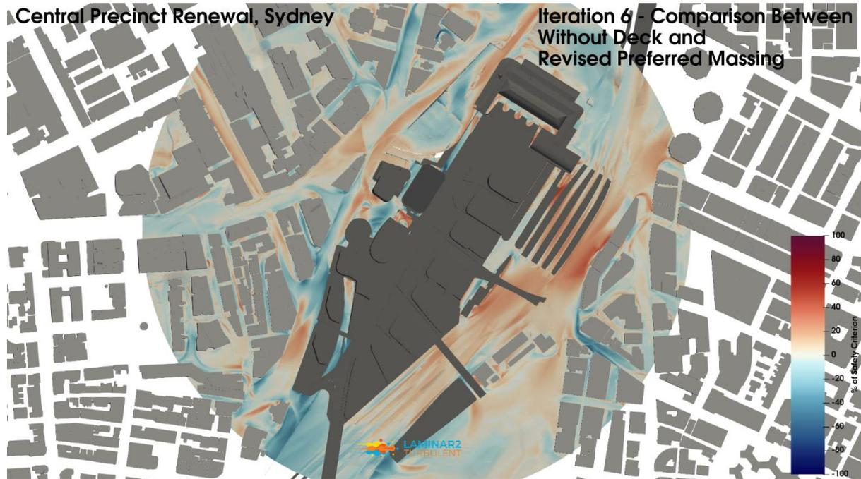
**Figure 166: Comparison of Maximum Pedestrian Level Environmental Wind Risk between Iteration 6 – Baseline Without Deck and Iteration 6 – Revised Preferred Massing, Planview.**
