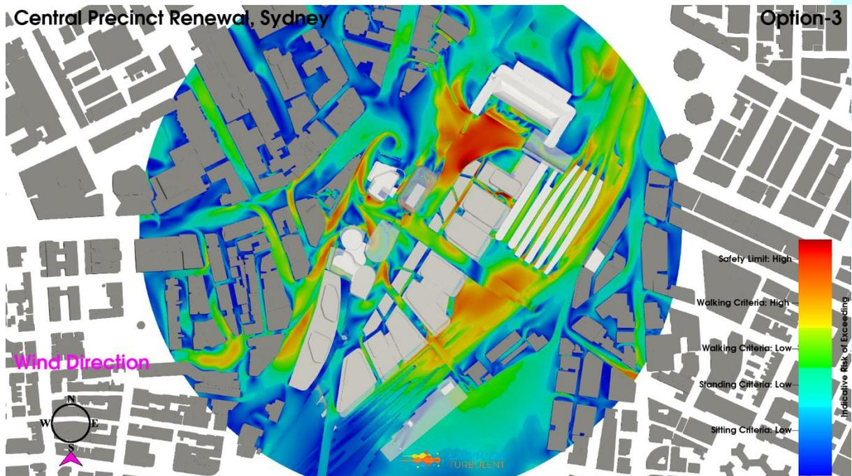
**Figure 58: Iteration 3 – Option 3 Configuration, South Wind Direction, Planview, Ground Level Pedestrian Environmental Wind Risk Contour Plot**
