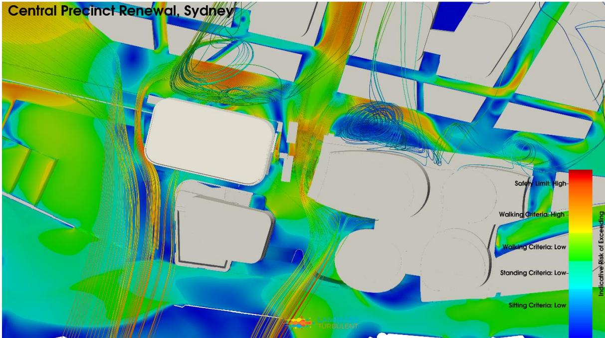
**Figure 132: Iteration 6 – Revised Preferred Massing Configuration, Northwest Wind Direction, Streamlines & Pedestrian Level Environmental Wind Risk Contour Plot**
