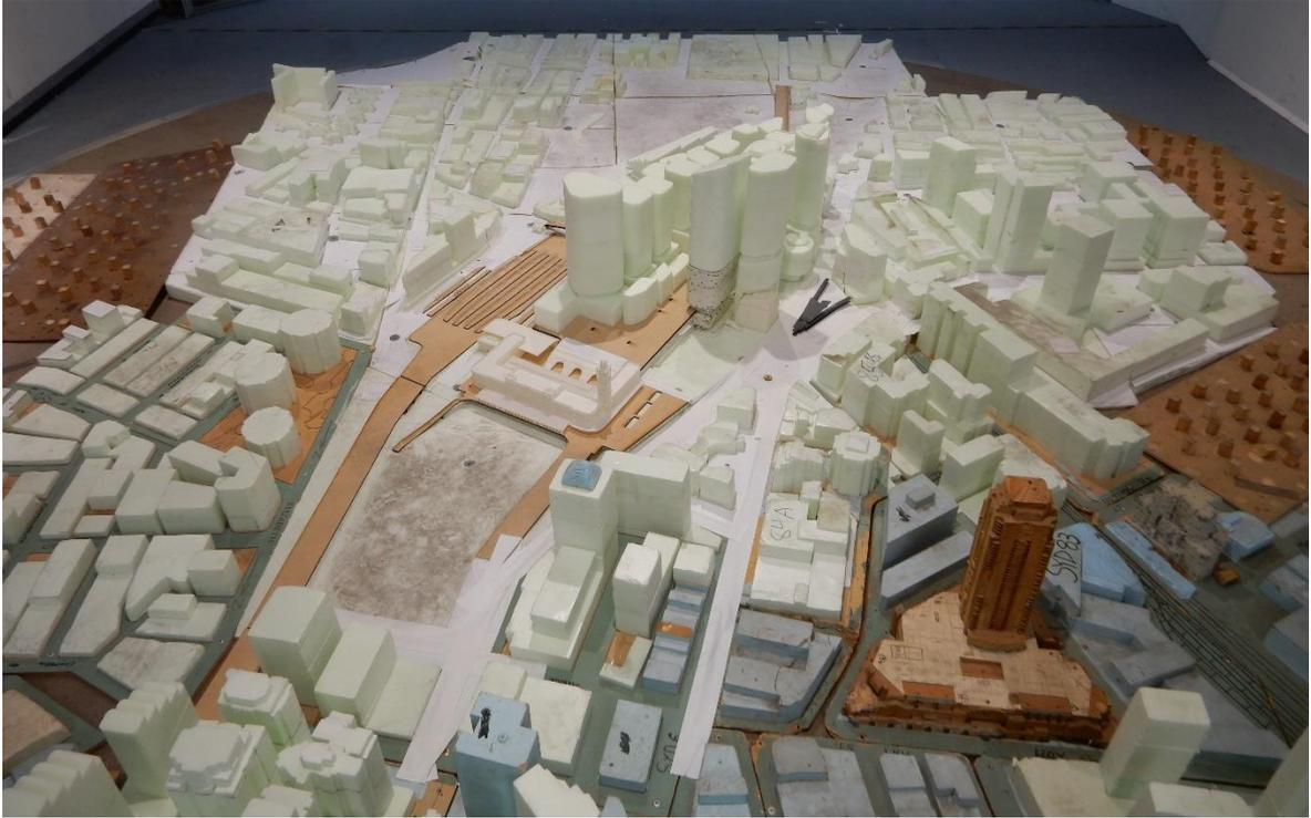
**Figure 3a – View from the north of the 1/400 scale model of the Central Precinct Renewal Masterplan – Configuration April 2022 in the wind tunnel.**
