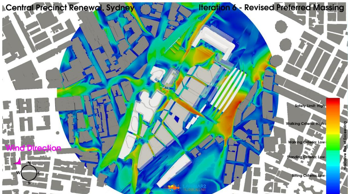
**Figure 129: Iteration 6 - Revised Preferred Massing Configuration, Northwest Wind Direction, Planview, Pedestrian Level Environmental Wind Risk Contour Plot**
