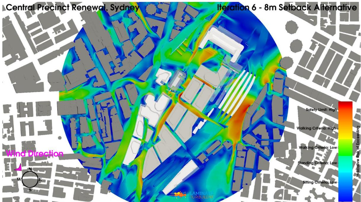
**Figure 163: Iteration 6 – 8m Setback Alternative Configuration, Northwest Wind Direction, Planview, Pedestrian Level Environmental Wind Risk Contour Plot**
