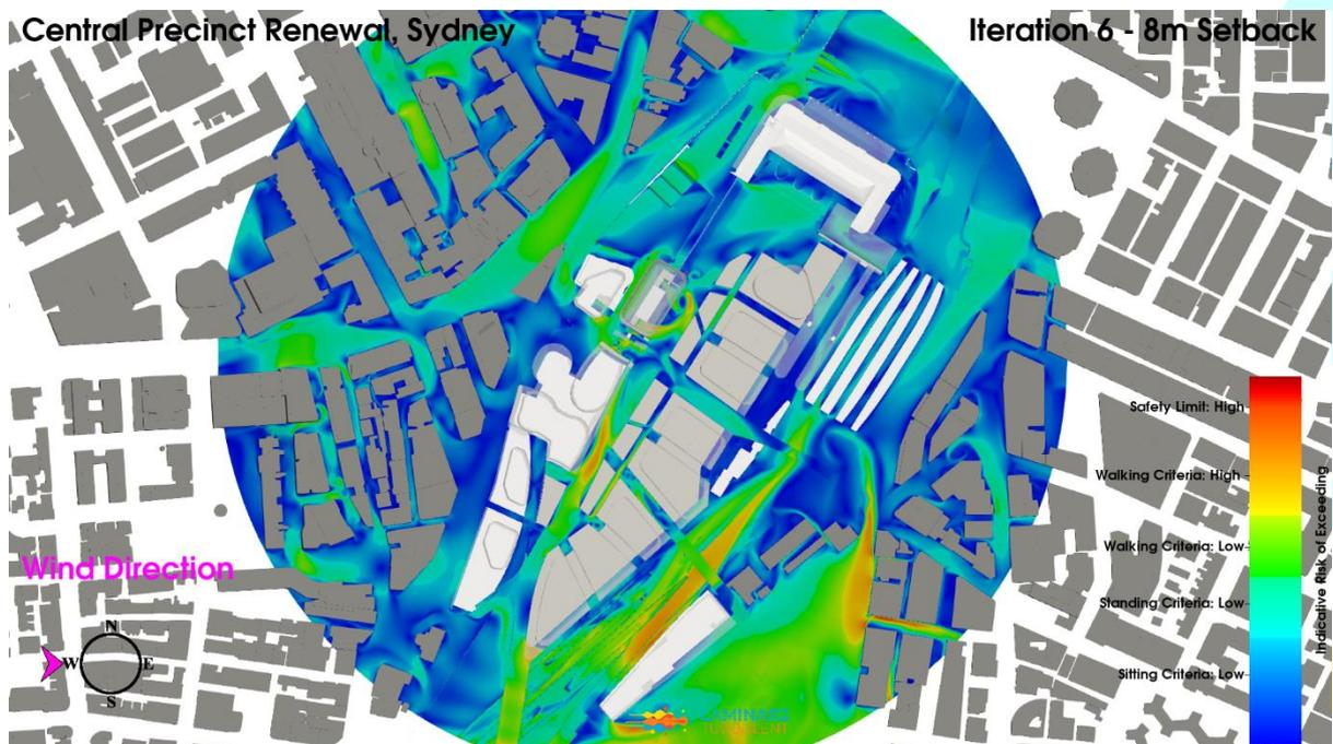
**Figure 149: Iteration 6 – 8m Setback Configuration, West Wind Direction, Planview, Pedestrian Level Environmental Wind Risk Contour Plot**
