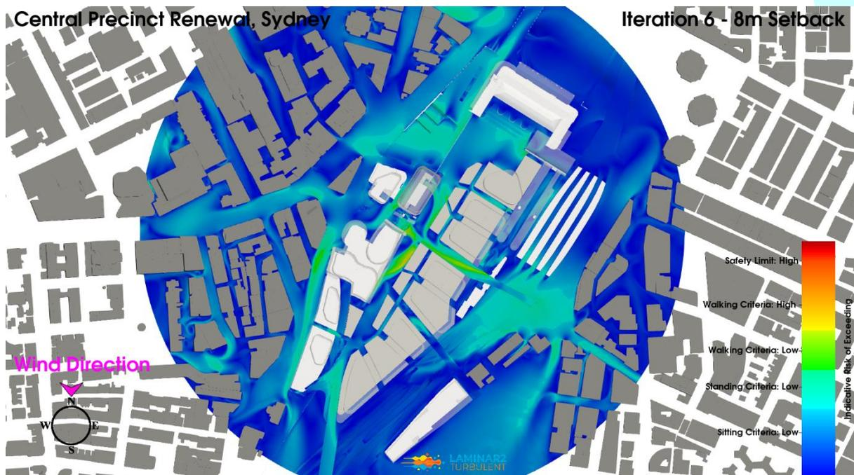
**Figure 143: Iteration 6 – 8m Setback Configuration, North Wind Direction, Planview, Pedestrian Level Environmental Wind Risk Contour Plot**
