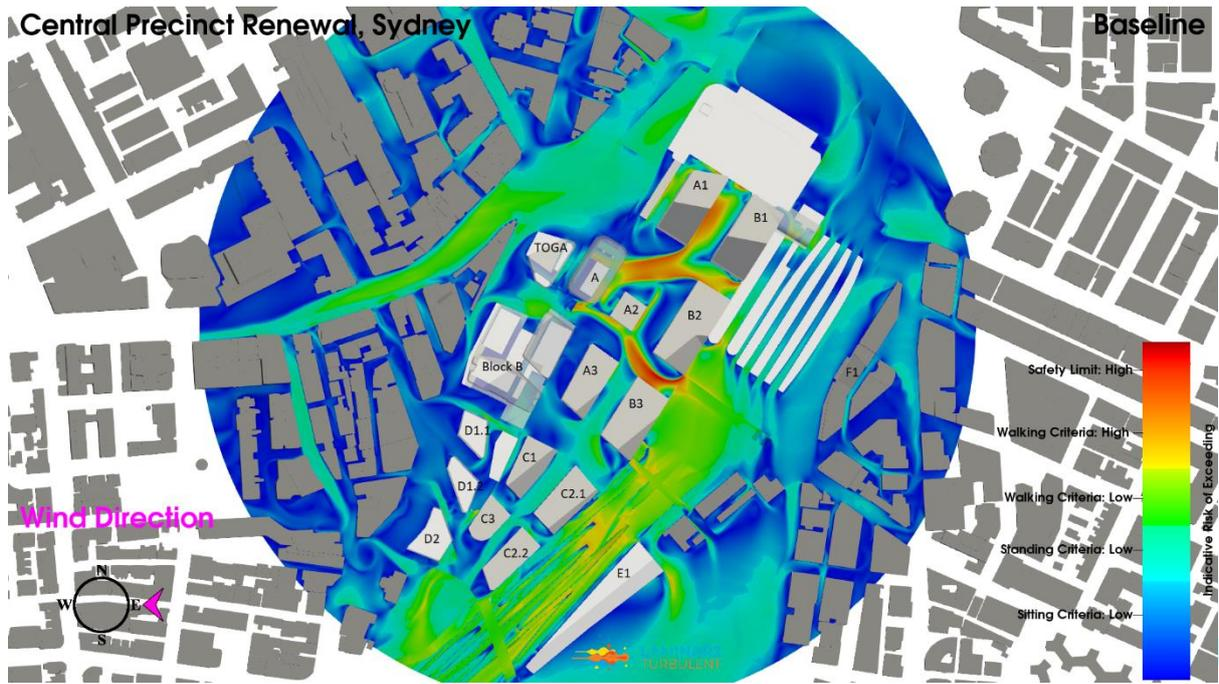
**Figure 8: Baseline Configuration, East Wind Direction, Planview, Ground Level Pedestrian Environmental Wind Risk Contour Plot**
