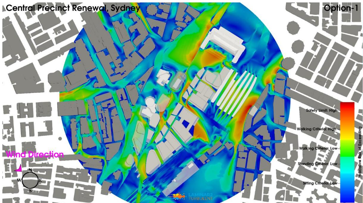
**Figure 40: Iteration 2 – Option 1 Configuration, Northwest Wind Direction, Planview, Ground Level Pedestrian Environmental Wind Risk Contour Plot**
