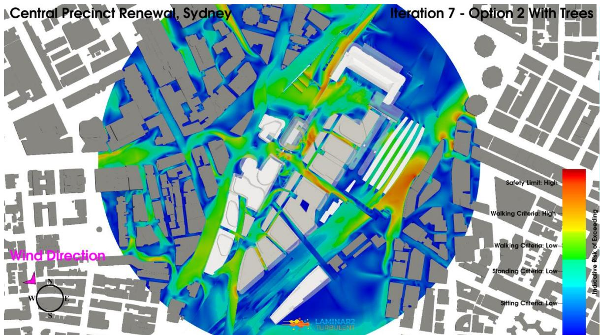
**Figure 187: Iteration 7 Option 2 With Trees, Northwest Wind Direction, Planview, Pedestrian Level Environmental Wind Risk Contour Plot**
