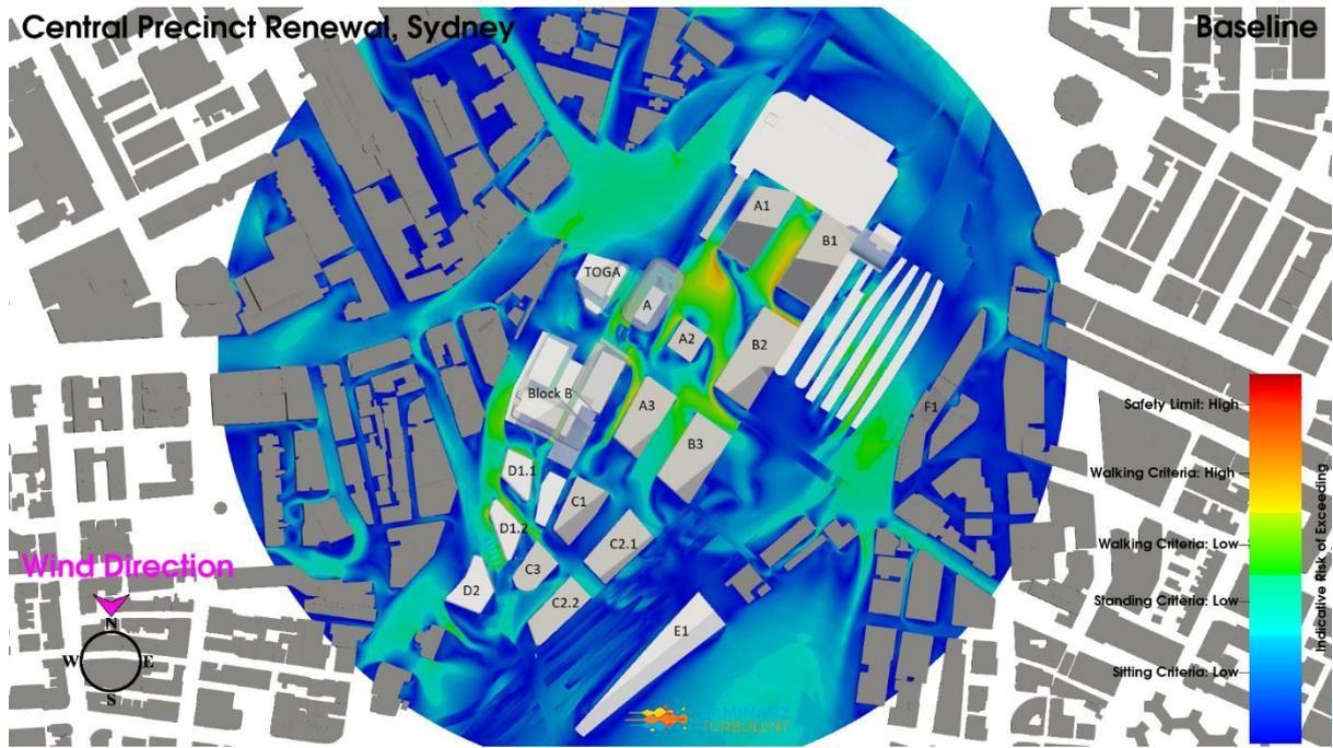
**Figure 6: Baseline Configuration, North Wind Direction, Planview, Ground Level Pedestrian Environmental Wind Risk Contour Plot**
