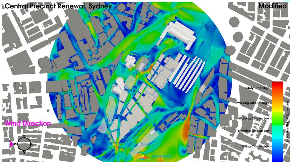
**Figure 29: Iteration 1 Configuration, West Wind Direction, Planview, Ground Level Pedestrian Environmental Wind Risk Contour Plot**
