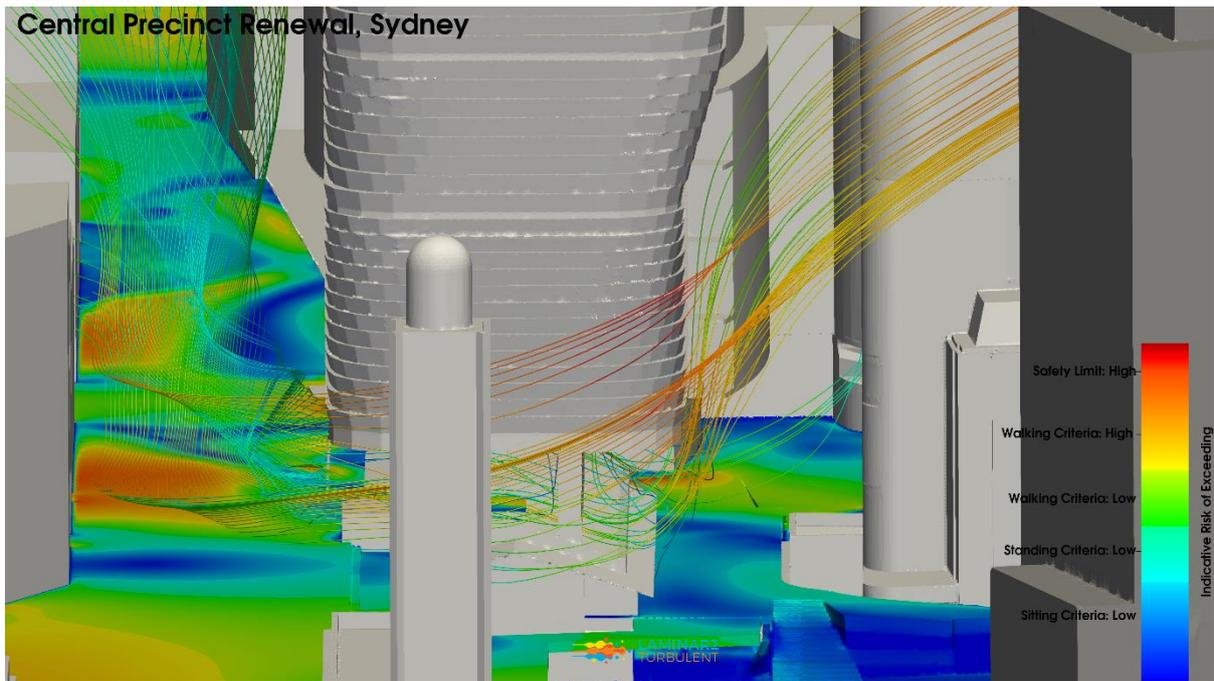
**Figure 134: Iteration 6 – Revised Preferred Massing Configuration, Northwest Wind Direction, Streamlines & Pedestrian Level Environmental Wind Risk Contour Plot**
