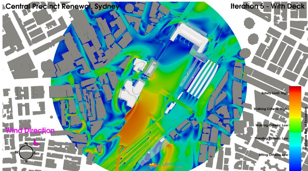
**Figure 96: Iteration 5 - Baseline With Deck Configuration, Northeast Wind Direction, Planview, Pedestrian Level Environmental Wind Risk Contour Plot**
