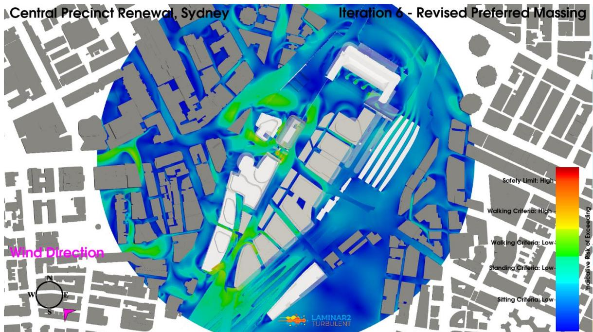
**Figure 125: Iteration 6 – Revised Preferred Massing Configuration, Southeast Wind Direction, Planview, Pedestrian Level Environmental Wind Risk Contour Plot**
