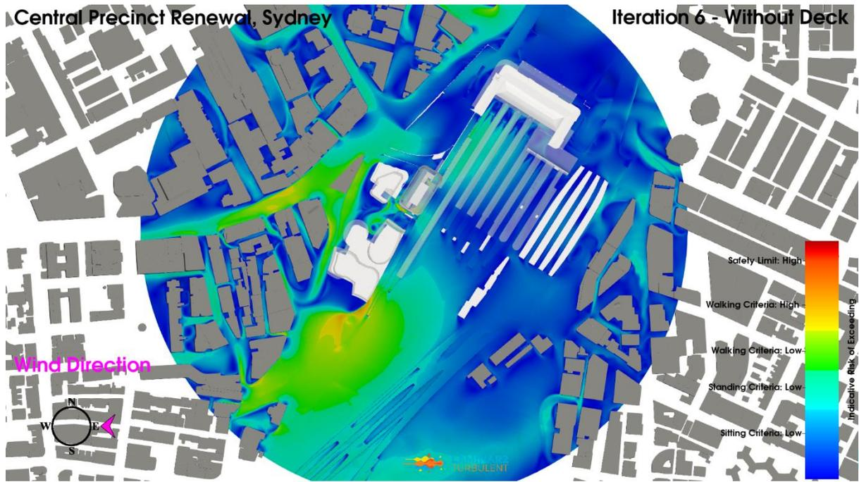
**Figure 110: Iteration 6 – Without Deck Configuration, East Wind Direction, Planview, Pedestrian Level Environmental Wind Risk Contour Plot**
