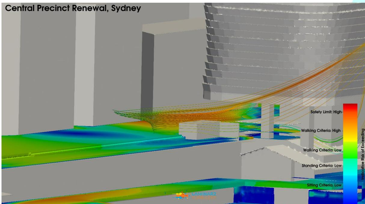
**Figure 135: Iteration 6 – Revised Preferred Massing Configuration, Northwest Wind Direction, Streamlines & Pedestrian Level Environmental Wind Risk Contour Plot**
