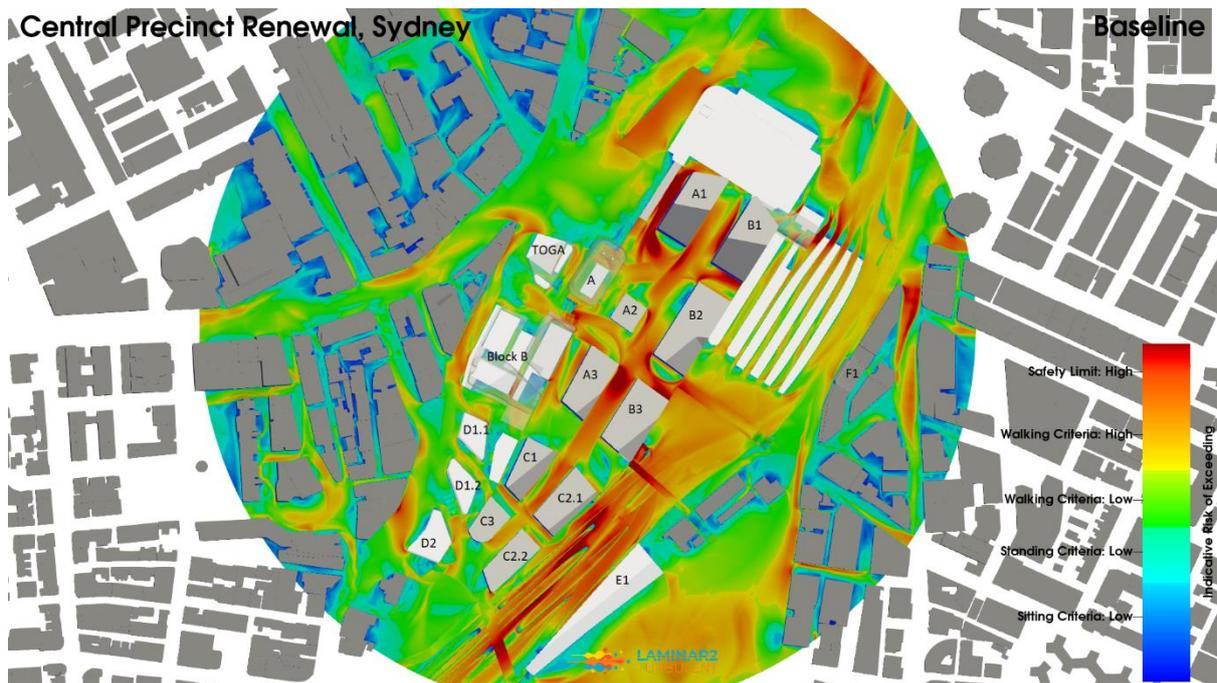
**Figure 17: Baseline Configuration, Combined Wind Directions, Planview, Ground Level Maximum Pedestrian Environmental Wind Risk Contour Plot**
