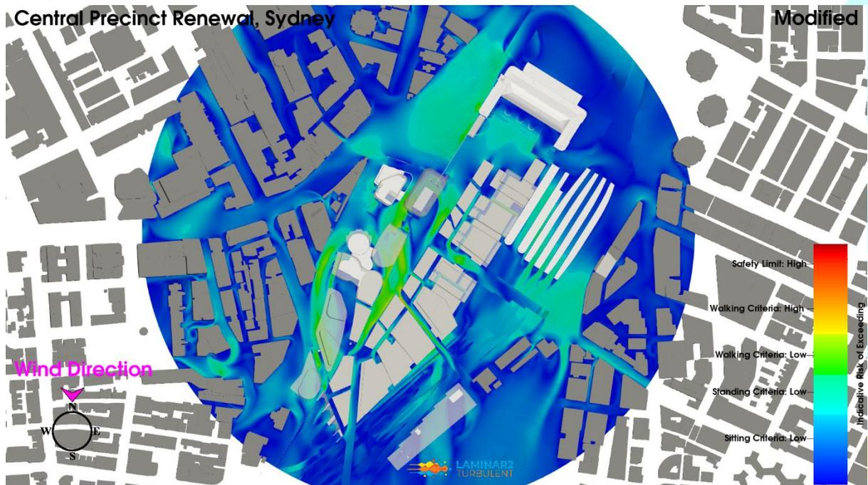
**Figure 23: Iteration 1 Configuration, North Wind Direction, Planview, Ground Level Pedestrian Environmental Wind Risk Contour Plot**
