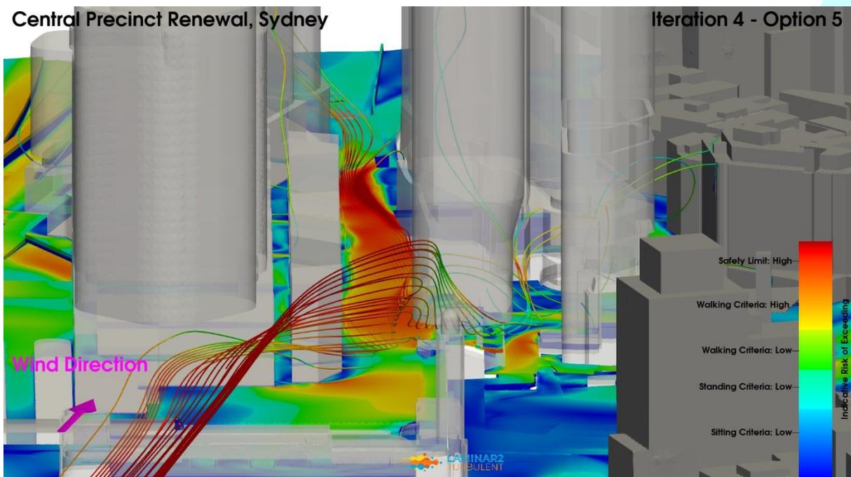
**Figure 79: Iteration 4 – Option 5 Configuration, Northeast Wind Direction, Streamlines & Pedestrian Level Environmental Wind Risk Contour Plot**
