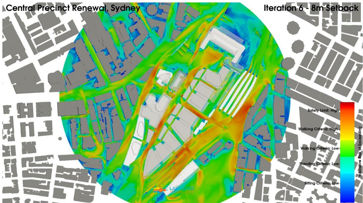
**Figure 151: Iteration 6 – 8m Setback Configuration, Combined Wind Directions, Planview, Maximum Pedestrian Level Environmental Wind Risk Contour Plot**
