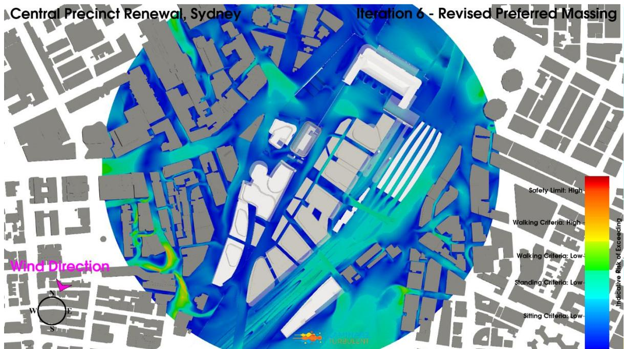
**Figure 121: Iteration 6 – Revised Preferred Massing Configuration, North-northeast Wind Direction, Planview, Pedestrian Level Environmental Wind Risk Contour Plot**
