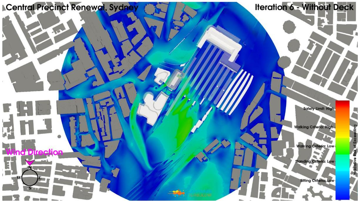
**Figure 108: Iteration 6 – Without Deck Configuration, North Wind Direction, Planview, Pedestrian Level Environmental Wind Risk Contour Plot**
