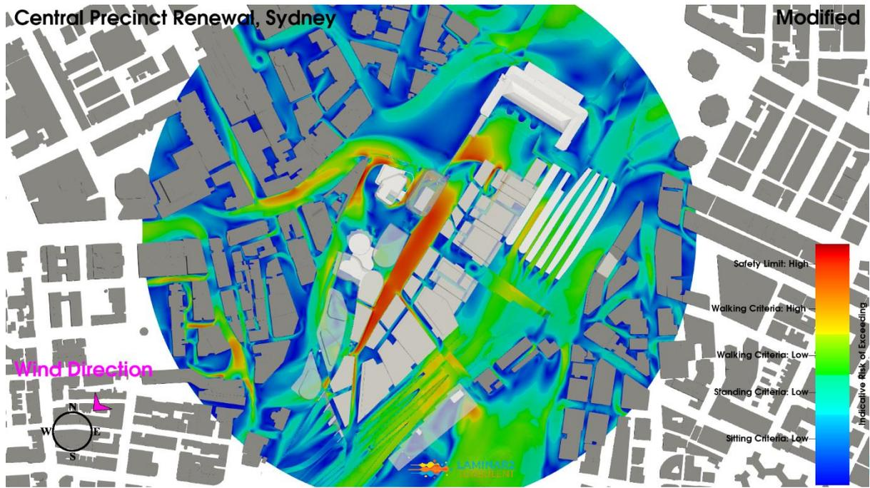
**Figure 24: Iteration 1 Configuration, Northeast Wind Direction, Planview, Ground Level Pedestrian Environmental Wind Risk Contour Plot**
