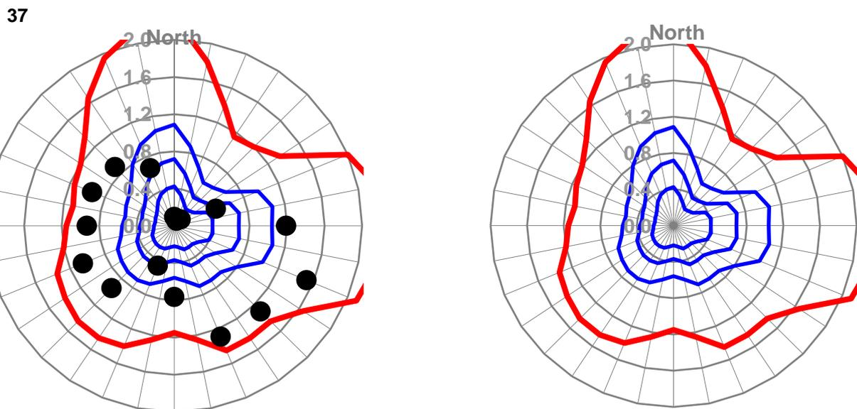
Peak velocity squared ratio  $\left| \frac{\overline{V}_{local}}{\overline{V}_{300m}} \right|^2$  as a function of wind direction
