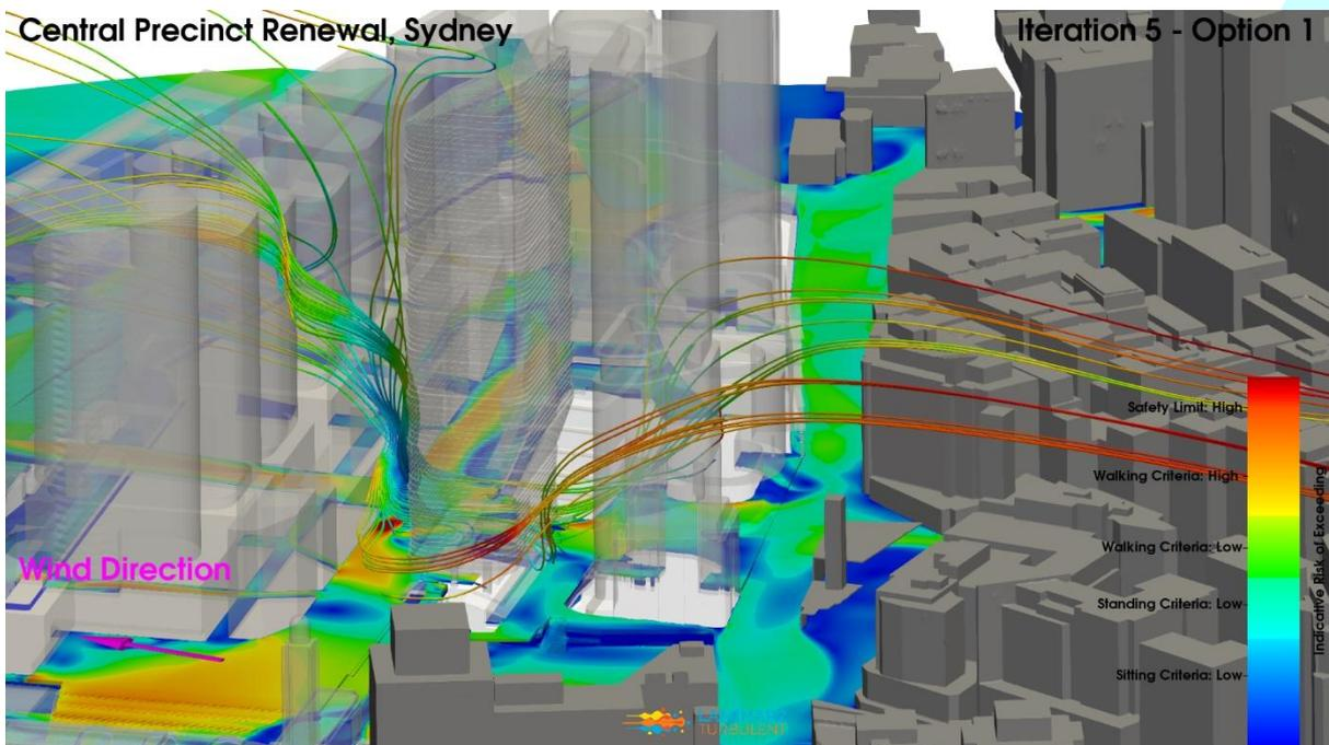
**Figure 87: Iteration 5 – Option 1 Configuration, Northwest Wind Direction, Streamlines & Pedestrian Level Environmental Wind Risk Contour Plot**
