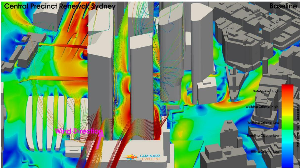
**Figure 14: Baseline Configuration, Northeast Wind Direction, Streamlines, Pedestrian Level Environmental Wind Risk Contour Plot**
