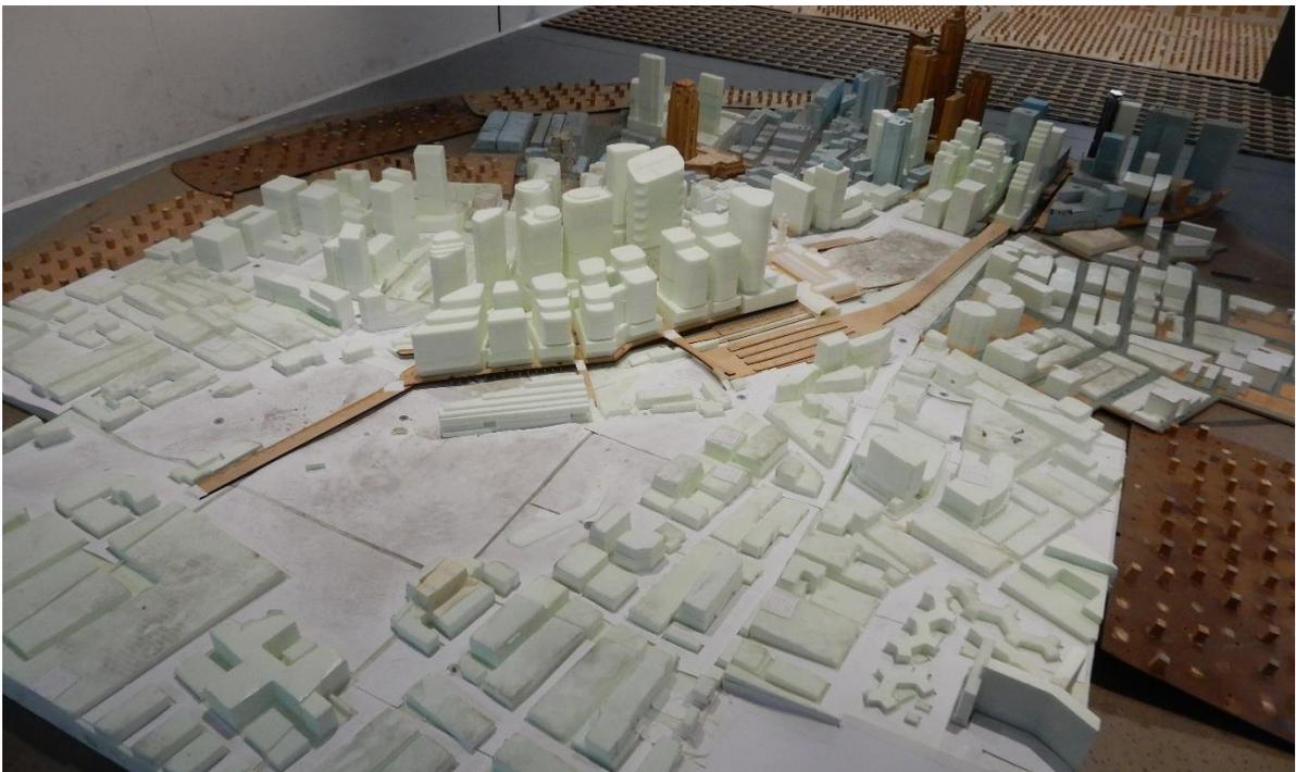
**Figure 3b – View from the southeast of the 1/400 scale model of the Central Precinct Renewal Masterplan – Configuration April 2022 in the wind tunnel.**
