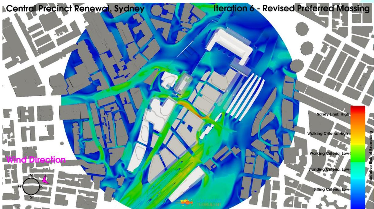
**Figure 123: Iteration 6 - Revised Preferred Massing Configuration, East-northeast Wind Direction, Planview, Pedestrian Level Environmental Wind Risk**
