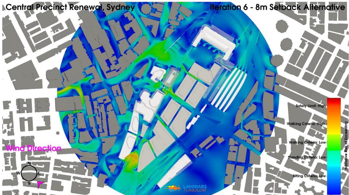
**Figure 159: Iteration 6 – 8m Setback Alternative Configuration, Southeast Wind Direction, Planview, Pedestrian Level Environmental Wind Risk Contour Plot**
