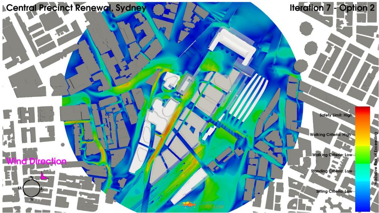
**Figure 184: Iteration 7 Option 2, Northeast Wind Direction, Planview, Pedestrian Level Environmental Wind Risk Contour Plot**
