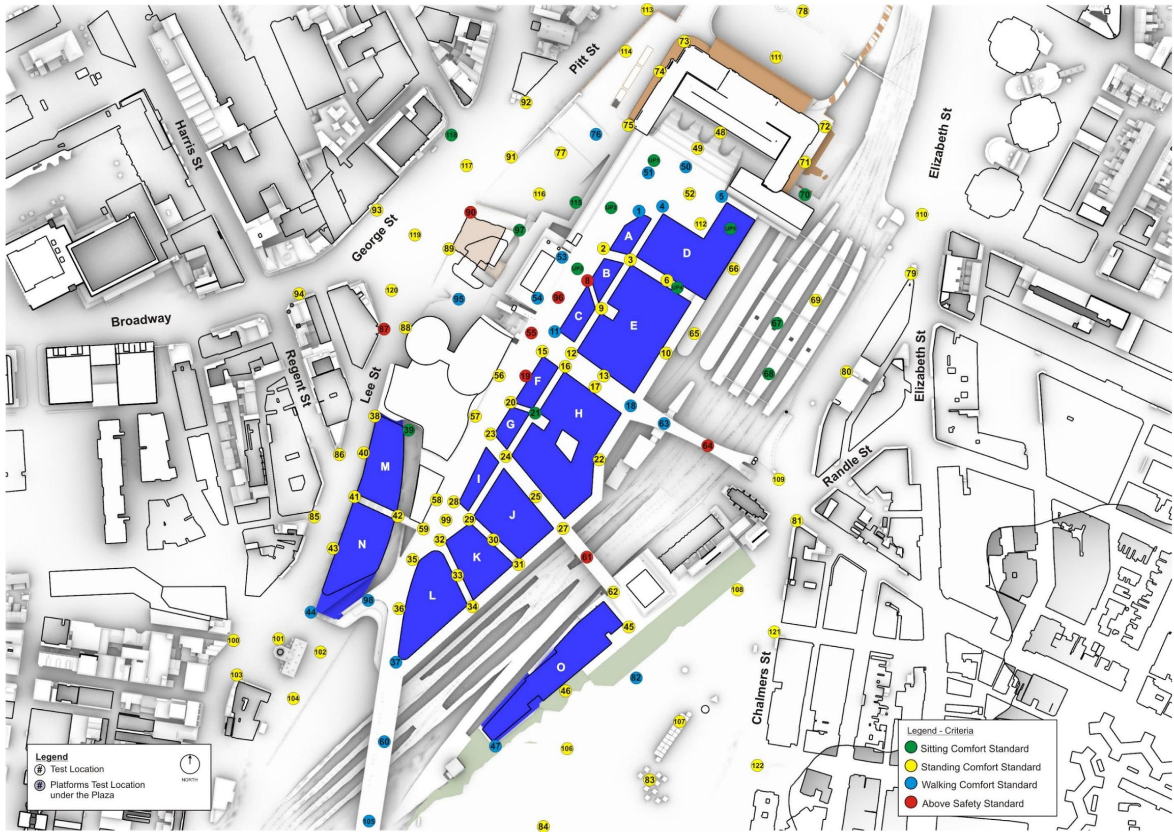
Figure 6b– Summary of wind conditions for Configuration April 2022 for 360° of wind direction
