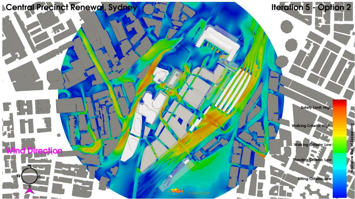
**Figure 92: Iteration 5 - Option 2 Configuration, South Wind Direction, Planview, Pedestrian Level Environmental Wind Risk Contour Plot**
