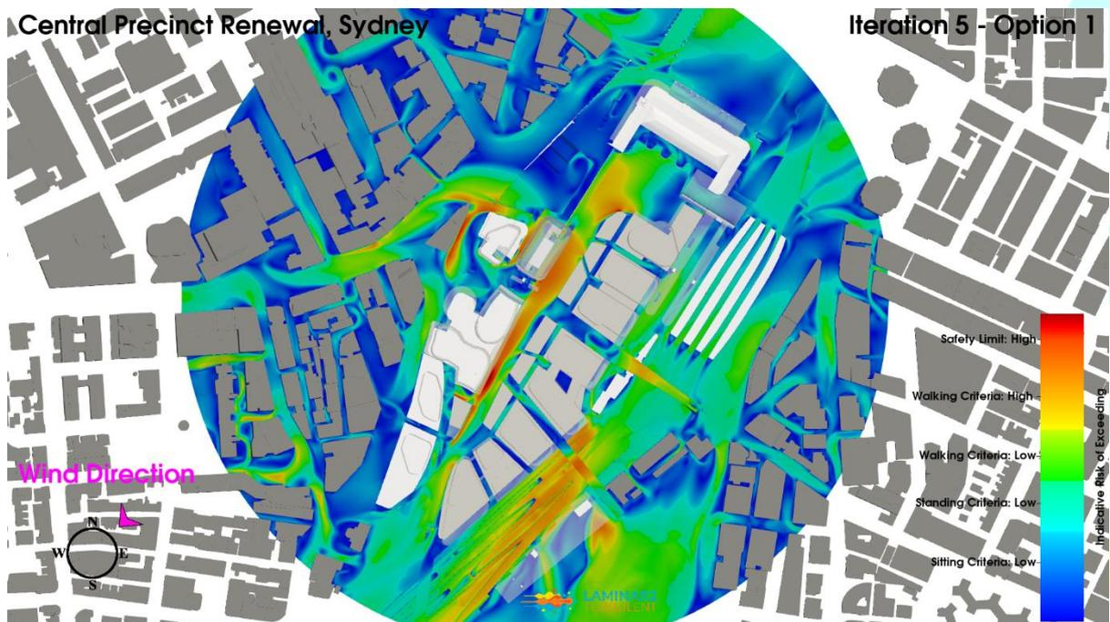
**Figure 83: Iteration 5 – Option 1 Configuration, Northeast Wind Direction, Planview, Pedestrian Level Environmental Wind Risk Contour Plot**
