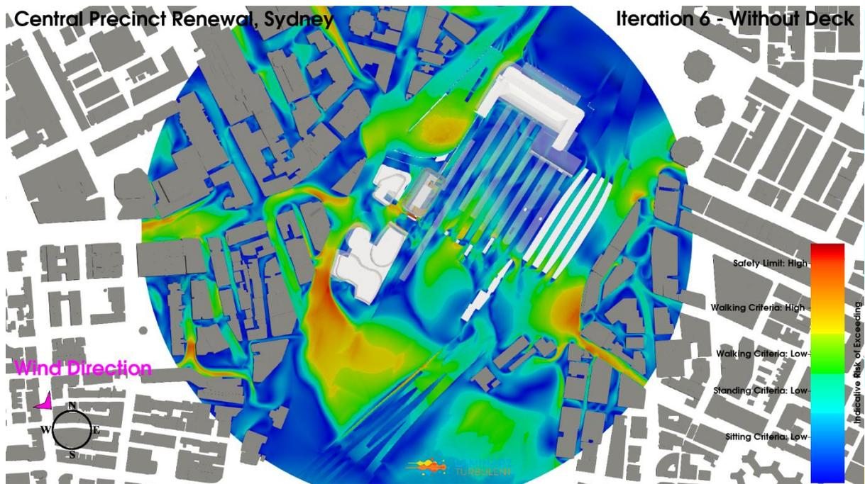
**Figure 115: Iteration 6 – Without Deck Configuration, Northwest Wind Direction, Planview, Pedestrian Level Environmental Wind Risk Contour Plot**
