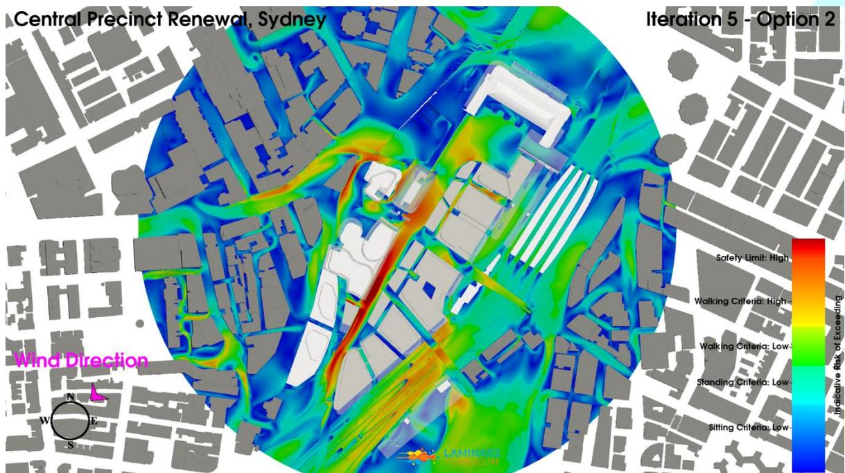
**Figure 91: Iteration 5 – Option 2 Configuration, Northeast Wind Direction, Planview, Pedestrian Level Environmental Wind Risk Contour Plot**
