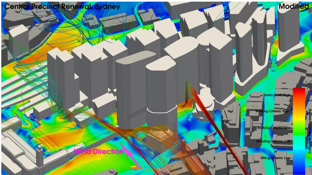
**Figure 34: Iteration 1 Configuration, Northwest Wind Direction, Streamlines, Pedestrian Level Environmental Wind Risk Contour Plot**
