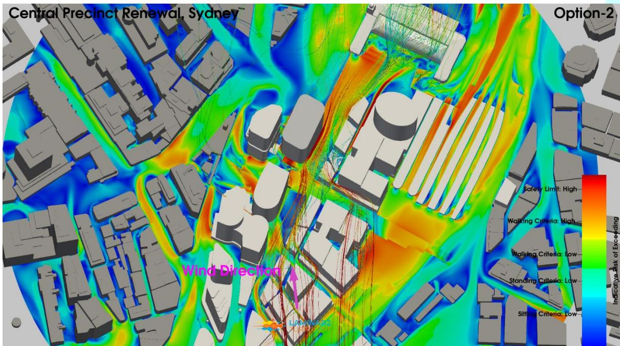
**Figure 51: Iteration 2 – Option 2 Configuration, South Wind Direction, Streamlines, Pedestrian Level Environmental Wind Risk Contour Plot**
