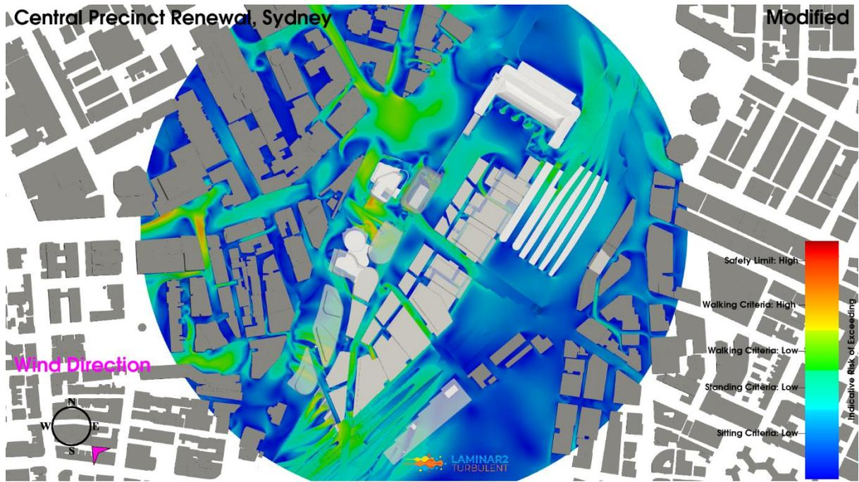
**Figure 26: Iteration 1 Configuration, Southeast Wind Direction, Planview, Ground Level Pedestrian Environmental Wind Risk Contour Plot**
