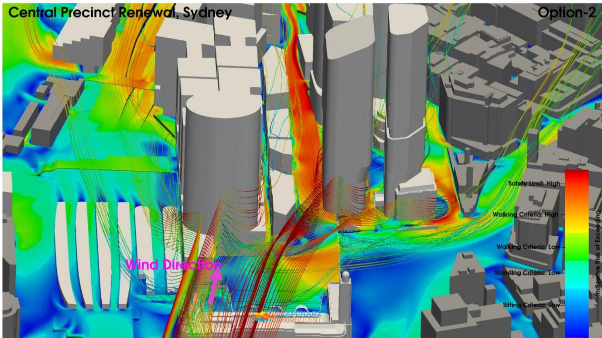
**Figure 50: Iteration 2 – Option 2 Configuration, Northeast Wind Direction, Streamlines, Pedestrian Level Environmental Wind Risk Contour Plot**
