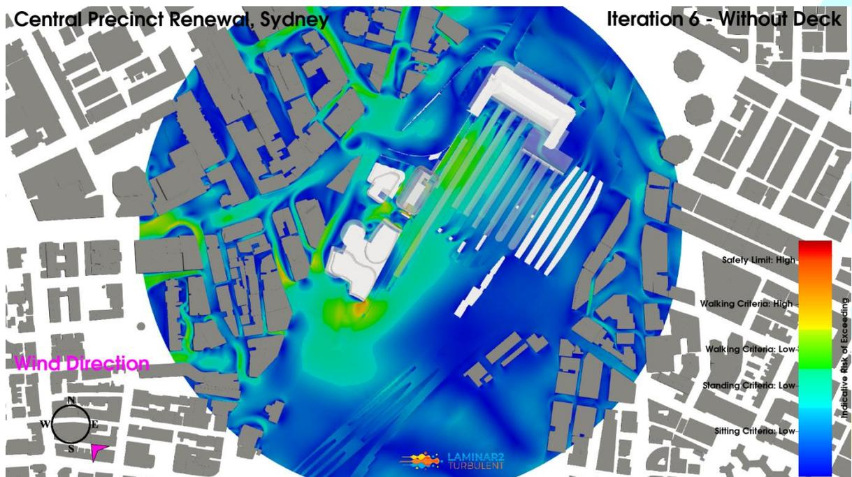
**Figure 111: Iteration 6 – Without Deck Configuration, Southeast Wind Direction, Planview, Pedestrian Level Environmental Wind Risk Contour Plot**
