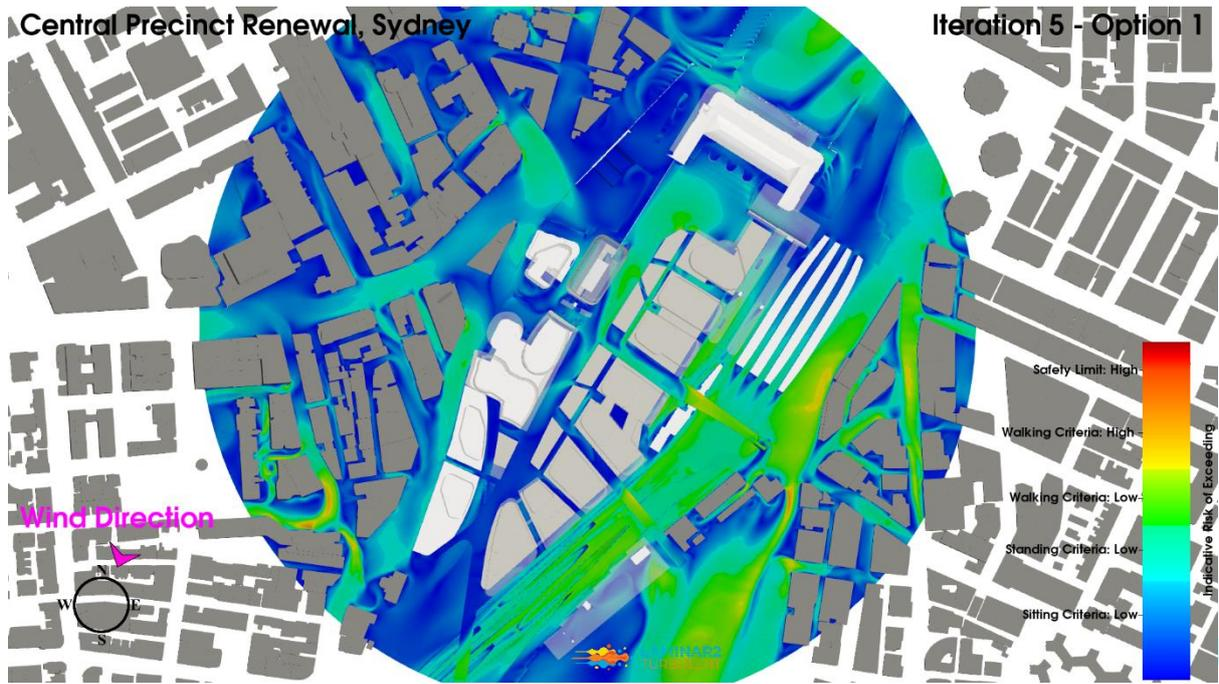
**Figure 82: Iteration 5 – Option 1 Configuration, North-northeast Wind Direction, Planview, Pedestrian Level Environmental Wind Risk Contour Plot**
