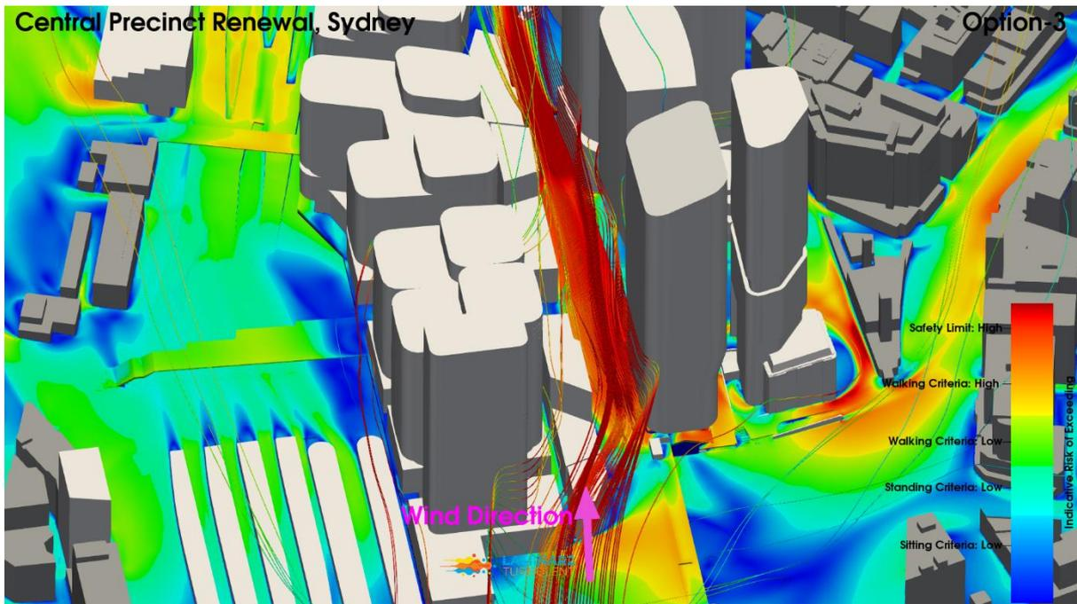
**Figure 61: Iteration 3 – Option 3 Configuration, Northeast Wind Direction (zoom view), Streamlines, Pedestrian Level Environmental Wind Risk Contour Plot**
