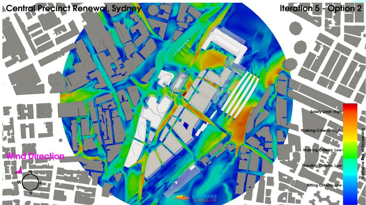
**Figure 93: Iteration 5 - Option 2 Configuration, Northwest Wind Direction, Planview, Pedestrian Level Environmental Wind Risk Contour Plot**
