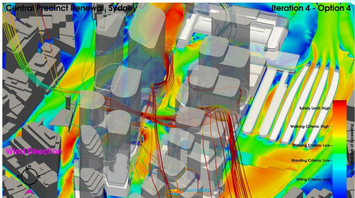
**Figure 70: Iteration 4 - Option 4 Configuration, South Wind Direction, Streamlines & Pedestrian Level Environmental Wind Risk Contour Plot**
