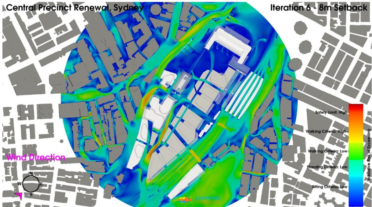
**Figure 148: Iteration 6 – 8m Setback Configuration, Southwest Wind Direction, Planview, Pedestrian Level Environmental Wind Risk Contour Plot**
