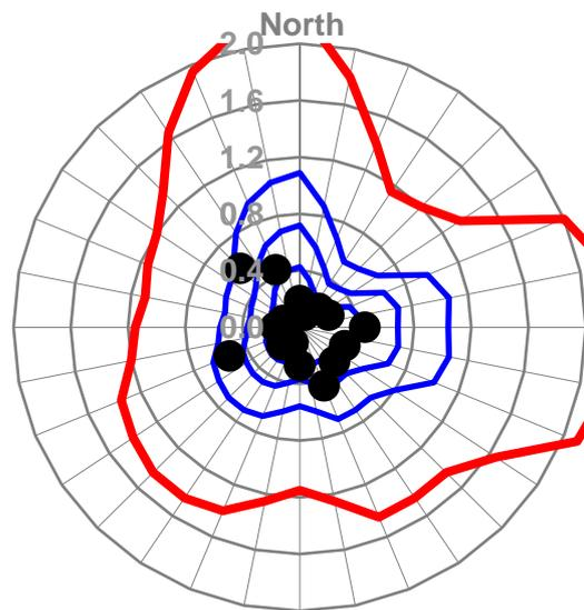
Peak velocity squared ratio  $\left| \frac{\hat{V}_{local}}{V_{300m}} \right|^2$  as a function of wind direction
