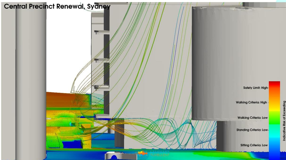
**Figure 139: Iteration 6 – Revised Preferred Massing Configuration, Northwest Wind Direction, Streamlines & Pedestrian Level Environmental Wind Risk Contour Plot**
