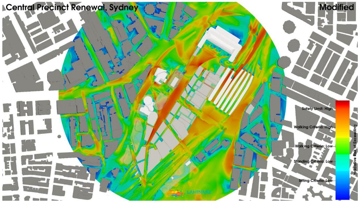
**Figure 22: Iteration 1 Configuration, Combined Wind Directions, Planview, Ground Level Maximum Pedestrian Environmental Wind Risk Contour Plot**
