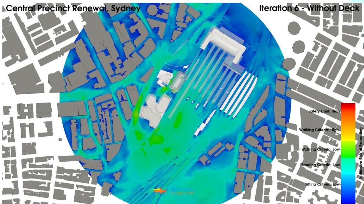
**Figure 117: Iteration 6 – Baseline Without Deck Configuration, Combined Wind Directions, Planview, Average Pedestrian Level Environmental Wind Risk**
