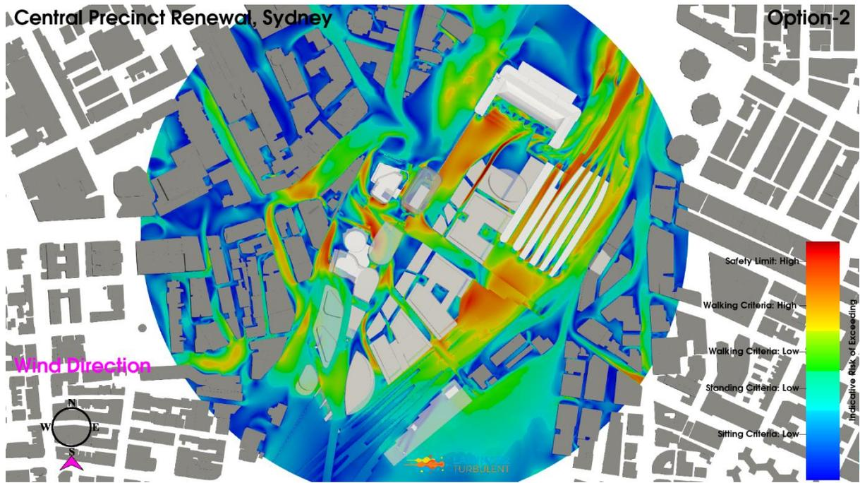
**Figure 48: Iteration 2 – Option 2 Configuration, South Wind Direction, Planview, Ground Level Pedestrian Environmental Wind Risk Contour Plot**
