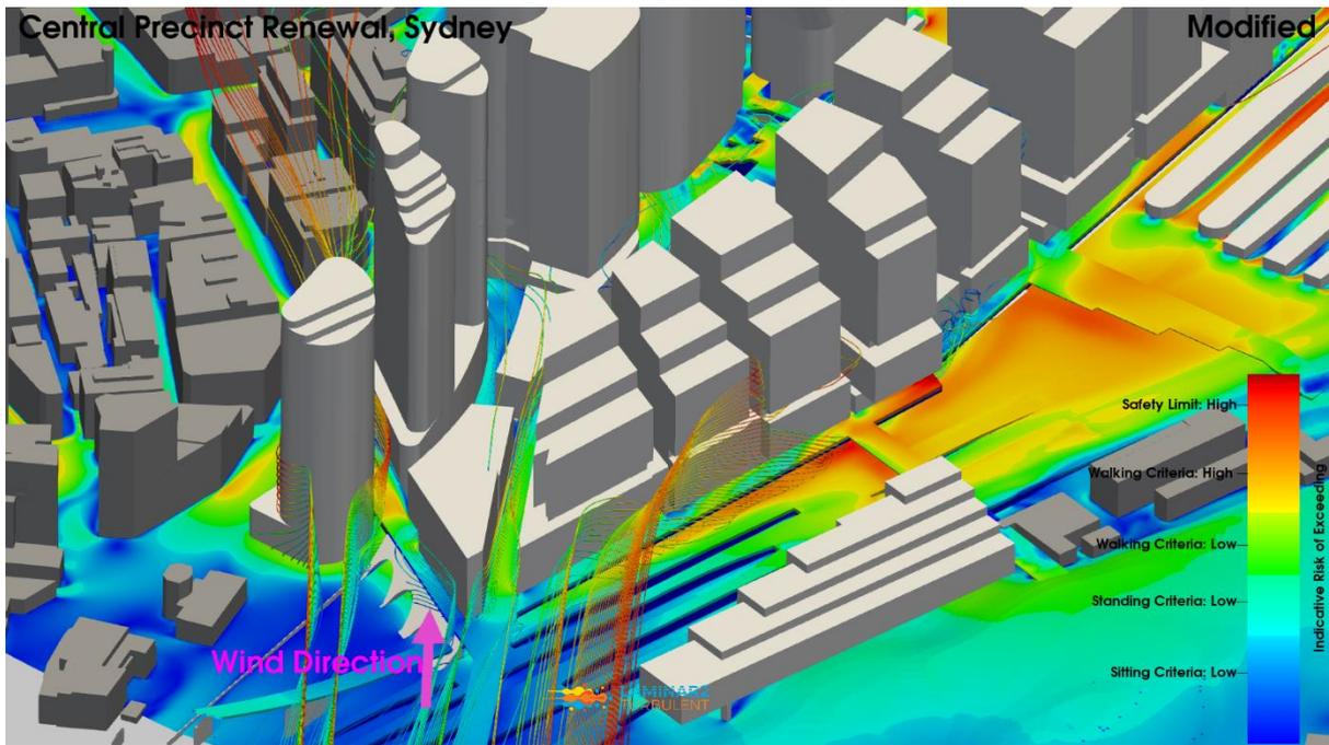
**Figure 32: Iteration 1 Configuration, South Wind Direction, Streamlines, Pedestrian Level Environmental Wind Risk Contour Plot**
