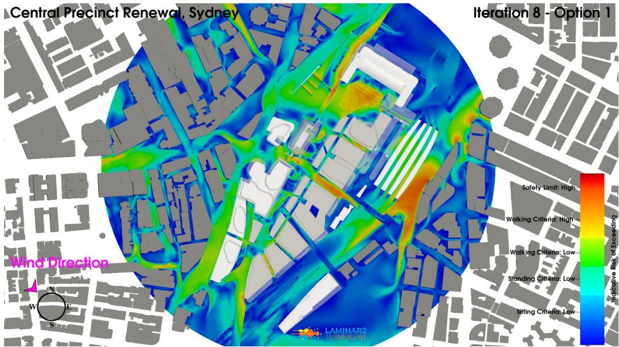
**Figure 188: Iteration 8 Option 1, Northwest Wind Direction, Planview, Pedestrian Level Environmental Wind Risk Contour Plot**
