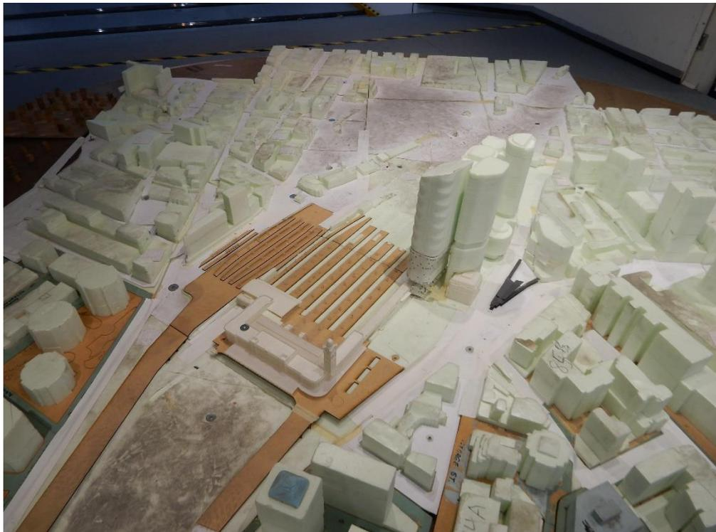
**Figure 4b – View from the north of the 1/400 scale model of the Central Precinct Renewal Masterplan – Existing Configuration in the wind tunnel.**
