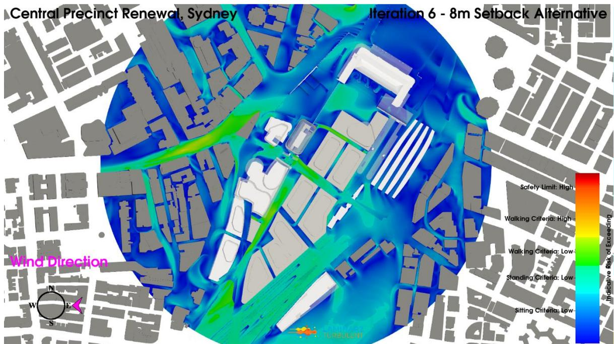
**Figure 158: Iteration 6 - 8m Setback Alternative Configuration, East Wind Direction, Planview, Pedestrian Level Environmental Wind Risk Contour Plot**
