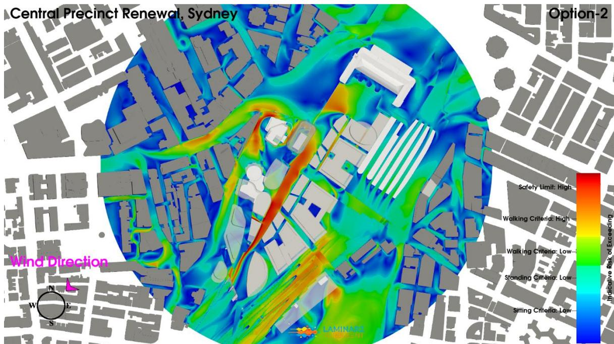
**Figure 47: Iteration 2 – Option 2 Configuration, Northeast Wind Direction, Planview, Ground Level Pedestrian Environmental Wind Risk Contour Plot**
