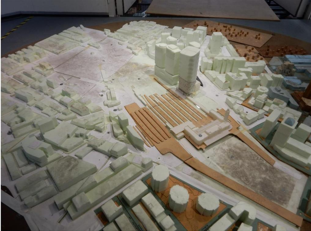
**Figure 4a – View from the northeast of the 1/400 scale model of the Central Precinct Renewal Masterplan – Existing Configuration in the wind tunnel.**
