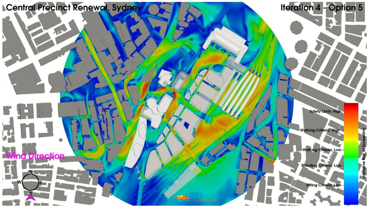
**Figure 76: Iteration 4 - Option 5 Configuration, South Wind Direction, Planview, Pedestrian Level Environmental Wind Risk Contour Plot**
