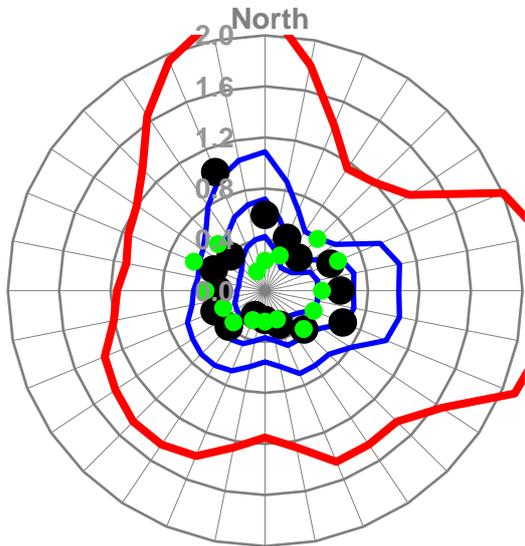
Peak velocity squared ratio  $\left| \frac{\widehat{V}_{\text{local}}}{\widehat{V}_{300\text{m}}} \right|^2$  as a function of wind direction
