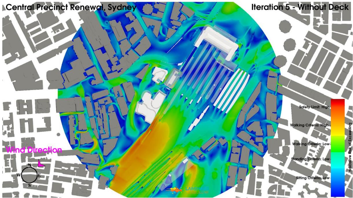
**Figure 101: Iteration 5 – Baseline Without Deck Configuration, Northeast Wind Direction, Planview, Pedestrian Level Environmental Wind Risk Contour Plot**
