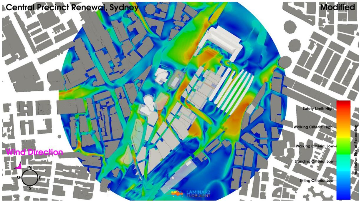
**Figure 30: Iteration 1 Configuration, Northwest Wind Direction, Planview, Ground Level Pedestrian Environmental Wind Risk Contour Plot**
