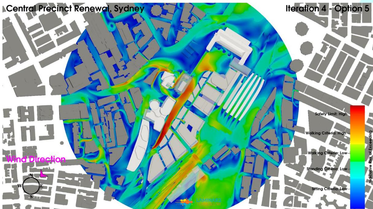
**Figure 75: Iteration 4 – Option 5 Configuration, Northeast Wind Direction, Planview, Pedestrian Level Environmental Wind Risk Contour Plot**
