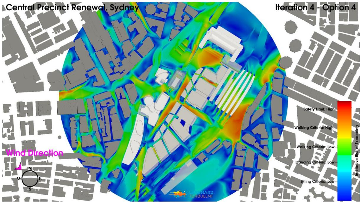
**Figure 69: Iteration 4 - Option 4 Configuration, Northwest Wind Direction, Planview, Pedestrian Level Environmental Wind Risk Contour Plot**
