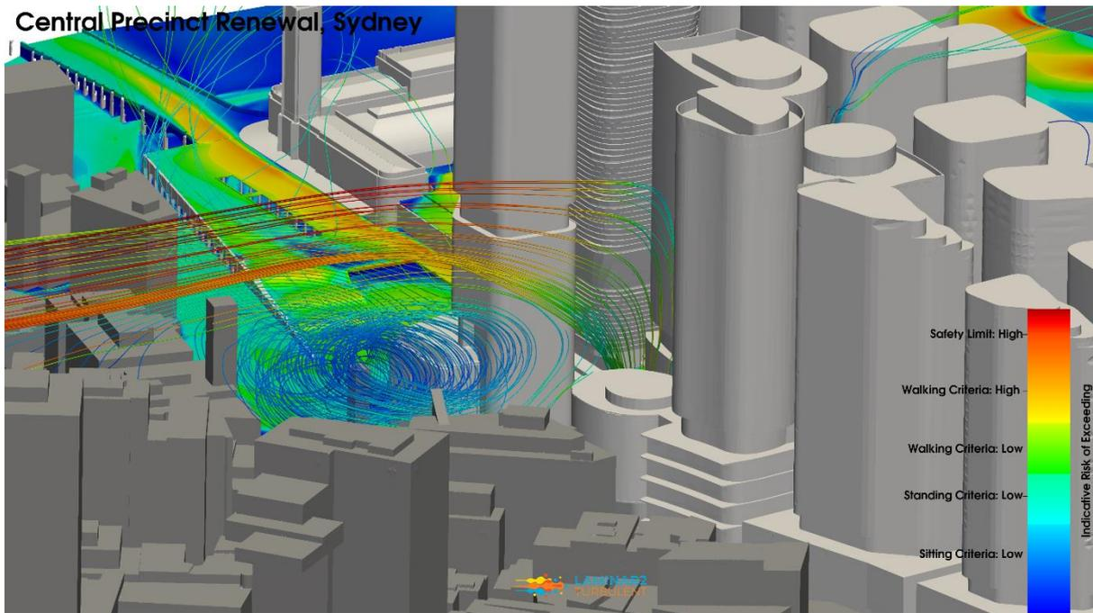
**Figure 136: Iteration 6 – Revised Preferred Massing Configuration, Northwest Wind Direction, Streamlines & Pedestrian Level Environmental Wind Risk Contour Plot**
