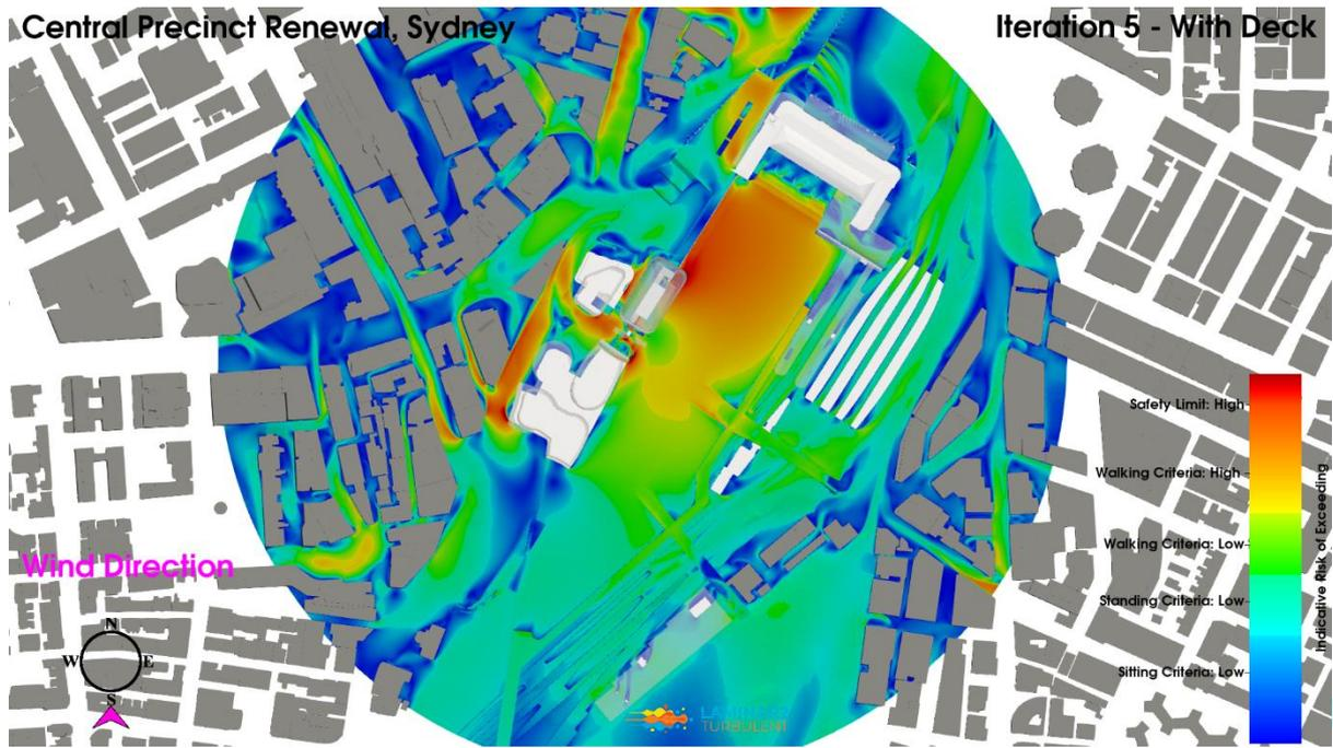
**Figure 97: Iteration 5 – Baseline With Deck Configuration, South Wind Direction, Planview, Pedestrian Level Environmental Wind Risk Contour Plot**
