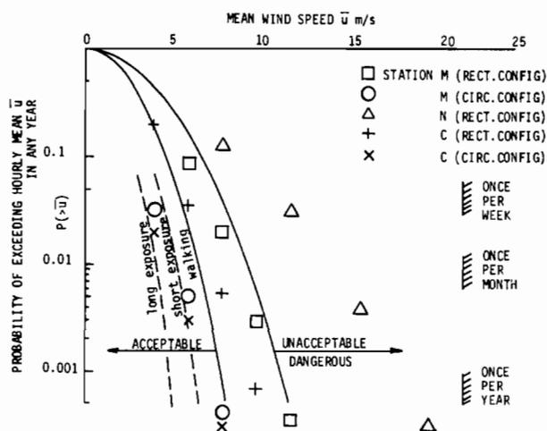
Fig.5. Probability distributions of mean wind speeds at several stations compared with Melbourne's criteria for environmental wind conditions (Daylight hours,  $\sigma_u = 0.3\bar{u}$ ,  $\hat{u} = 2\bar{u}$ ).
