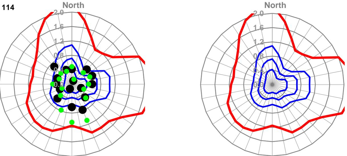
Peak velocity squared ratio  $\left| \frac{\bar{V}_{local}}{\bar{V}_{300m}} \right|^2$  as a function of wind direction
