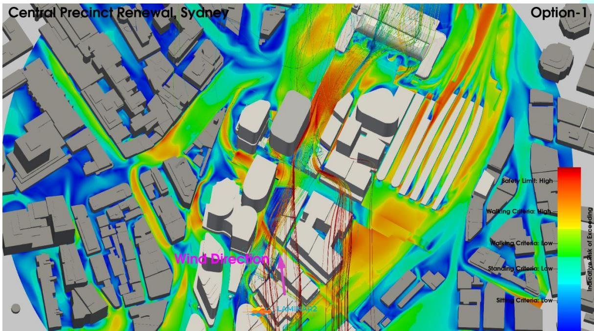
**Figure 42: Iteration 2 – Option 1 Configuration, South Wind Direction, Streamlines, Pedestrian Level Environmental Wind Risk Contour Plot**
