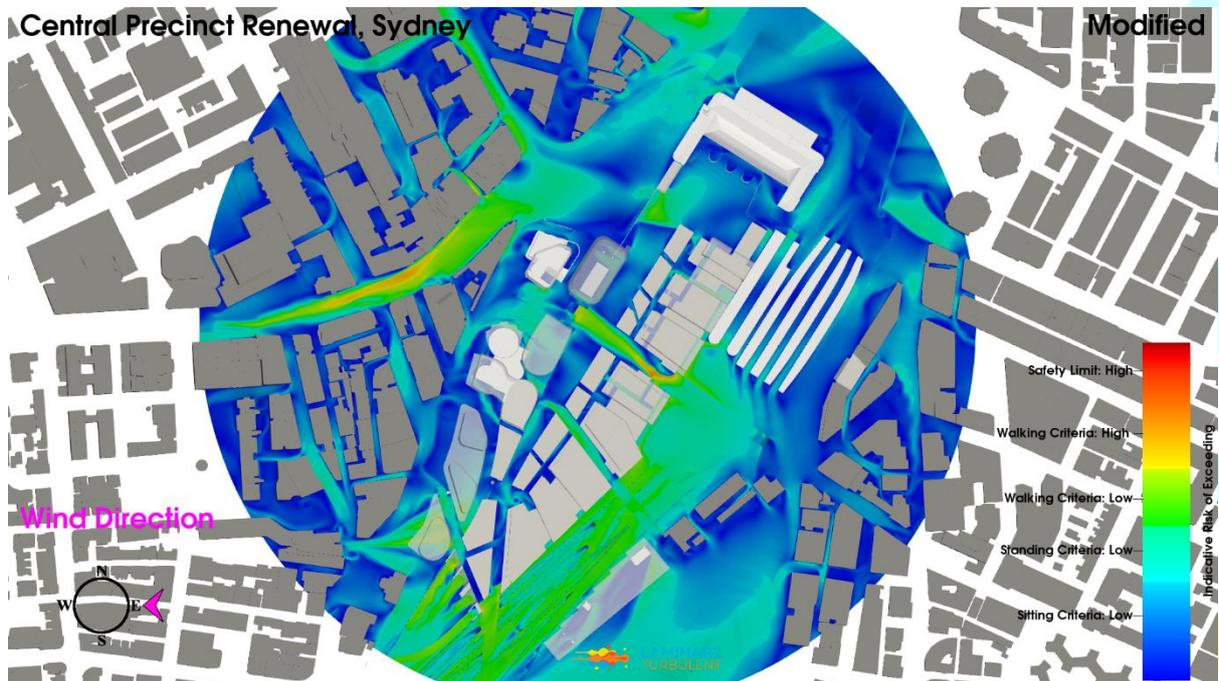
**Figure 25: Iteration 1 Configuration, East Wind Direction, Planview, Ground Level Pedestrian Environmental Wind Risk Contour Plot**
