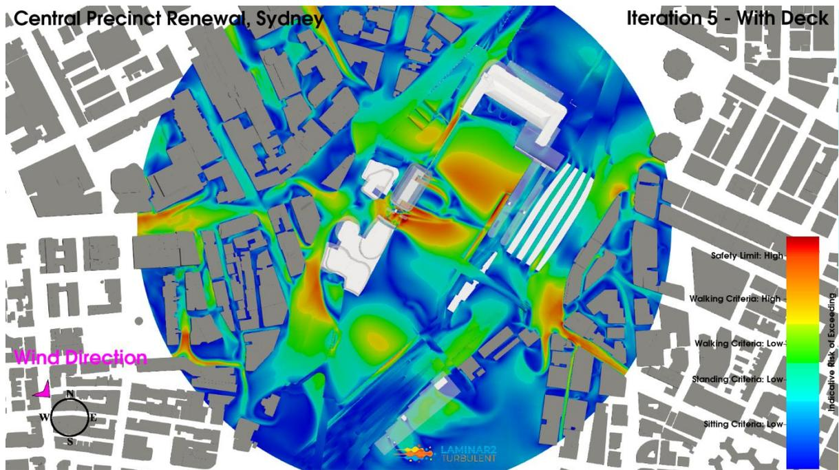
**Figure 98: Iteration 5 – Baseline With Deck Configuration, Northwest Wind Direction, Planview, Pedestrian Level Environmental Wind Risk Contour Plot**
