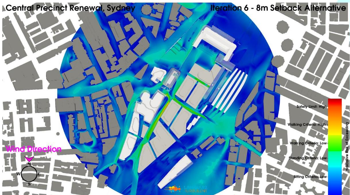
**Figure 156: Iteration 6 – 8m Setback Alternative Configuration, North Wind Direction, Planview, Pedestrian Level Environmental Wind Risk Contour Plot**
