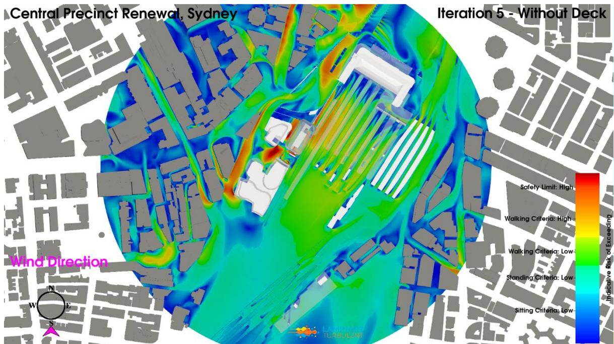
**Figure 102: Iteration 5 – Baseline Without Deck Configuration, South Wind Direction, Planview, Pedestrian Level Environmental Wind Risk Contour Plot**
