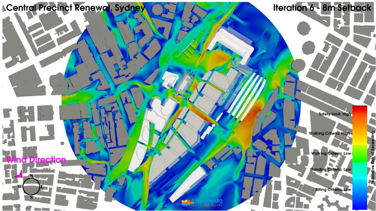
**Figure 150: Iteration 6 – 8m Setback Configuration, Northwest Wind Direction, Planview, Pedestrian Level Environmental Wind Risk Contour Plot**
