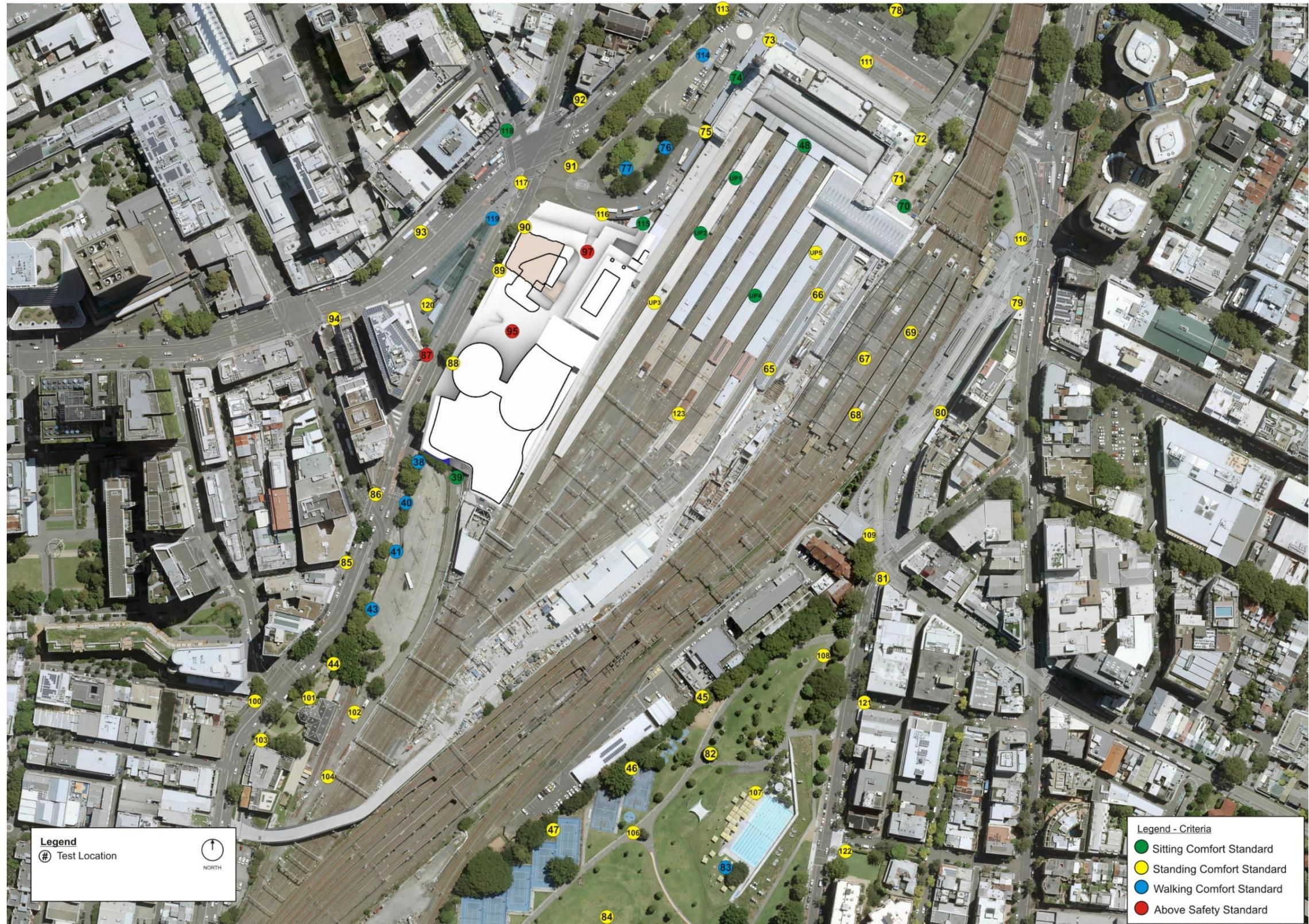
Figure 6a – Summary of wind conditions for Existing Configuration for 360° of wind direction
