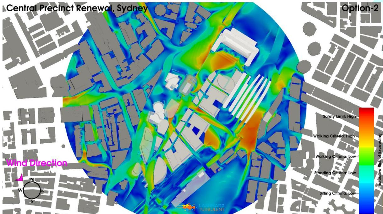
**Figure 49: Iteration 2 – Option 2 Configuration, Northwest Wind Direction, Planview, Ground Level Pedestrian Environmental Wind Risk Contour Plot**
