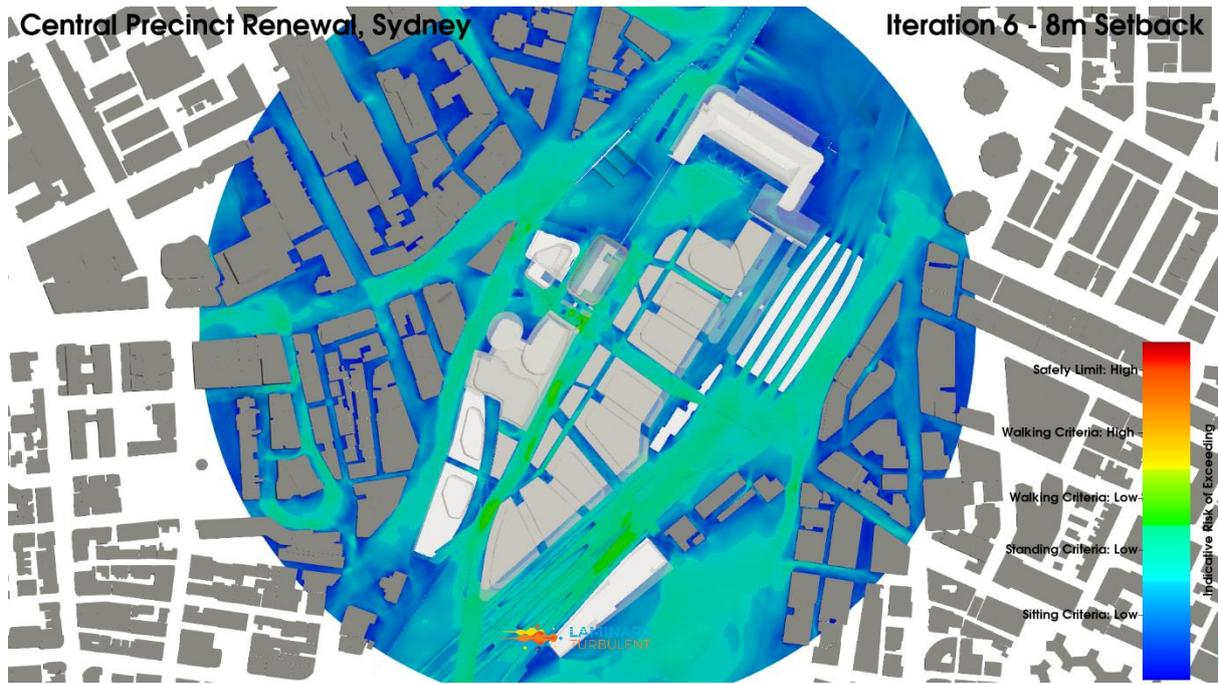
**Figure 152: Iteration 6 – 8m Setback Configuration, Combined Wind Directions, Planview, Average Pedestrian Level Environmental Wind Risk Contour Plot**
