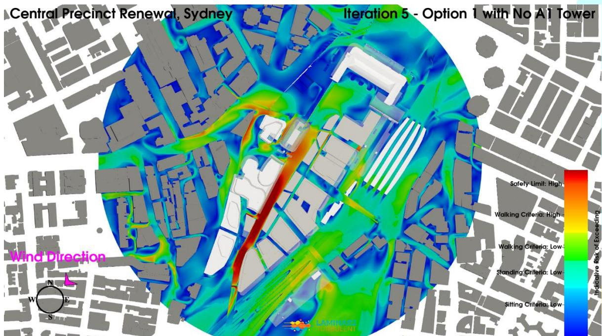
**Figure 105: Iteration 5 - Option 1 With No A1 Tower Configuration, Northeast Wind Direction, Planview, Pedestrian Level Environmental Wind Risk Contour Plot**
