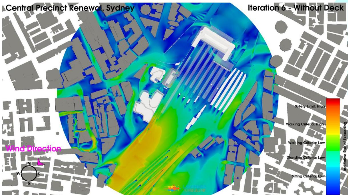
**Figure 109: Iteration 6 – Without Deck Configuration, Northeast Wind Direction, Planview, Pedestrian Level Environmental Wind Risk Contour Plot**
