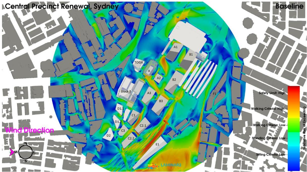
**Figure 12: Baseline Configuration, West Wind Direction, Planview, Ground Level Pedestrian Environmental Wind Risk Contour Plot**
