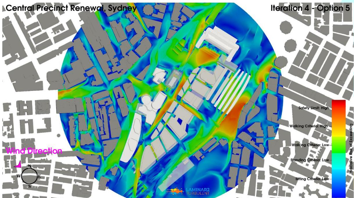
**Figure 77: Iteration 4 - Option 5 Configuration, Northwest Wind Direction, Planview, Pedestrian Level Environmental Wind Risk Contour Plot**
