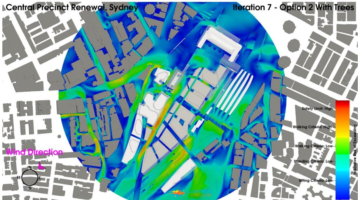
**Figure 186: Iteration 7 Option 2 With Trees, Northeast Wind Direction, Planview, Pedestrian Level Environmental Wind Risk Contour Plot**
