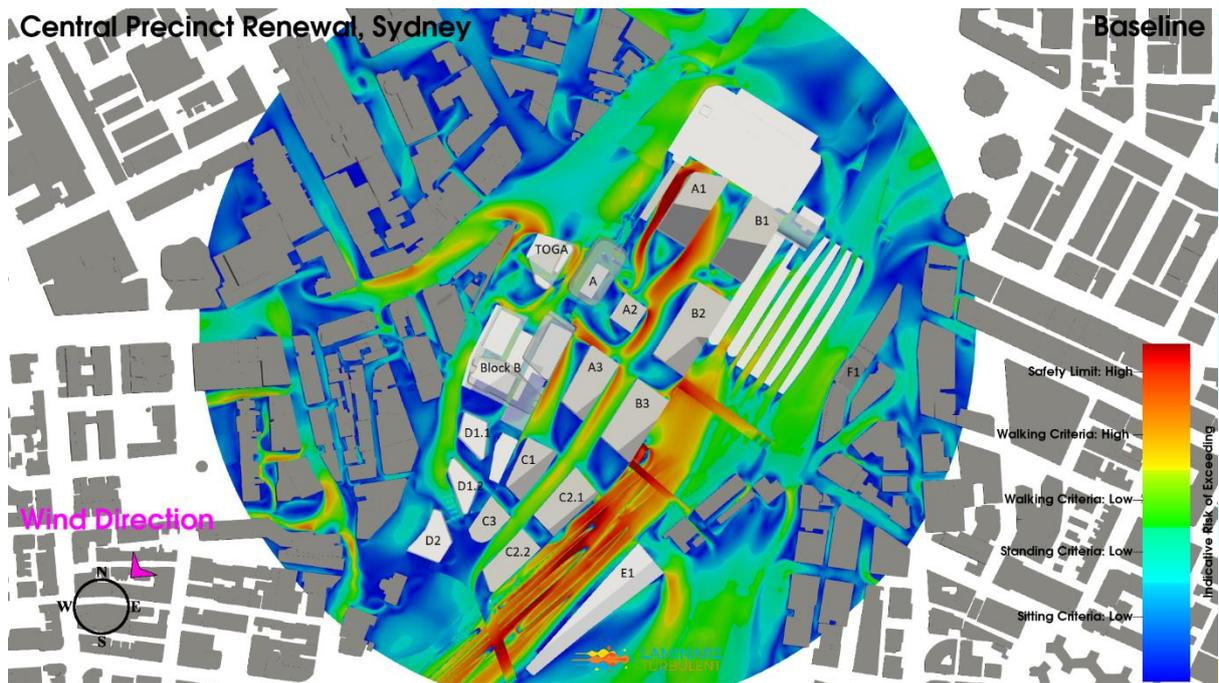
**Figure 7: Baseline Configuration, Northeast Wind Direction, Planview, Ground Level Pedestrian Environmental Wind Risk Contour Plot**
