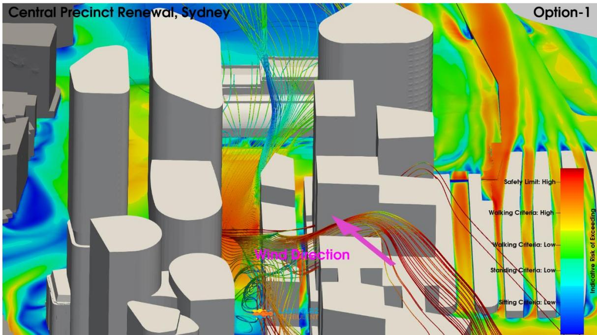
**Figure 43: Iteration 2 – Option 1 Configuration, South Wind Direction (zoom view), Streamlines, Pedestrian Level Environmental Wind Risk Contour Plot**
