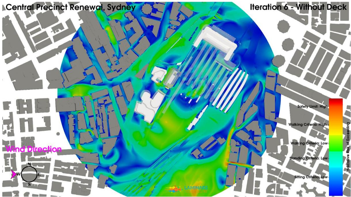
**Figure 114: Iteration 6 – Without Deck Configuration, West Wind Direction, Planview, Pedestrian Level Environmental Wind Risk Contour Plot**
