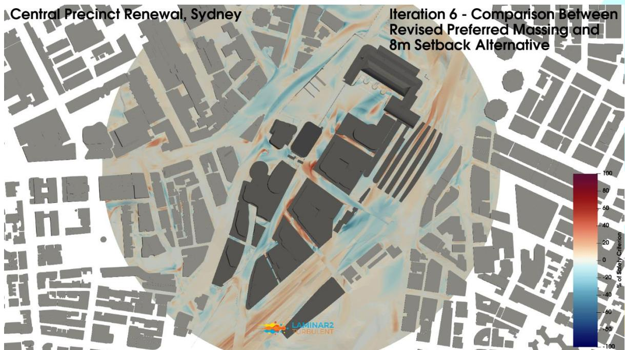
**Figure 168: Comparison of Maximum Pedestrian Level Environmental Wind Risk between Iteration 6 - Baseline Without Deck and Iteration 6 - 8m Setback Alternative, Planview.**
