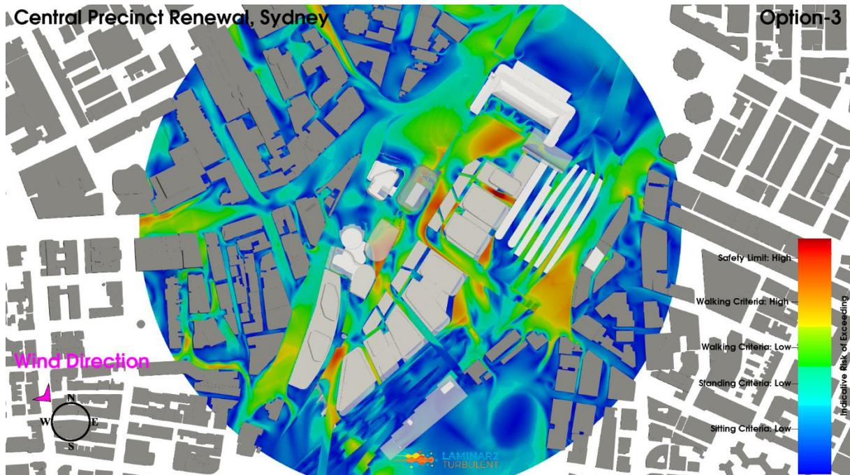
**Figure 59: Iteration 3 – Option 3 Configuration, Northwest Wind Direction, Planview, Ground Level Pedestrian Environmental Wind Risk Contour Plot**
