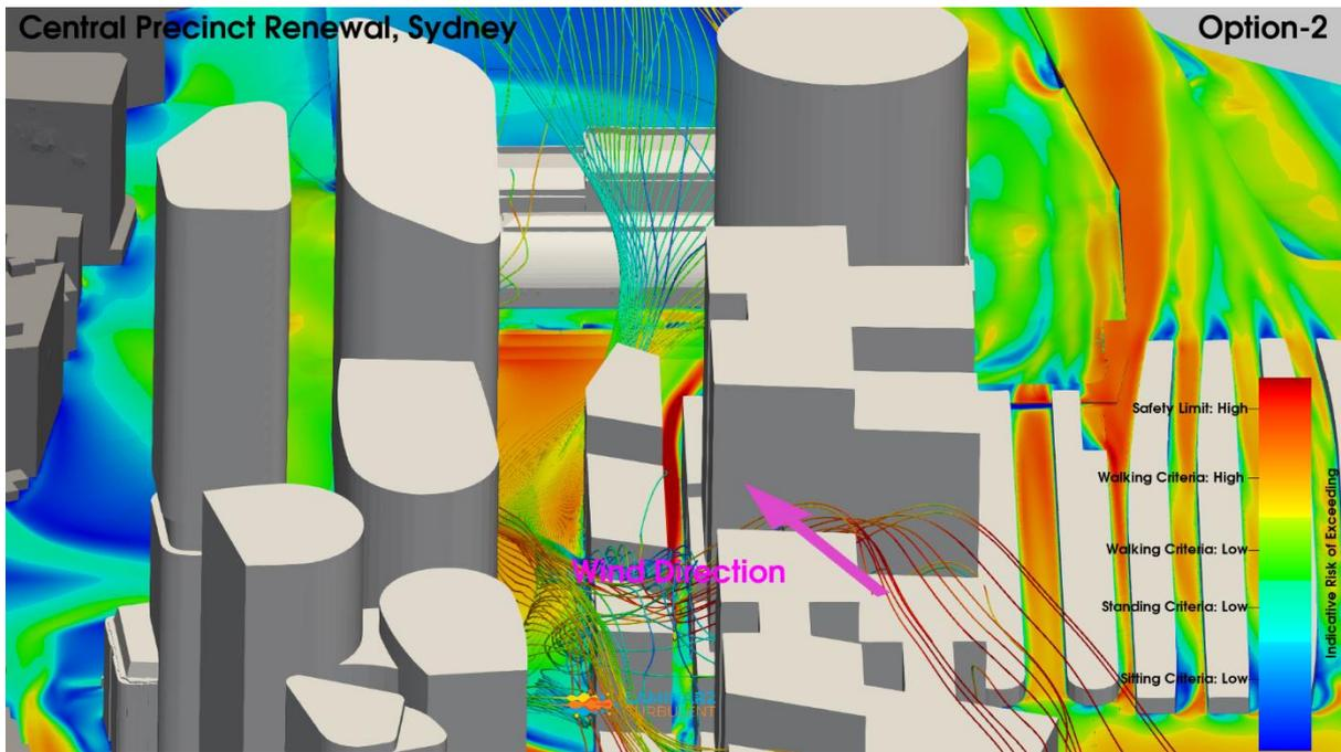
**Figure 52: Iteration 2 – Option 2 Configuration, South Wind Direction (zoom view), Streamlines, Pedestrian Level Environmental Wind Risk Contour Plot**
