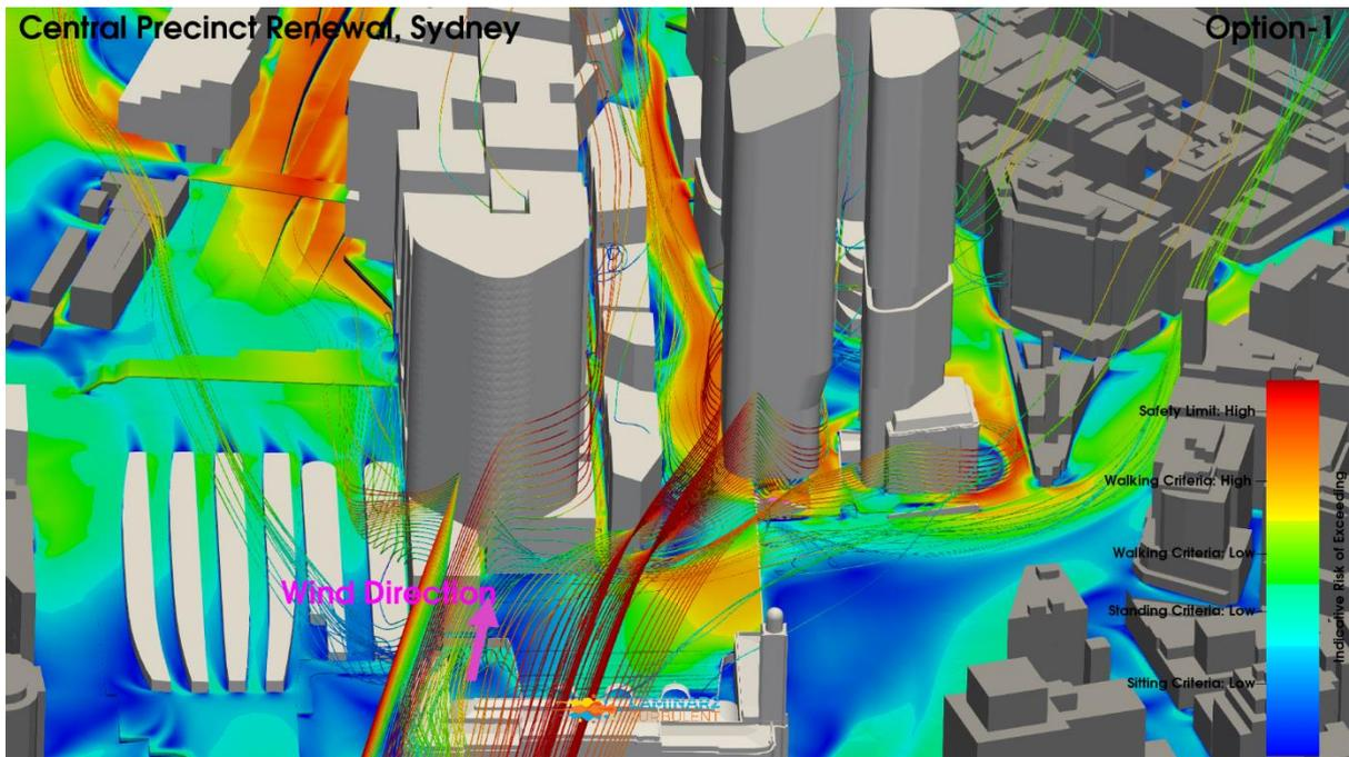
**Figure 41: Iteration 2 – Option 1 Configuration, Northeast Wind Direction, Streamlines, Pedestrian Level Environmental Wind Risk Contour Plot**
