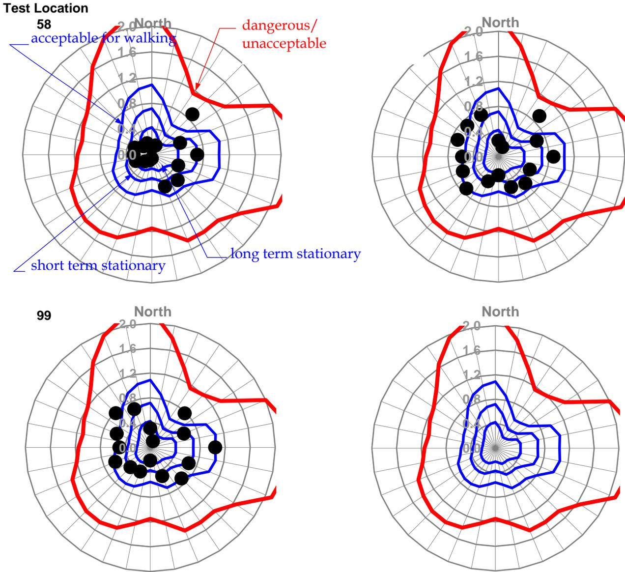
Peak velocity squared ratio  $\left| \frac{\hat{V}_{local}}{\hat{V}_{300m}} \right|^2$  as a function of wind direction
