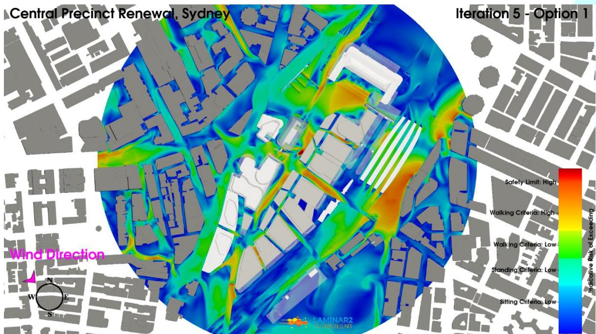
**Figure 85: Iteration 5 - Option 1 Configuration, Northwest Wind Direction, Planview, Pedestrian Level Environmental Wind Risk Contour Plot**
