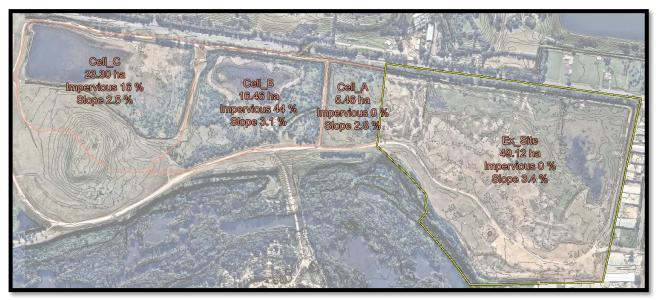
Plate 2 – Existing Conditions Catchment Plan
