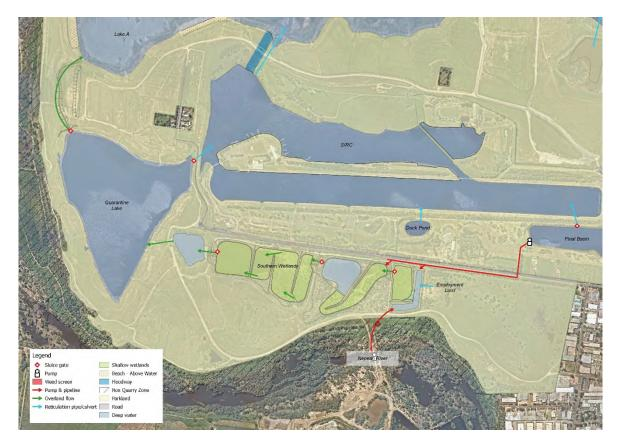
Figure 10: Revised design of water supply and treatment system in the South.
