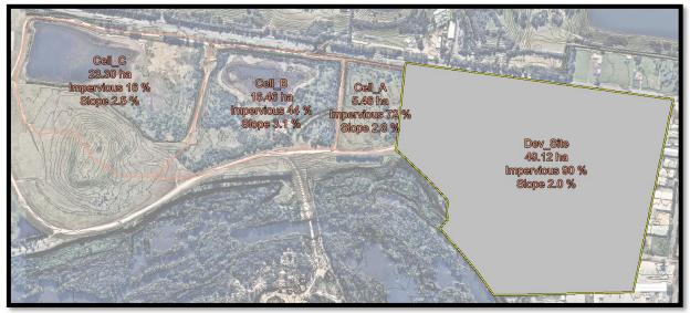
Plate 4 – Developed Conditions Catchment Plan
