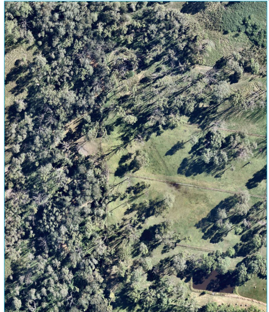
Figure 3-17 Aerial image of site 41. Overland flow path is evident in centre of image
