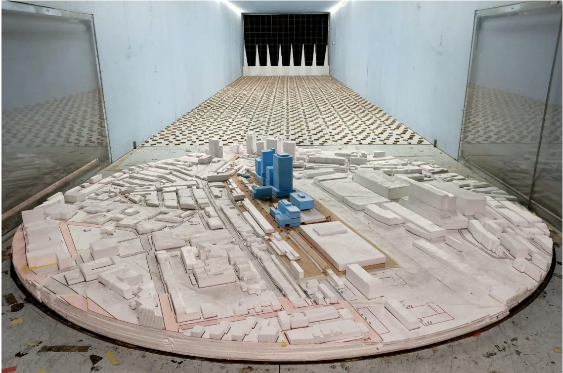
Figure 4e: Photograph of the Wind Tunnel Model (Case 1) - view from the west
