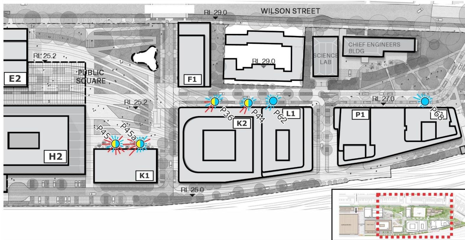
Figure 17a: Wind Tunnel Results: With Paint Shop Sub-Precinct Massing (Treatment Scenario 01)
