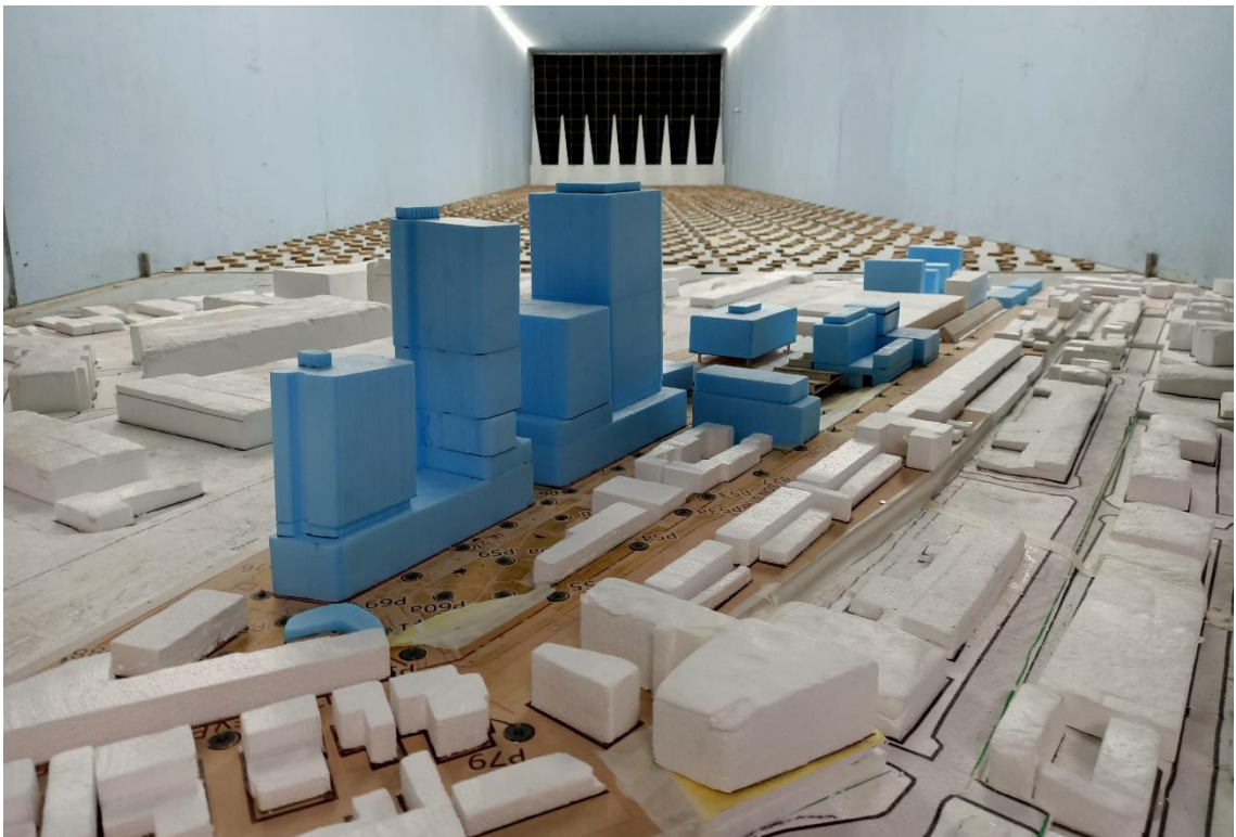
Figure 5a: Photograph of the Wind Tunnel Model with Clothing Store Sub-Precinct (Case 2) - view from north-east
