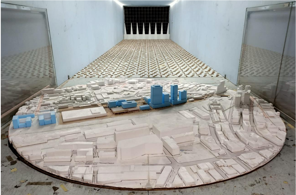
Figure 5d: Photograph of the Wind Tunnel Model with Clothing Store Sub-Precinct (Case 2) - view from the south
