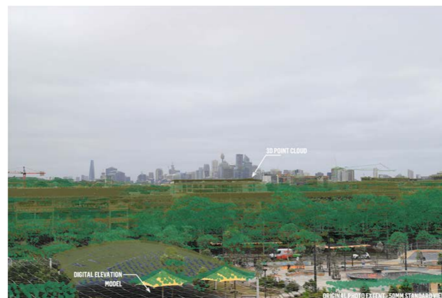
Figure 25 View 02 - Existing conditions with 3D point cloud for accurate alignment of model overlay on photograph
