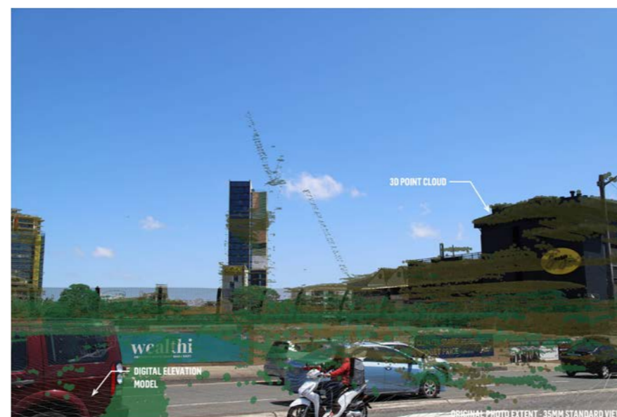
Figure 22 View 01 - Existing conditions with 3D point cloud for accurate alignment of model overlay on photograph
