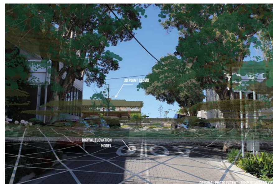
Figure 31 View 04 - Existing conditions with 3D point cloud for accurate alignment of model overlay on photograph
