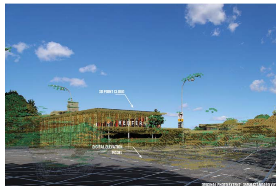
Figure 28 View 03 - Existing conditions with 3D point cloud for accurate alignment of model overlay on photograph
