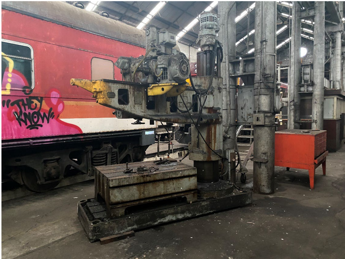
Figure 4.68: Drilling machine produced by William Asquith Ltd of Halifax, England, likely fabricated in the 1920s. The item is not listed as part of the ATP or Railcorp S170 Registers. (Source: Curio Projects, 2022)
